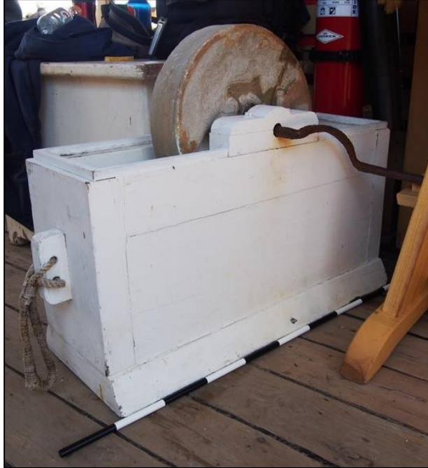
Figure 47. A well-worn grindstone set inside of a wooden frame onboard the whaleship Charles W. Morgan in July 2015 (image courtesy of Mystic Seaport).
