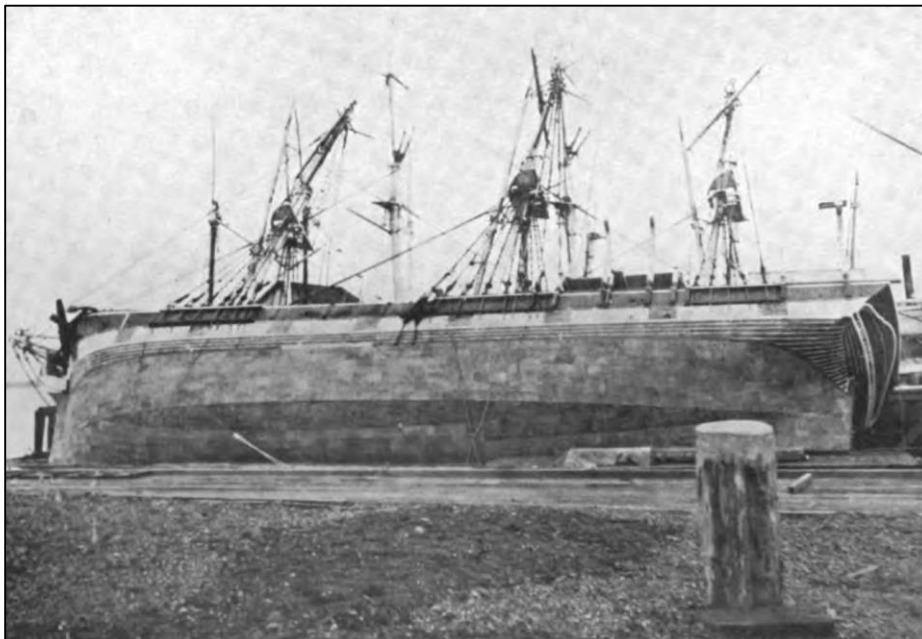
Figure 27. Whaleship James Arnold careened onto its starboard side while being refit. From Maury, N.B. 1896.
