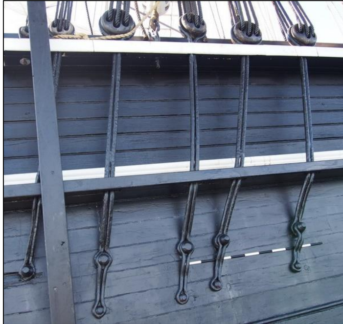
Figure 35. Chainplates attached to the mid-ship portion of the hull of the whaleship Charles W. Morgan and used to stay the mainmast (image courtesy of Mystic Seaport).
