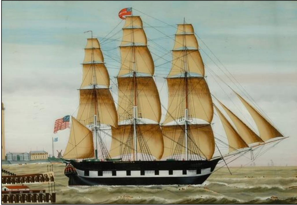
Figure 37. Painting of the whaleship Konohasset showing the false gun port paint scheme. From: http://www.skinnerinc.com/auctions/2431/lots/275 .
