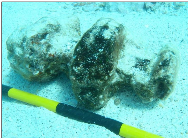
Figure 69. Remains of an ‘upper block’ of a cutting tackle recorded at Section B of the Two Brothers shipwreck site; note the grooved face on the wooden sheave in the center and portions of outer shell and the pin are present (image courtesy of Papahānaumokuākea Marine National Monument).
