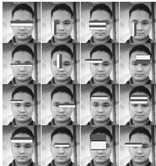
Figure 3.7: Haar-like features for face detection
