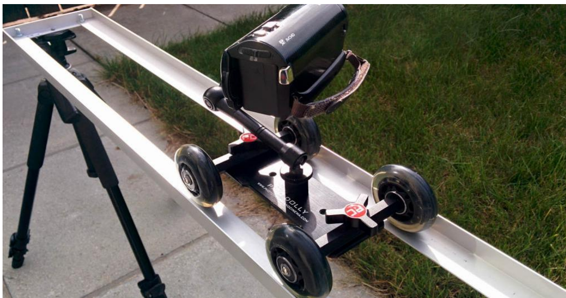
Figure: Showing the L-shape aluminum track which is similar to the track that were built for the tracking system in this project.
