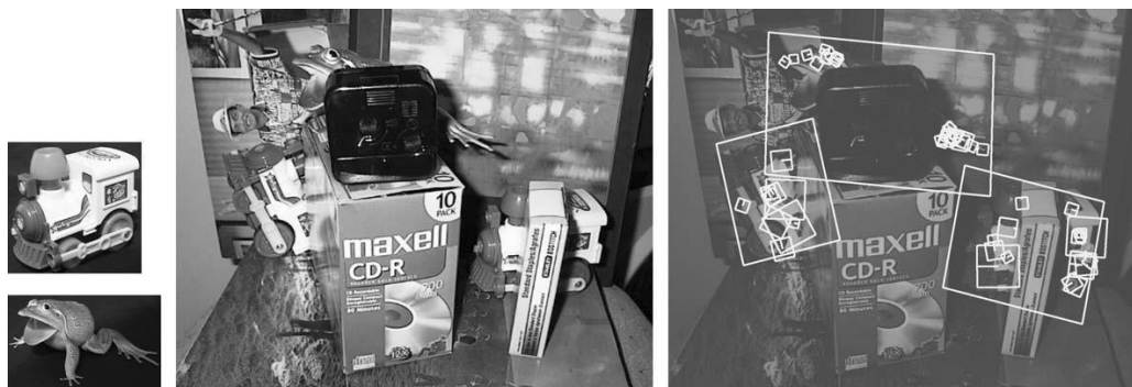
Figure 3.10: Example of how a local descriptor method, like SIFT can be used in detection of objects.
