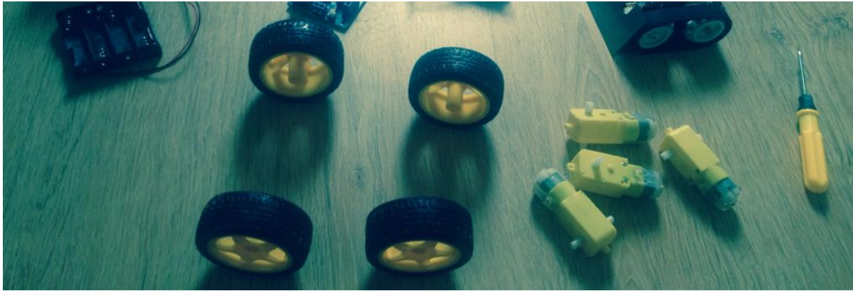
Figure 4.14: DC Driver Motors and wheels used in the automated tracking camera system.
