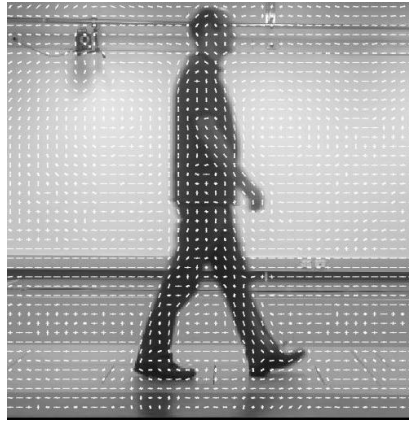
Figure 5.14 (a): Showing the oriented gradient vector in the image
