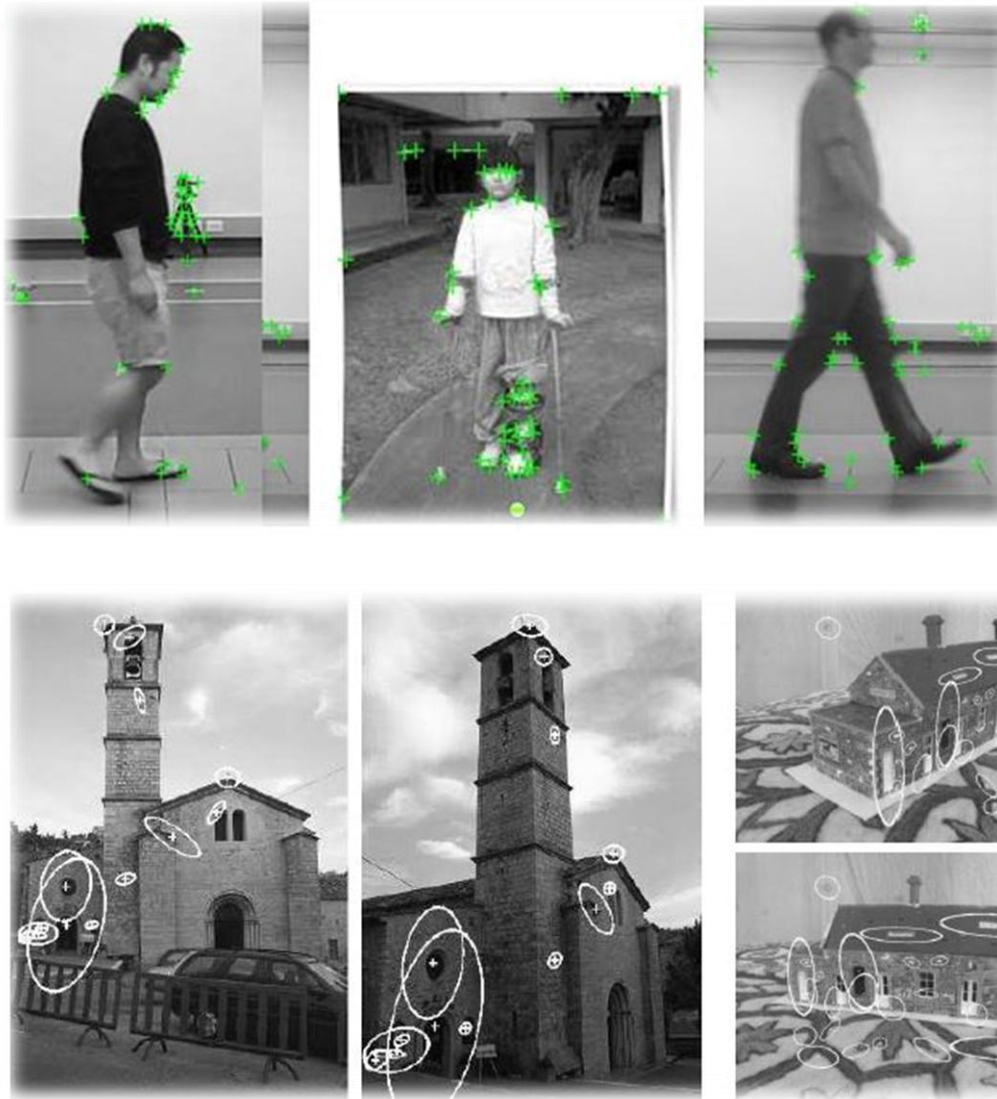
Figure 3.6: Harris point detector, detecting points in images with different viewpoints (K. Mikolajczyk and C. Schmid, 2002)
