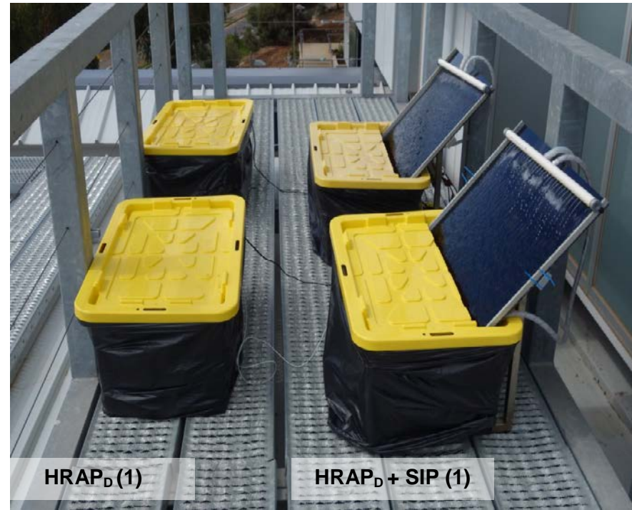
Plate 4.4: Model HRAP arrangement for operational configuration II; No-IP vs. IPs of varying length. HRAPs included a) HRAP D , b) HRAP D + Long IP (1.10 m, 0.75 m 2 ) and c) HRAP D + Short IP (0.55 m, 0.37 m 2 ).
