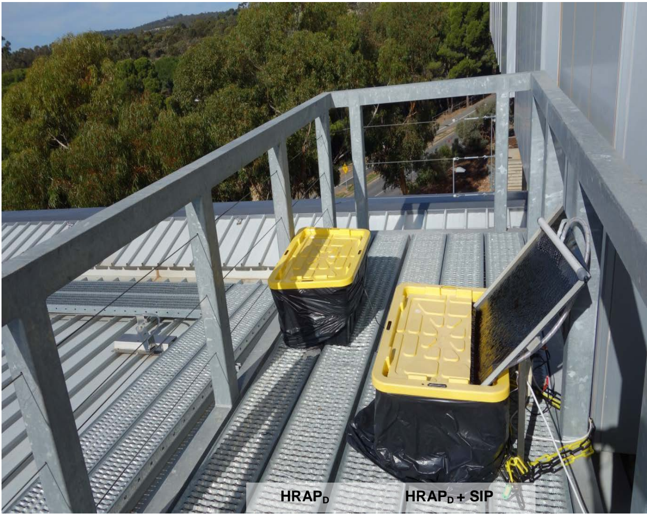
Plate 3.1: Model HRAP experimental set-up Configuration (1) HRAP D + Short IP (SIP) vs. HRAP D . Ponds were operated with optically clear (tap) water under dark incubation.
