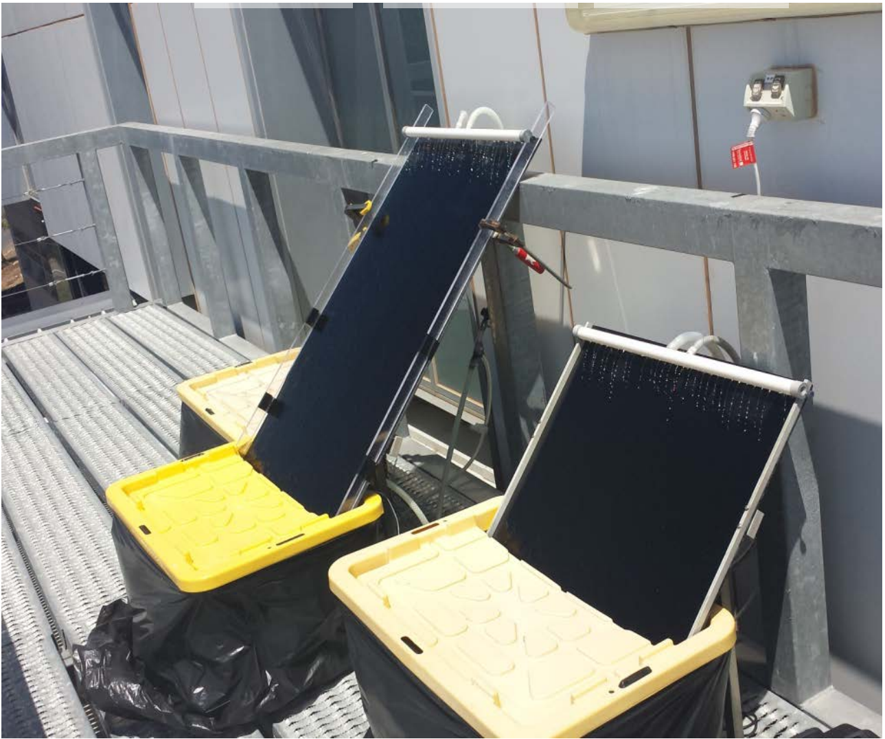
Plate 3.2: Model HRAP experimental configuration 2: HRAP D vs. HRAP D + Short IP (SIP) (0.55 m) and HRAP D + Long IP (LIP) (1.10 m).
