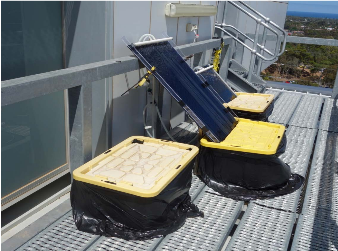
Plate 2.3: Model high rate algal ponds (HRAPs) with an included inclined plane (IP). Systems included a HRAP without an IP, and an HRAP with a Long-IP (HRAP + LIP: 1.10 m, 0.75 m 2 ) and a Short-IP (HRAP + SIP; 0.55m, 0.37 m 2 ). Shown are the model systems when dark incubated with the bulk water covered with the IP exposed to sunlight
