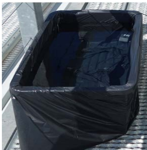
Plate 2.2: Pond lining; Photographed example of a fully lined pond.
