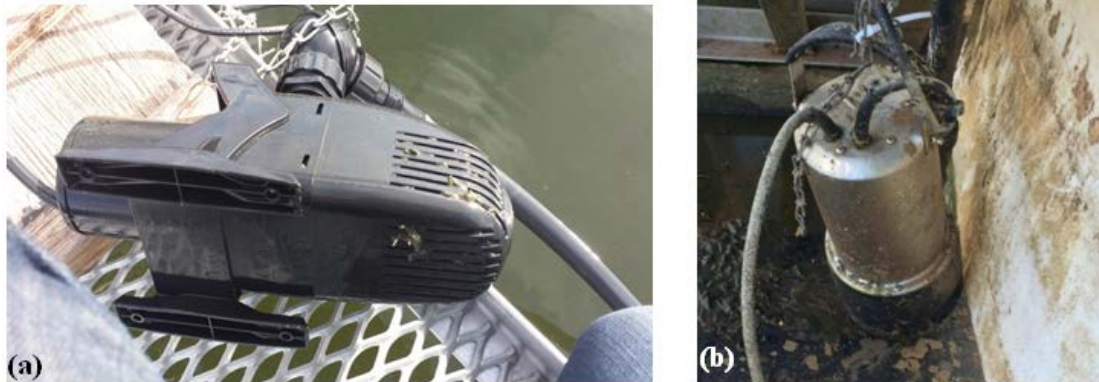
Plate 2.11: Submersible pumps used for IP operation at Kingston on Murray (KoM): a) Aqua Pro™ AP7500 multi-use pump and b) unspecified submersible pump
