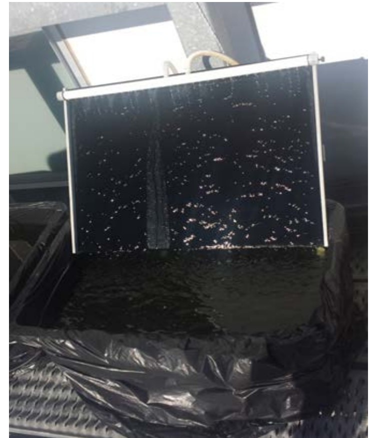
Plate 2.4: Example of the solar exposed model HRAPs. Show is the HRAP + SIP (Short-IP, 0.55 m and 0.37 m 2 ) when bulk water and IP are solar exposed.
