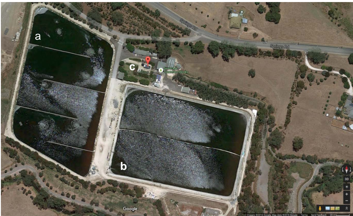
Plate 4.1: Aerial view of Mt Barker WWTP; including the a) aeration lagoon, b) polishing lagoon and c) dissolved air filtration (DAF) plant and sample collection site. Image available from https://www.google.com.au/maps/@-35.0699777,138.8749558,787m/data=!3m1!1e3
