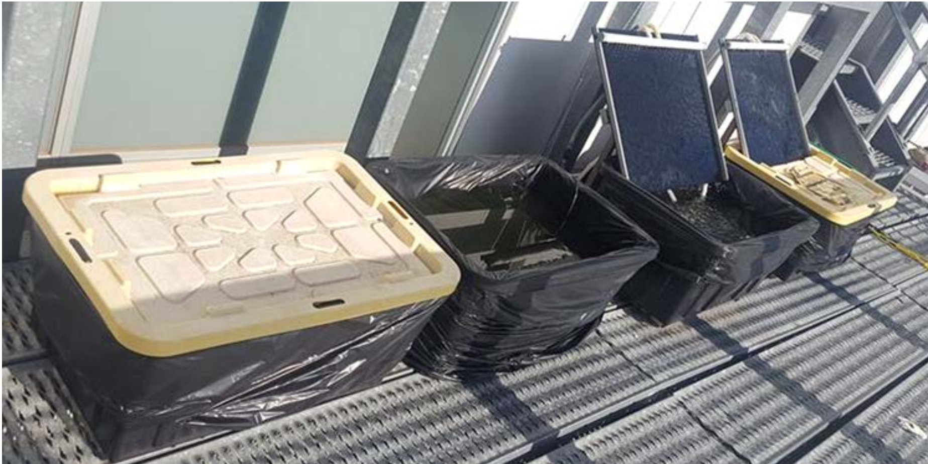
Plate 5.1: Model HRAPs arrangement for operational configuration II; comparison between open and covered HRAPs; a) HRAP D , b) HRAP L , c) HRAP L + IP and d) HRAP D + IP, where IP of 0.37 m 2 (0.55 m) was used.
