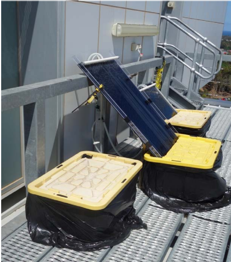
Plate 4.3: Model HRAP arrangement for operational configuration II; No-IP vs. IPs of varying length. HRAPs included a) HRAP D , b) HRAP D + Long IP (LIP; 1.10 m, 0.75 m 2 ) and c) HRAP D + Short IP (SIP; 0.55 m, 0.37 m 2 ).
