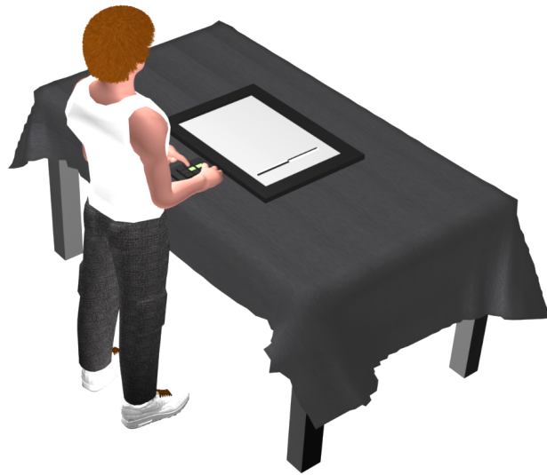
Figure 8.1: An illustration of the experimental setup. A computer screen was inserted into a table allowing participants to view stimuli on the transverse plane. The illustration shows a radial line to the participant's right
