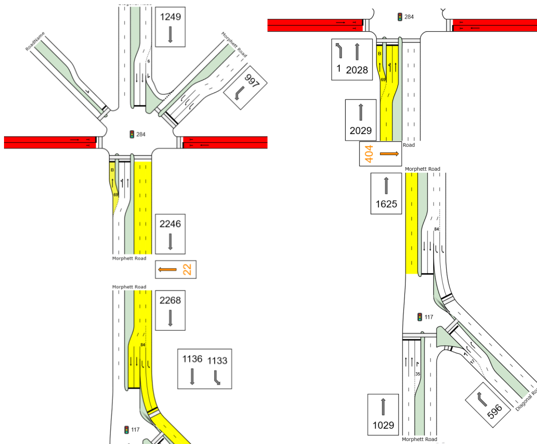
Figure 14. Network flow from SIDRA
