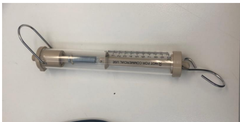
Figure 21. 10 N dynamometer used for prototype experiments
