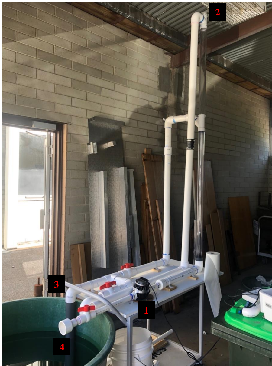
Figure 10 The setup of the flow cell. (1) is the flow meter, (2) is where the load cell is positioned, (3) and (4) are the entrance and exits respectively.
