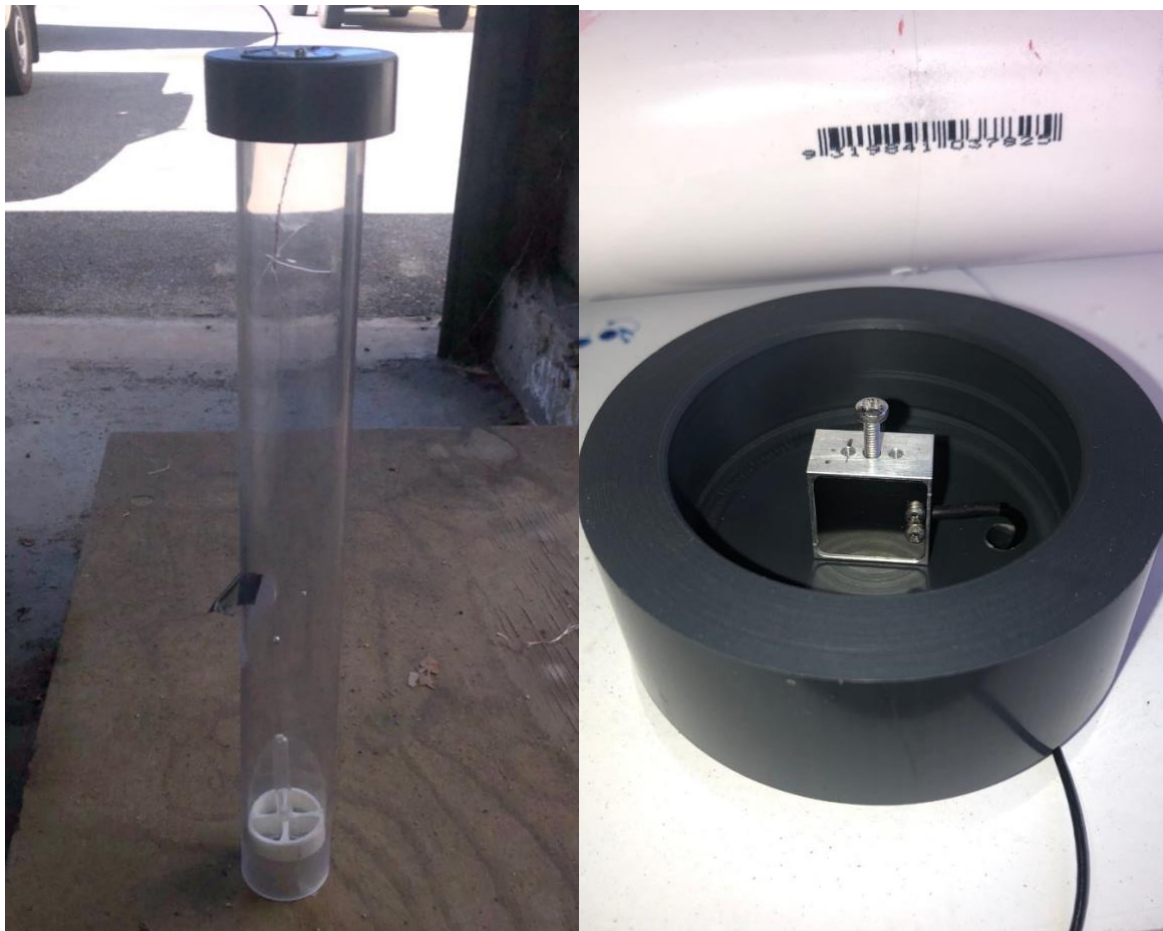
Figure 11. Mock-up showing what the very top of the section looks like, with the PVC cap containing the load cell and the specimen suspended beneath it (left). The inside of the PVC and the load cell (right).
