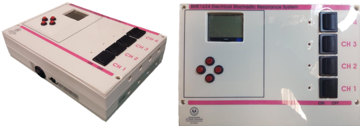
Figure 5 Previous ESRS System (isometric and front face views) showing the user interface, 4 push-buttons and channel selection switches
