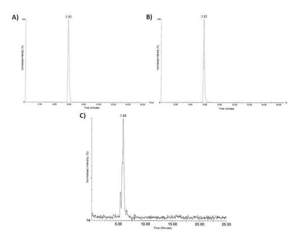
**Figure 4.14:** Trace of MS detection of HPLC separated samples; A) 2-keto-L-gulonate standard, eluting 5.85 minutes. B) L-idonate standard, eluting 5.85 minutes and C) TC59682 end-point assay, major peak eluting 5.88 minutes. Performed by Flinders Analytical Services
