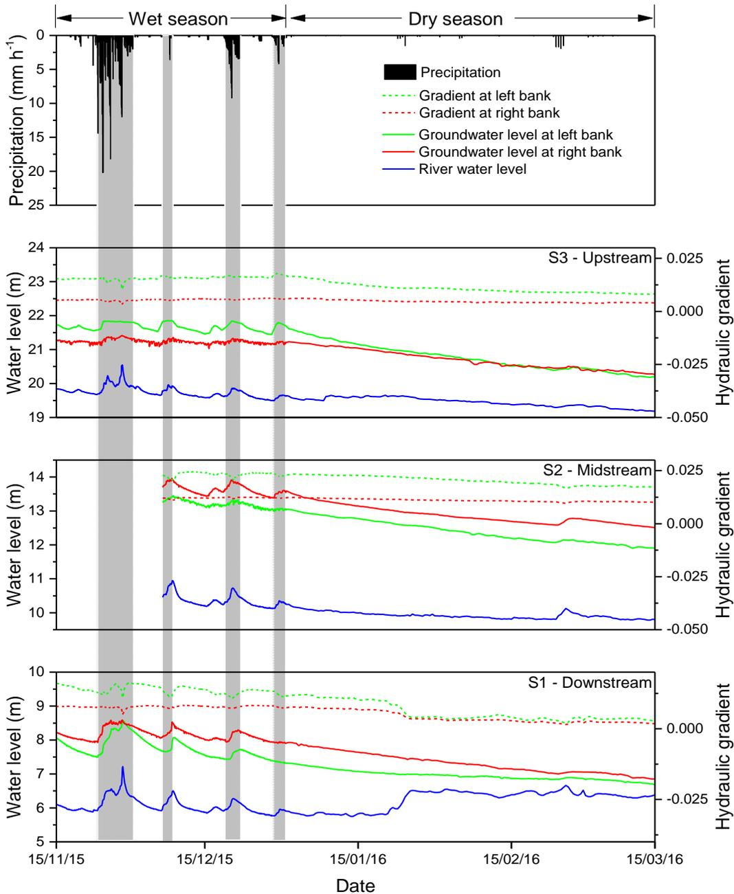
Figure 2.3: Local precipitation (top) and measured water levels and gradients in the three cross-sections from 15 November, 2015 until 15 March 2016. Grey shaded periods show the days of storm events.
