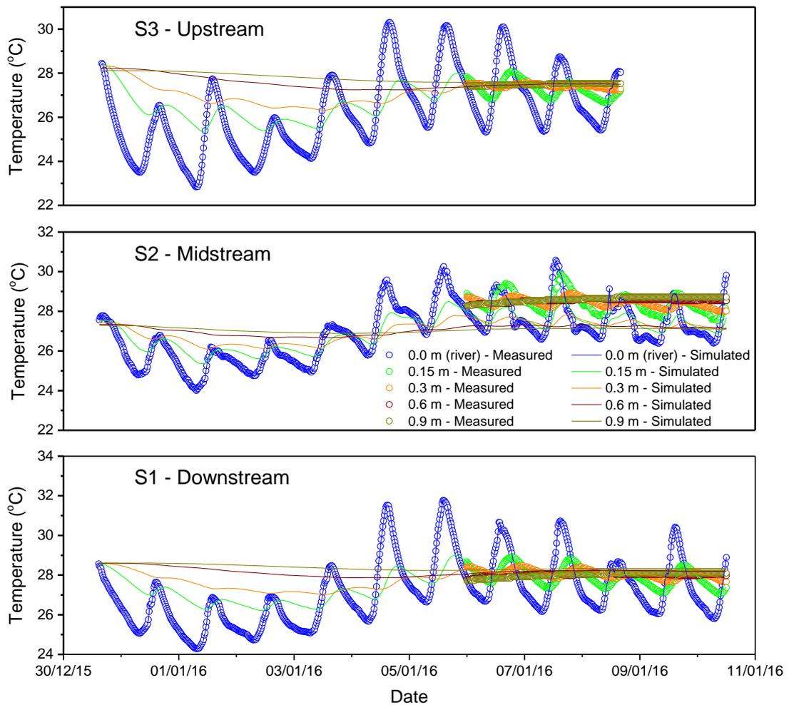
Figure 2.4: Comparison of measured and simulated temperatures in the river at 0.15, 0.3, 0.6 and 0.9 m in the river bed for the three simulated sites over the calibration period. Temperature measurements in the river bed start 6/1/2016.
