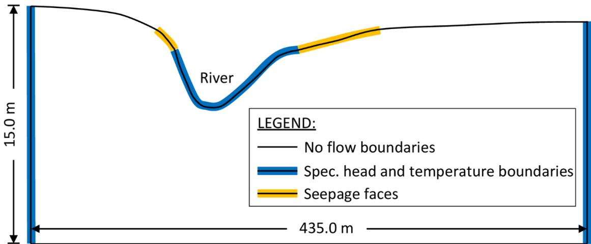
Figure 2.2: Model setup for the downstream cross-section (S1). Boundary conditions for the other cross-sections were the same, but the shape of the cross-section was slightly different (based on the survey data).
