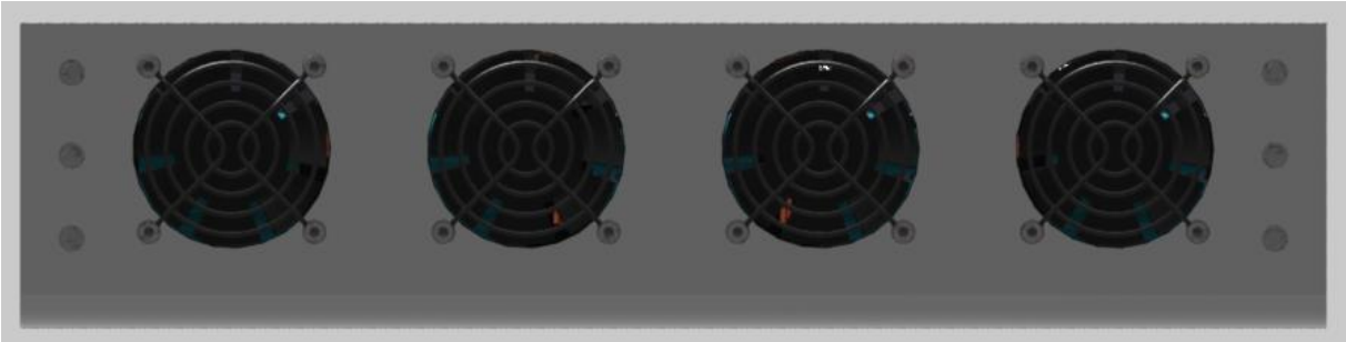
Figure 3-38. The side-view of the ESS enclosure's inlets, showing the use of finger guards and ACFs.
