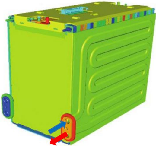
Figure 2-6. CAD model of a battery pack that uses indirect liquid cooling, blue arrows indicate coolant input and red arrows indicate coolant output [50].
