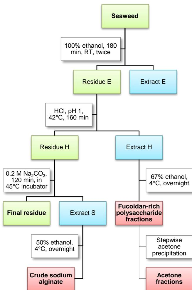
**Figure 1. Overview of the sequential biorefinery extraction process**
