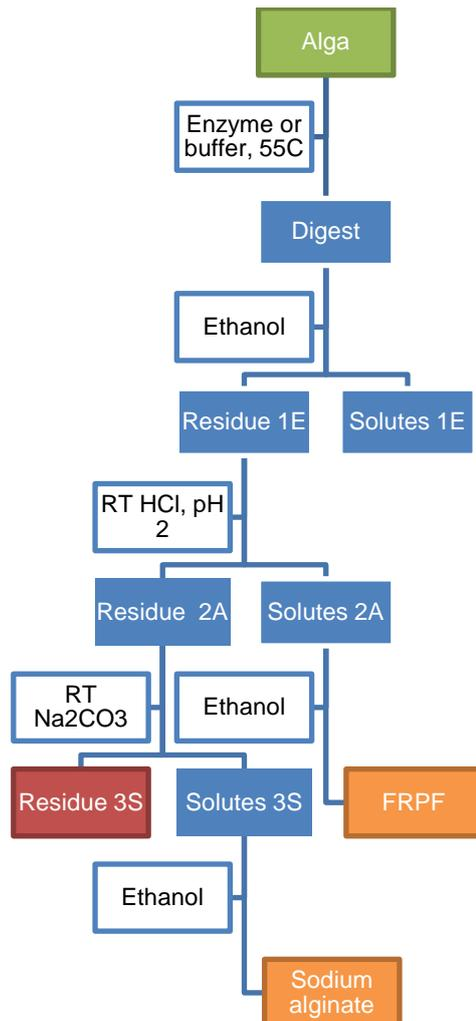
Figure 3.8. Flow chart of the enzyme treatment and sequential extraction process
