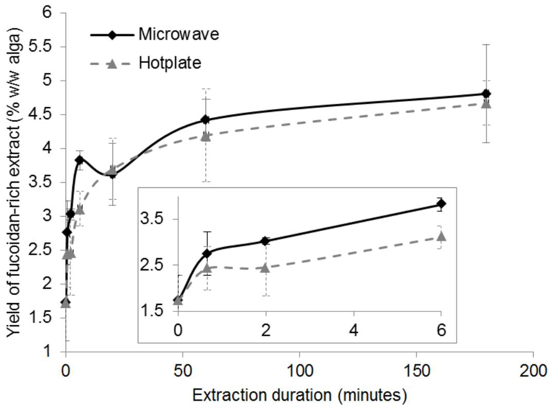
Figure 3.2. The yield of fucoidan-rich extract achieved using the microwave and hotplate throughout the 180 minutes extractions. And inlay: the same plot, zoomed in to better show the 0-6 minute period. Error bars indicate standard deviation (n=3).
