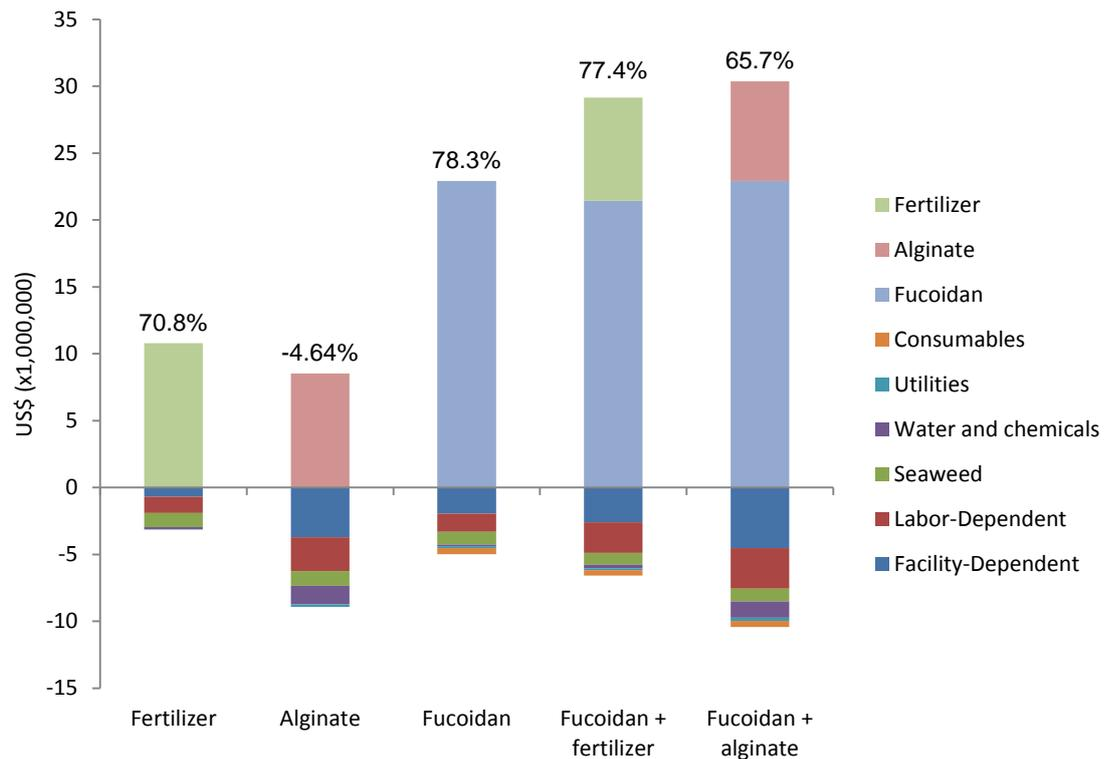
**Figure 7. Annual operating costs and revenues of the different processes, when operating at full-time capacity**
