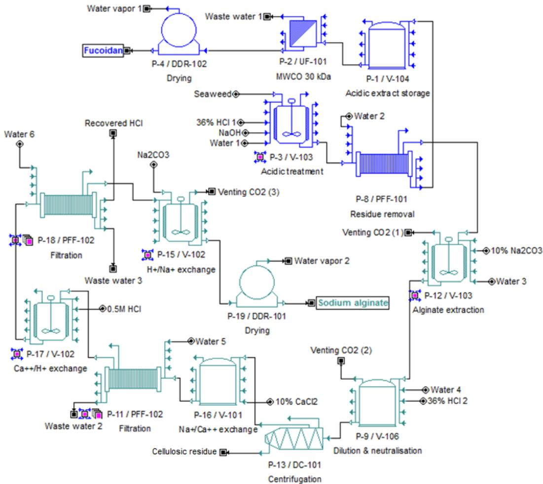
Figure 5. Integrated fucoidan and alginate production process flow-chart
