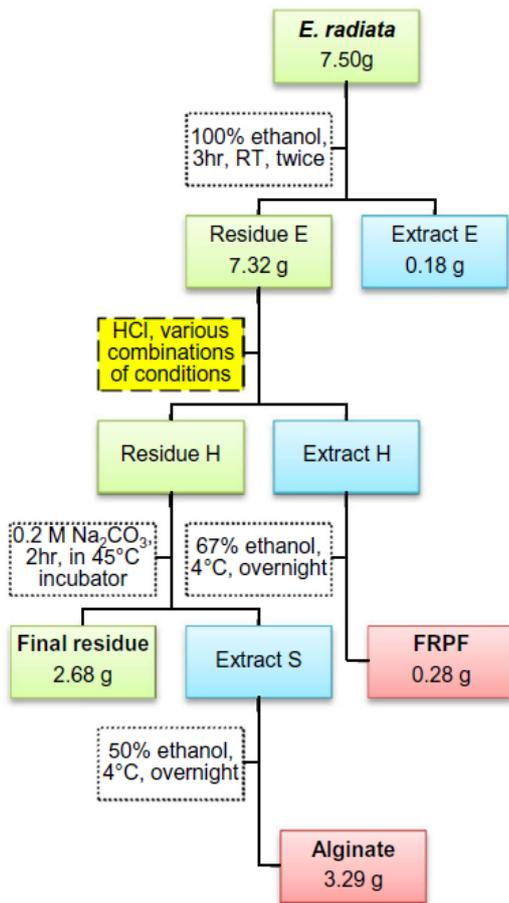
**Figure 4.1. Overview of the sequential biorefinery extraction process.**
