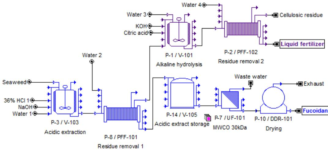
Figure 4. Integrated fucoidan and fertilizer production process flow-chart
