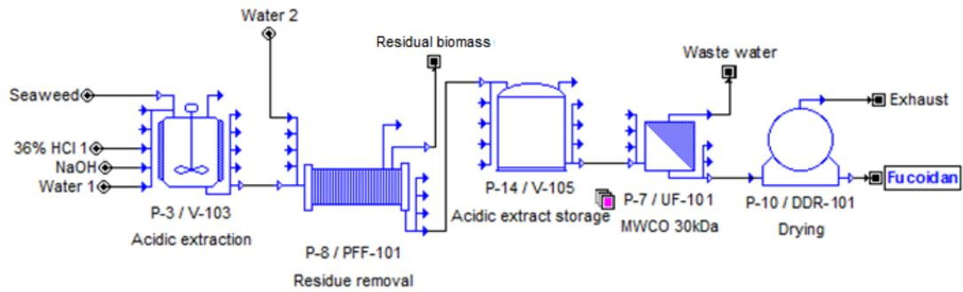
**Figure 1. Fucoidan production process flow-chart**
