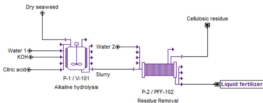
**Figure 3. Fertilizer production process flow-chart**
