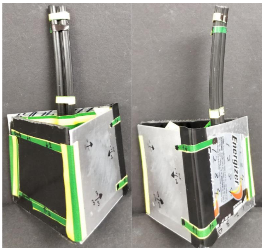
Figure 6.1. Five sample units, comprised of twin-core insulated wire, a peeled battery mounted on aluminium sheeting, aluminium sheeting, electrical tape, and polypropylene plastic. Each sample within the sample unit contains reference points for DD visualisation and sample ID information.
