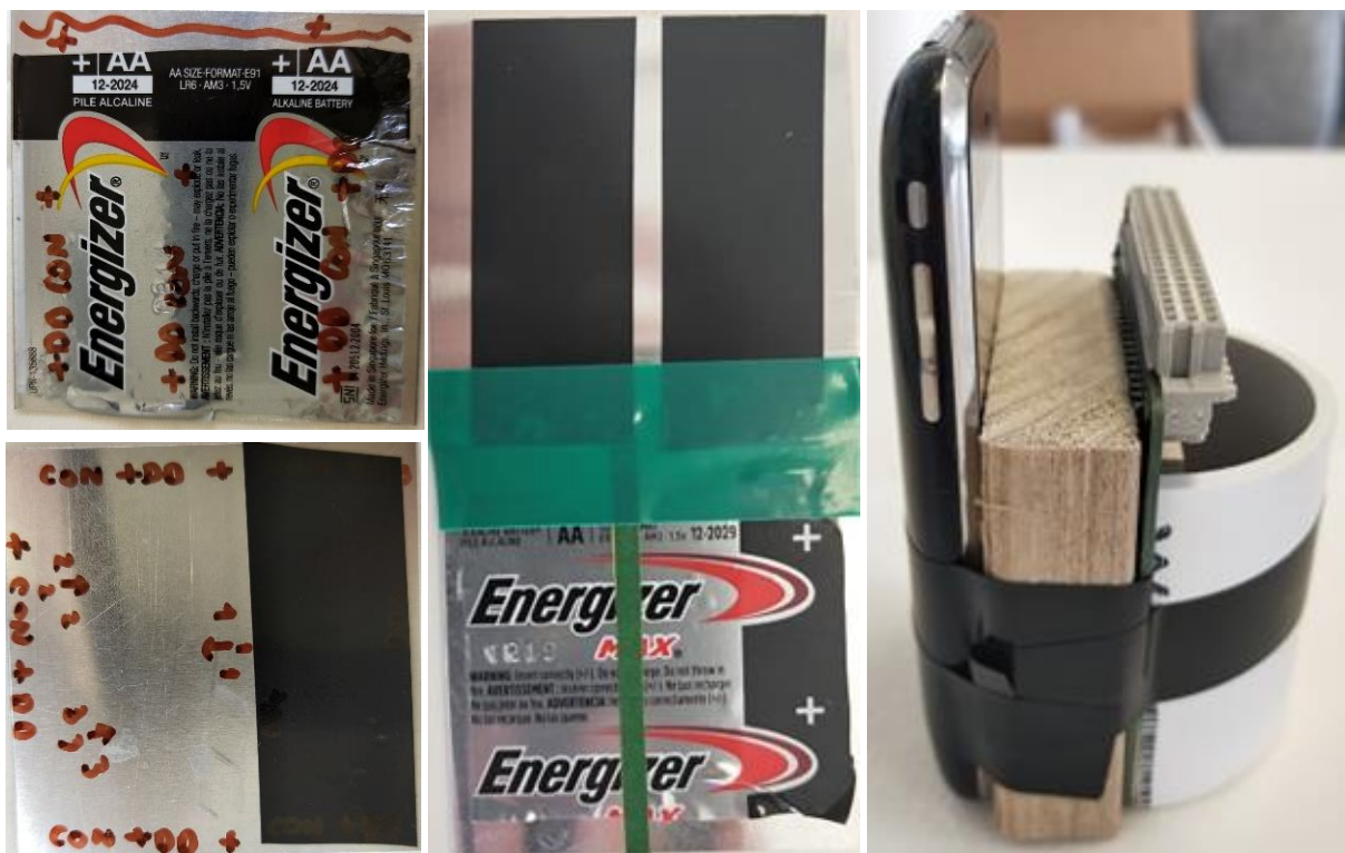
Supp. Figure 6.7. Sample units for Trial 1 (left), Trial 2 (middle), and Trial 3 (right). Sample units are comprised of the following: a peeled battery mounted on aluminium sheeting, aluminium sheeting, and electrical tape for Trail 1; a peeled battery mounted on aluminium sheeting and electrical tape for Trial 2; and a mobile phone, SIM card, pine wood, circuit board, and PVC for Trial 3. Each sample within the sample unit contains reference ID information.
