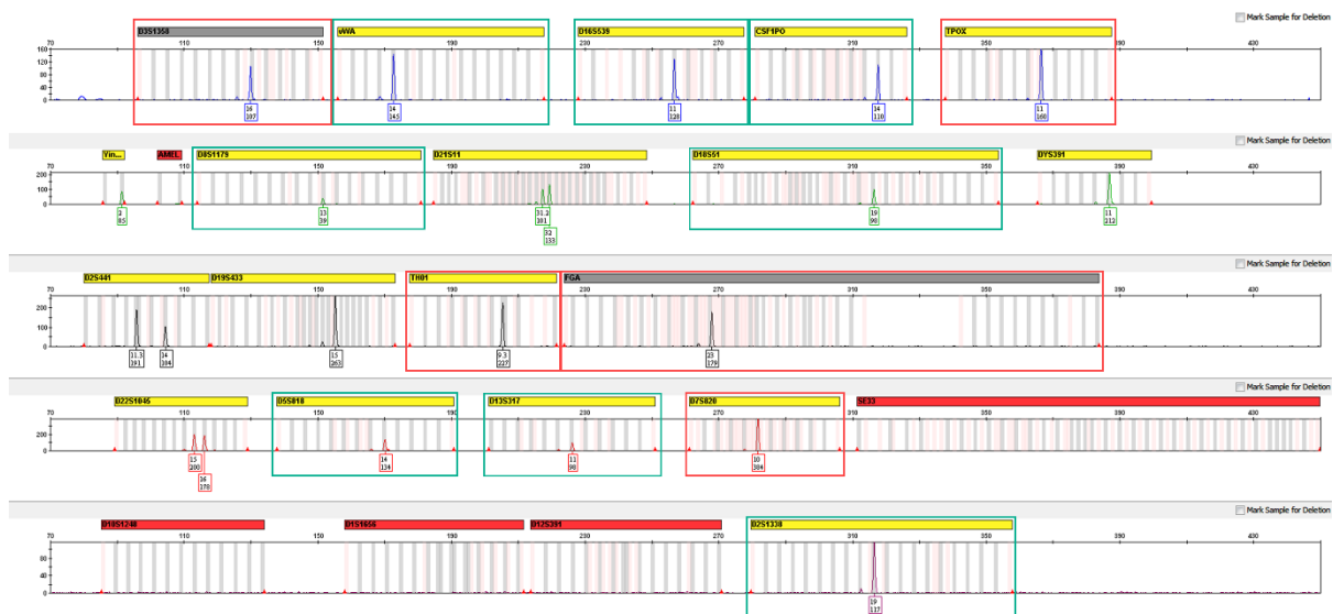
Figure 3.23. Example of a profile showing high unexpected homozygosity. The green boxes are around loci that are expected to be heterozygous but are below the 150 RFU threshold to be considered. The red boxes are around loci that are above 150 RFU and are therefore called as false homozygotes.
