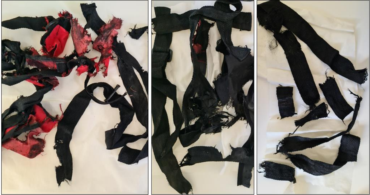
Supp. Figure 6.11. Post-detonation canvas bag fragments from the straps taped/lifted for STR analysis. Bags were placed immediately next to the charge.
