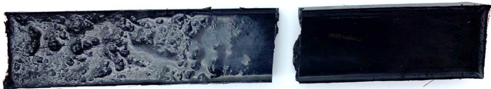
Figure 5.61: Cured polymer reinforced with carbon nanotubes (1.0 g) after three point bent test showing site of structural failure.
