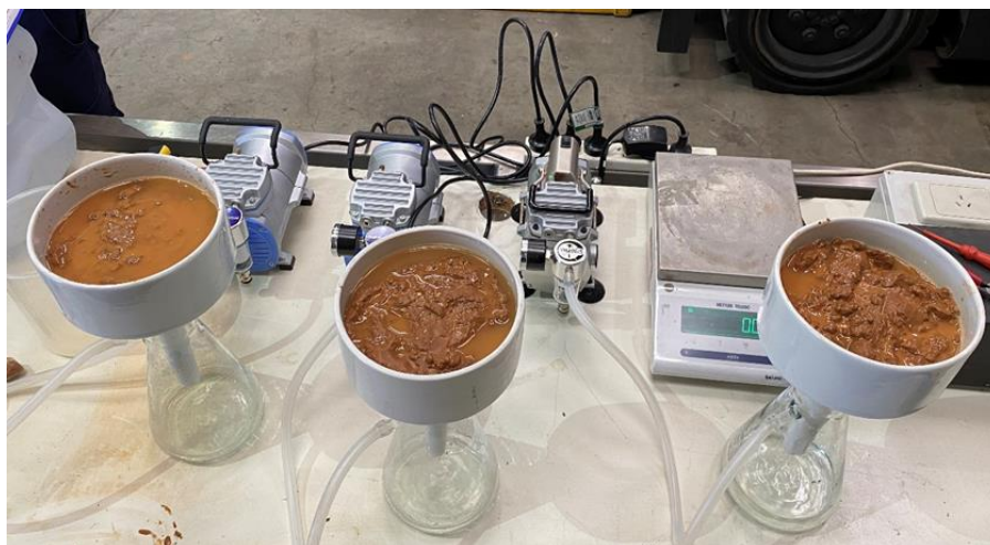
Figure 2.110: Ore is being filtered using vacuum filtration.
