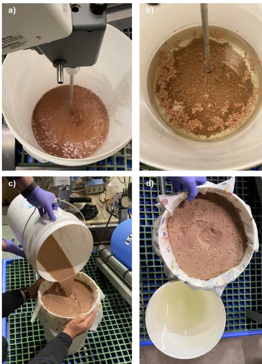
Figure 2.111: a) filtered leach solution and 50-poly( S-r -canola) polymer being stirred, b) solution after 30 minutes stirring, c) filtration through cloth and d) recovered polymer and leach solution after gold uptake.
