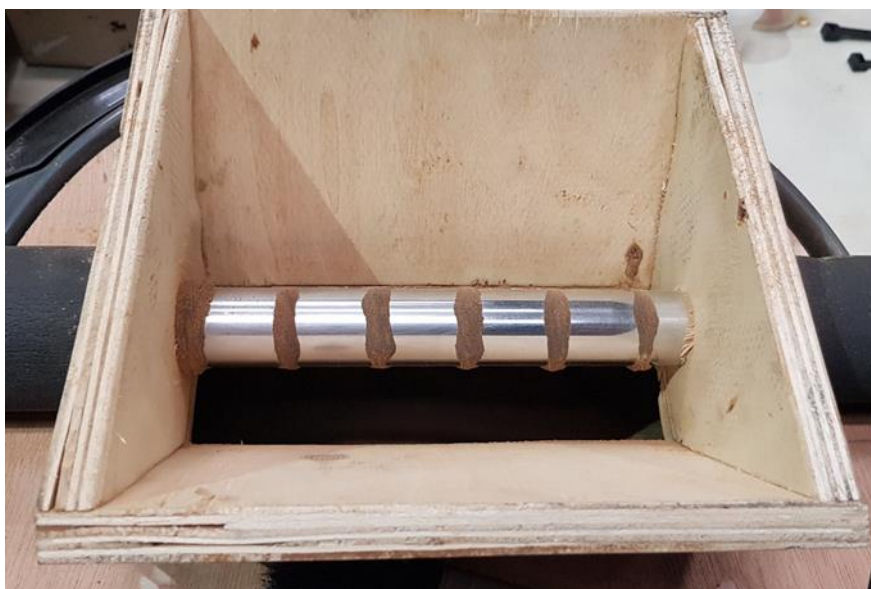
Figure 2.46: Magnetic material was removed by pouring the ore over a strong tubular magnet.
