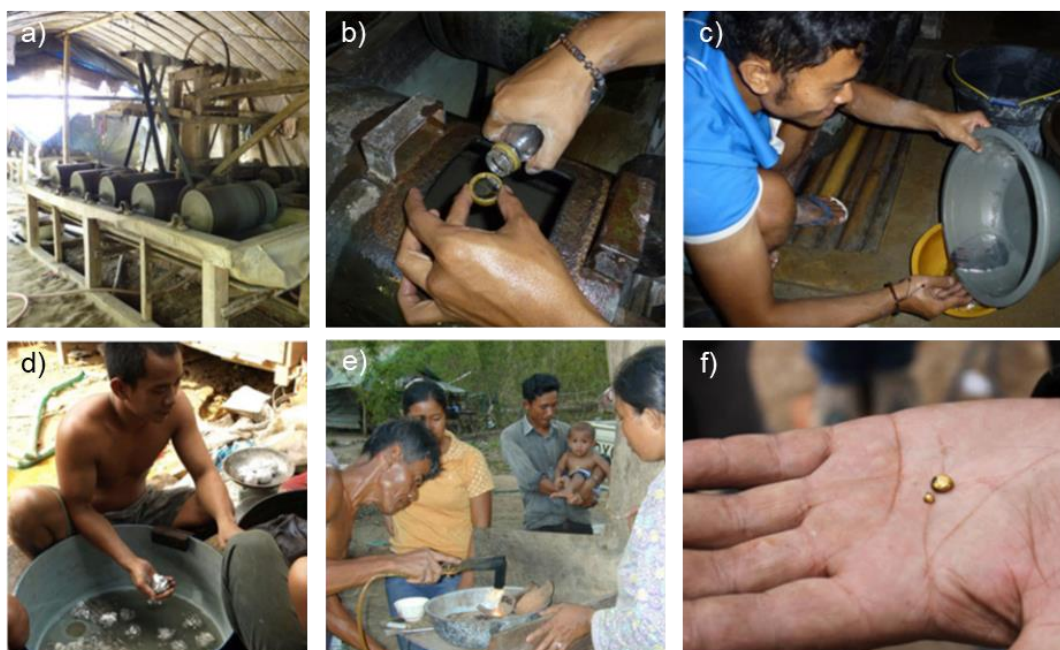
Figure 2.2: Gold recovery process in ASGM. a) Gold bearing material is crushed and mixed with water in mills. b) Mercury is added to the crushed material (up to 1 kg per 20 g of ore). c) After the amalgamation process the remaining mercury is recovered. d) Gold-mercury amalgam is recovered. e) The mercury in the amalgam is removed by a blow torch. f) Isolated gold from an artisanal mine. Image reproduced under a Creative Commons CC-BY-NC license. 3
