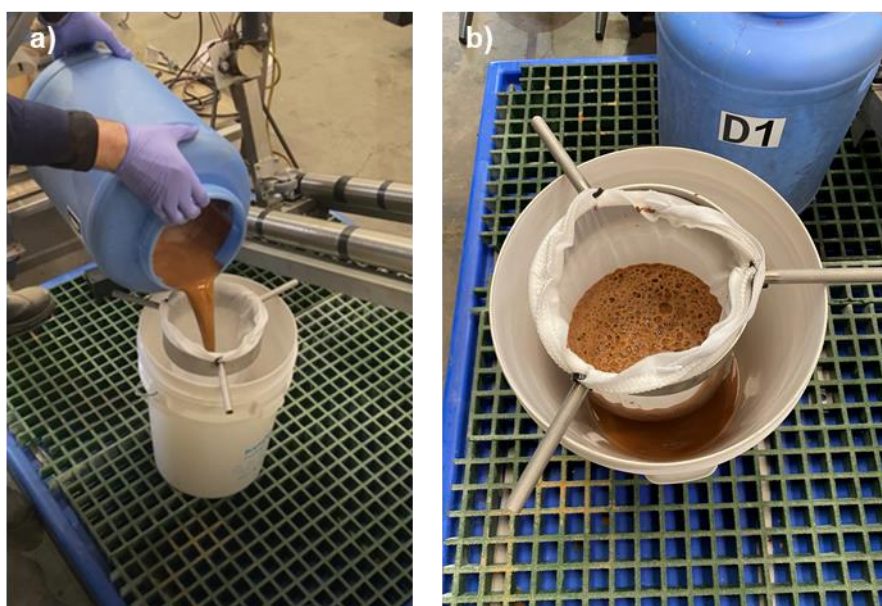
Figure 2.109: a) reaction mixture is being poured into 50 \mu\text{m} nylon filter bag, b) top view of filter bag.
