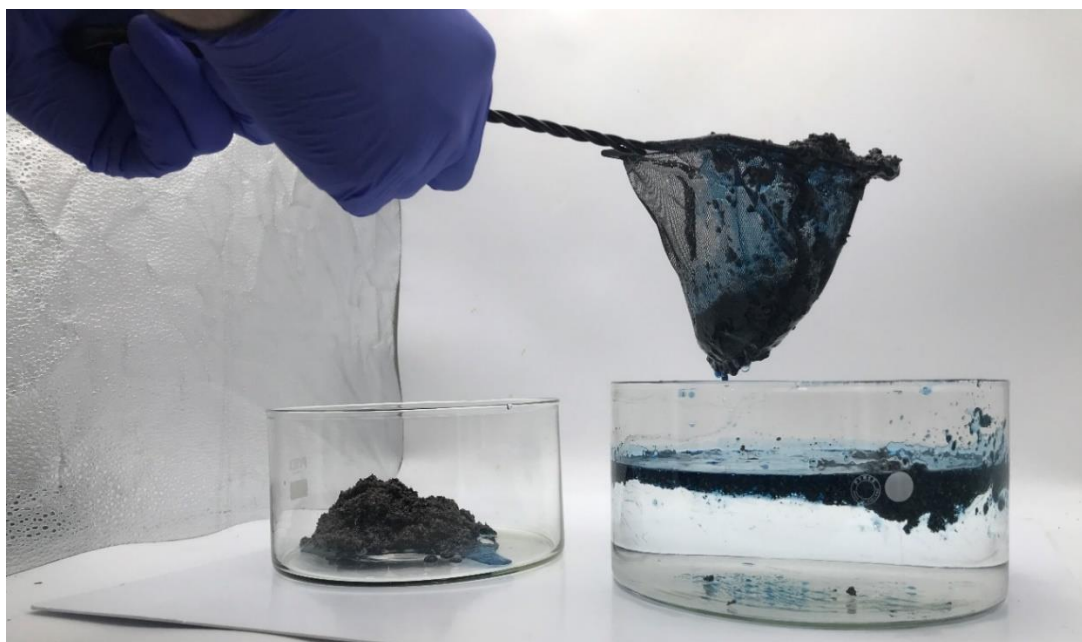
Figure 3.38: Removing the 50-poly( S-r -canola) polymer and oil mixture from the water using a net. Reproduced with permission from the Royal Society of Chemistry. 45
