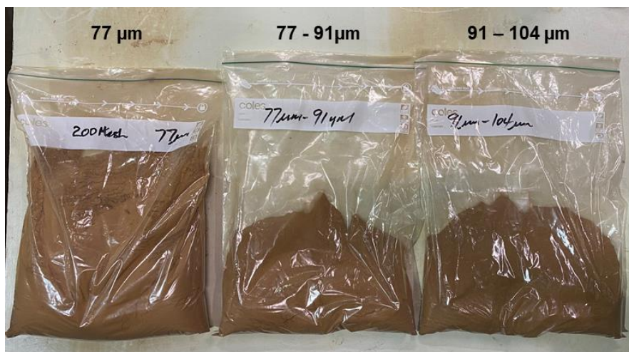
Figure 2.105: Ore used for this experiment classified into three size ranges (77 \mu\text{m} , 77 – 91 \mu\text{m} , 91 – 104 \mu\text{m} ) with a total mass of 4759.4 g
