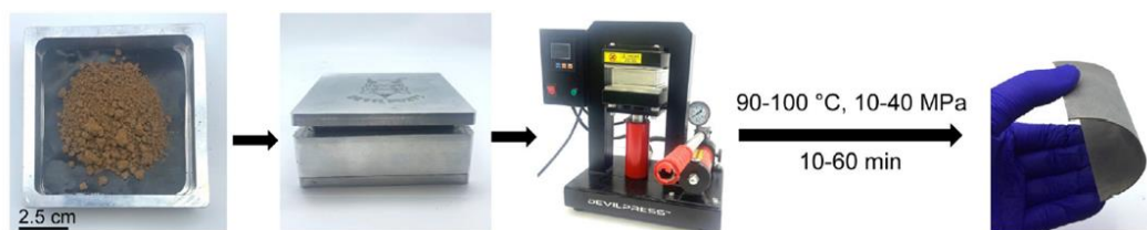
Figure 4.3: A sulfur-canola oil polymer is processed by active compression moulding which results in flexible polymer mats. © 2020 Wiley-VCH Verlag GmbH & Co. KGaA, Weinheim. Images reproduced under a RightsLink license. 14
