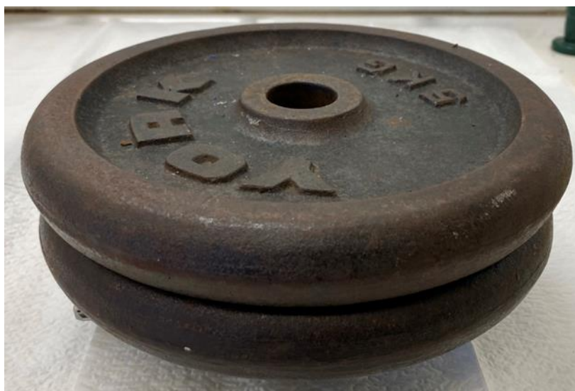
Figure 5.49: 10 kg weight on polymer samples after triethylamine adhesion was started. © 2021 Wiley-VCH GmbH. Image was reproduced under a RightsLink license. 24
