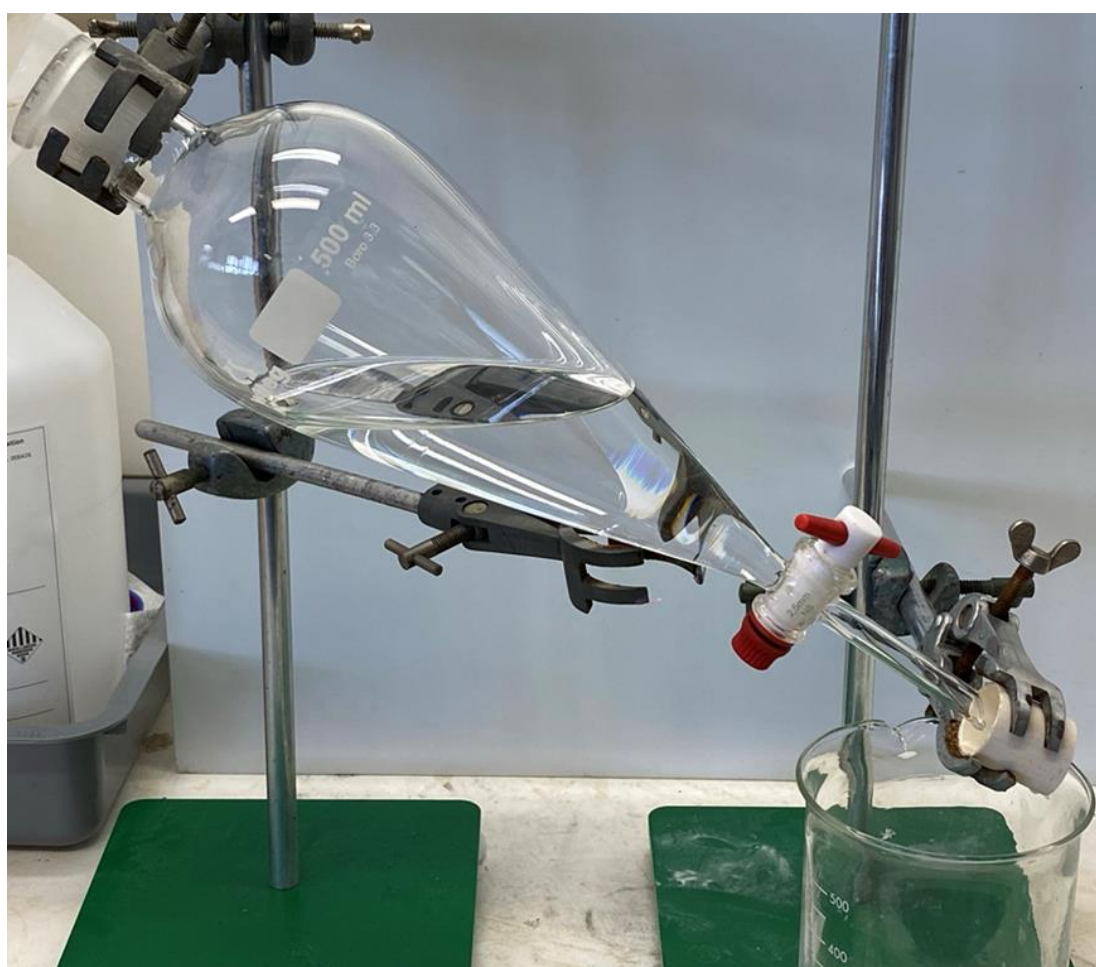
Figure 4.97: A separator funnel was set up so that a steady flow of 5 mL/min of THF could pass through the uncoated PVC pipe. Reproduced with permission from the Royal Society of Chemistry. 25
