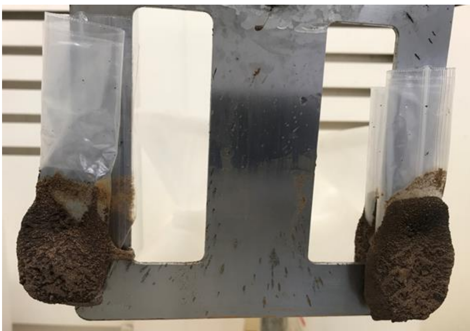
Figure 2.99: Magnetic material stuck to the magnets attached to the stirrer bar.
