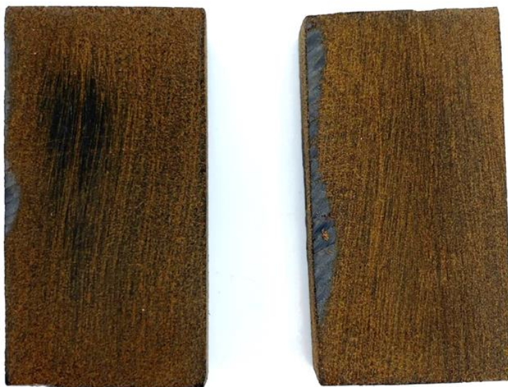
Figure 5.48: Polymer pieces with sandpaper treated surface ready for adhesion using triethylamine. © 2021 Wiley-VCH GmbH. Image was reproduced under a RightsLink license. 24
