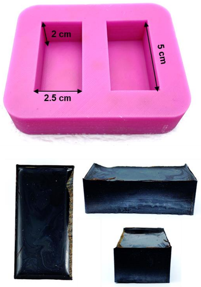
Figure 5.29: Silicon mould into which the liquid polymer is poured prior to curing and cured polymer block. © 2021 Wiley-VCH GmbH. Image was reproduced under a RightsLink license. 24
