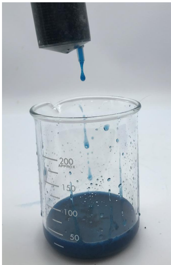
Figure 3.40: Oil removal by adding the oil 50-poly( S-r -canola) polymer mixture into a syringe and pressing the oil out. Reproduced with permission from the Royal Society of Chemistry. 45
