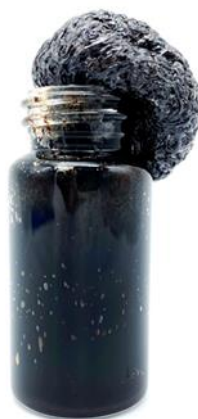
Figure 5.12: 25% DCPD reaction at 170 °C, 6.5 minutes after the canola oil and DCPD was added to the molten sulfur. © 2021 Wiley-VCH GmbH. Image was reproduced under a RightsLink license. 24
