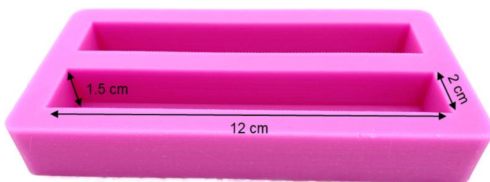
Figure 5.26: Mould for pouring polymers for three point bend testing. © 2021 Wiley-VCH GmbH. Image was reproduced under a RightsLink license. 24
