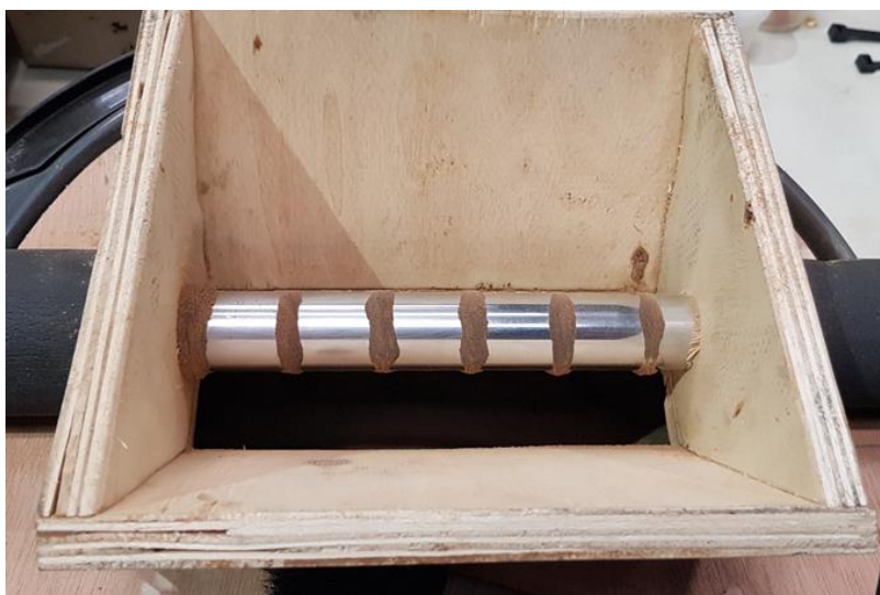
Figure 2.106: A strong tubular magnet was used to remove magnetic material from the ore.
