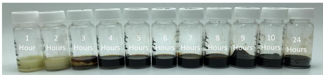
Figure 4.44: Reaction of 3.00 g DCPD and 3.00 g sulfur synthesised at 140 °C in an oven 24 hours. The image shows all samples after the final sample of 24 h reaction time was removed from the oven. Reproduced with permission from the Royal Society of Chemistry. 25
