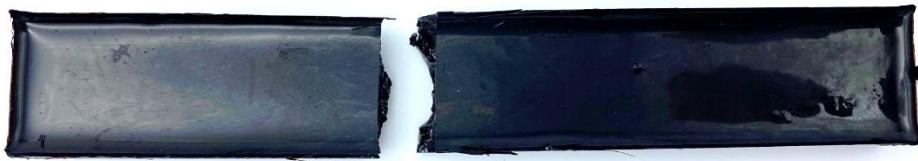
Figure 5.59: Cured polymer reinforced with carbon nanotubes (0.5 g) after three point bent test showing site of structural failure.
