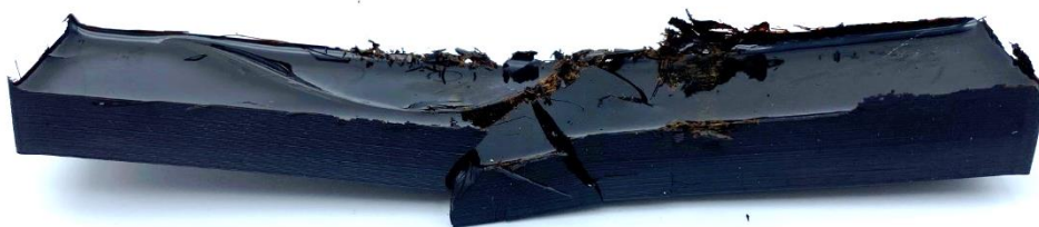
Figure 5.55: Cured polymer with loose carbon fibre (0.5 g) reinforcement after three point bent test showing site of structural failure.
