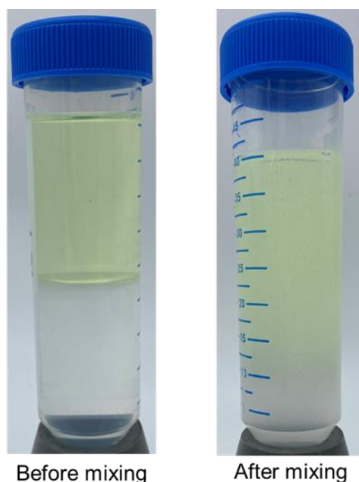
Figure 4.90: Mixture of equal volumes of diesel fuel and water before and after end-over-end mixing, illustrating the emulsion that forms. Reproduced with permission from the Royal Society of Chemistry. 25
