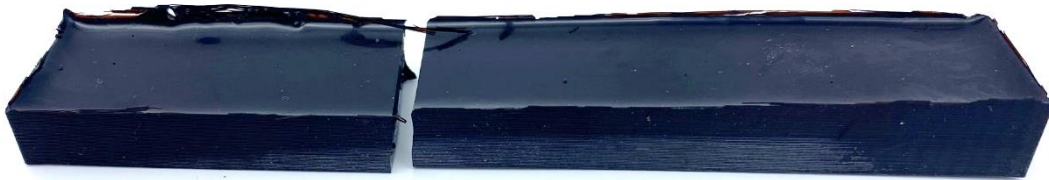
Figure 5.53: Cured polymer with no reinforcement after three-point bend test showing site of structural failure.
