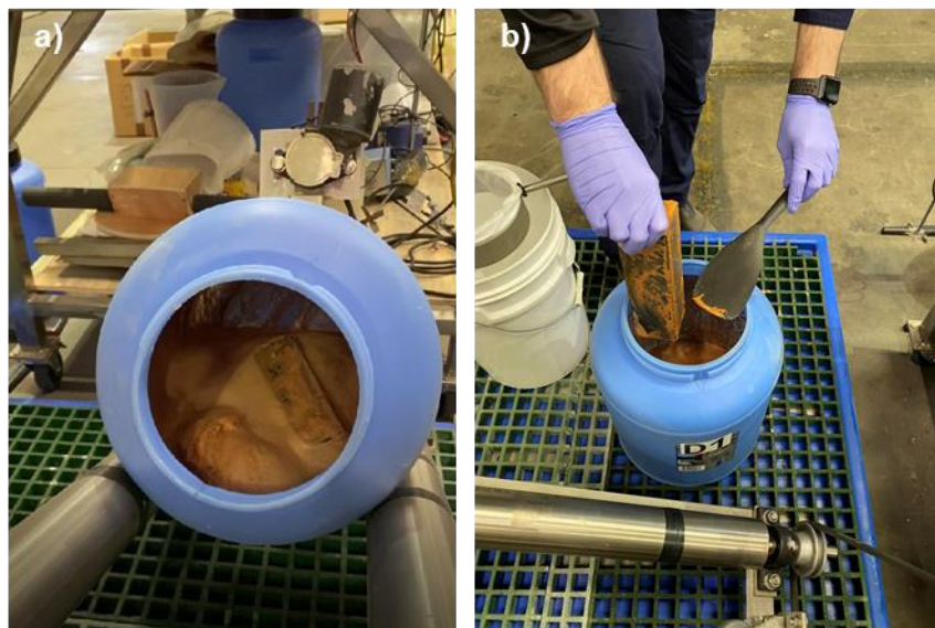
Figure 2.108: a) reaction mixture after 2 hours, b) PVC block is removed prior to filtration.
