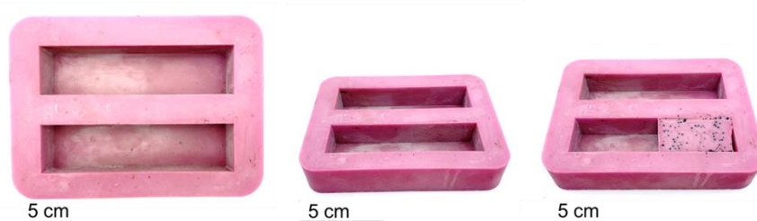
Figure 5.43: Silicon mould for polymer pouring with the dimensions of L10 cm x W2.5 cm x D2.0 cm and with a silicon block (L4 cm x W2.5 cm x D2.0 cm) fitted to minimise the volume of polymer needed to fill the mould. © 2021 Wiley-VCH GmbH. Image was reproduced under a RightsLink license. 24
