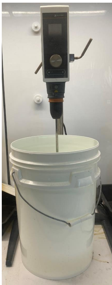
Figure 2.33: General set up for ore oxidation experiment and gold recovery experiment using the polysulfide. (20 L bucket is shown here but 5 L buckets were also used).
