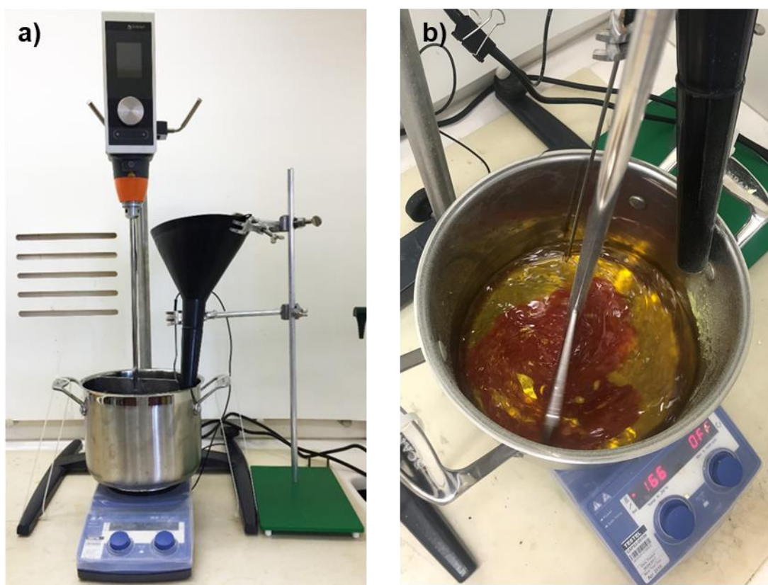
Figure 2.51: a) Set-up of 700 g poly(S- r -canola) synthesis. b) Reaction after some sulfur was added, two phases can be seen with molten sulfur at the bottom and canola oil at the top.
