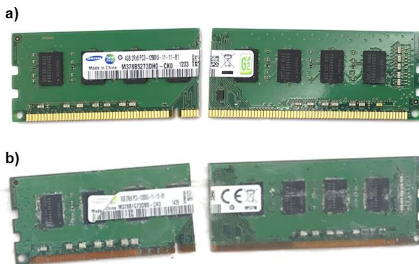
Figure 2.49: Representative RAM module a) before and b) after oxidation.
