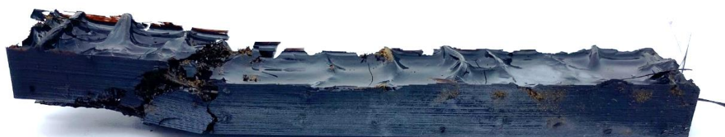
Figure 5.57: Cured polymer reinforced with carbon fibre (0.5 g) after three point bent test showing site of structural failure.
