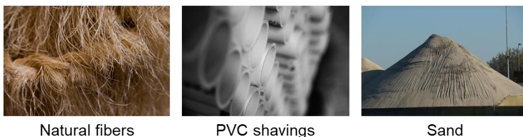
Figure 5.2: A range of natural fibres (sisal fibres 7 , coconut coir 9 and wool 8 ), PVC shavings 9 and sand 9 have been evaluated as parts of polymer composites. Image credits: Fibres: Scratching post by Andrew Malone under a CC BY 2.0 licence. PVC by pepperberryfarm under a CC BY-NC-ND 2.0 licence. Sand: Sand patters by PK under a CC BY 2.0 licence.
