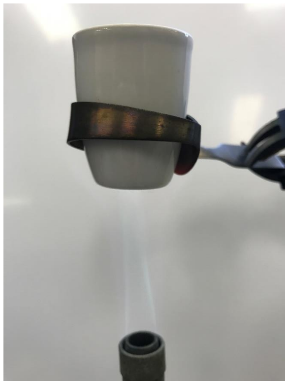
Figure 2.22: Gold bearing 50-poly(S- r -canola) polymer incineration set-up. The wet or dry polymer was placed into the crucible and a Bunsen burner was used to heat the crucible until the polymer was incinerated.
