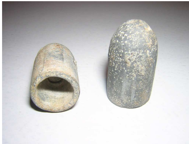
Figure 6. Two original .577 calibre minie bullets excavated from the site of a South Australian colonial militia's practice range in Old Noarlunga, South Australia (Grguric, 2005: 12-13). The impression of the firearm's rifling can clearly be seen on the example at left, in the form of lines running lengthways down the side of the bullet. These examples date from between ca 1859-1866. Author's Collection.
