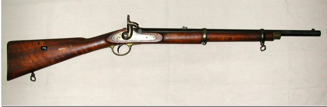
Figure 5. The Pattern 1853 Enfield rifled musket, .577 Calibre. This is the short ‘muskatoon’ model, a term which effectively means the same as ‘carbine.’ There was also a longer ‘2-band’ model and an even longer ‘3-band’ model, so designated on account of the number of barrel bands present securing the barrel to the stock. Courtesy of the South Australian Museum.
