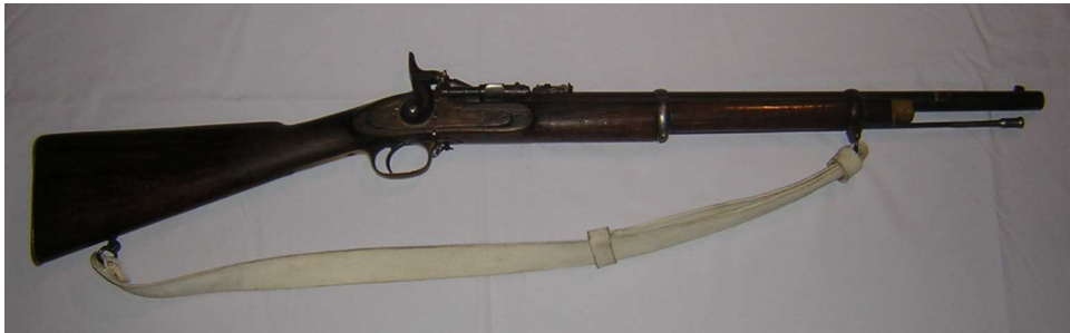
Figure 9. Snider carbine, .577 calibre. Short rifles such as these were favoured by the settlers for their handiness. This is the model known as the 'Artillery Carbine', as it was originally designed by the British for their artillerymen. Note that it is of the same basic design as the rifled musket above (figure 34) though this one is a breechloader. Author's collection.
