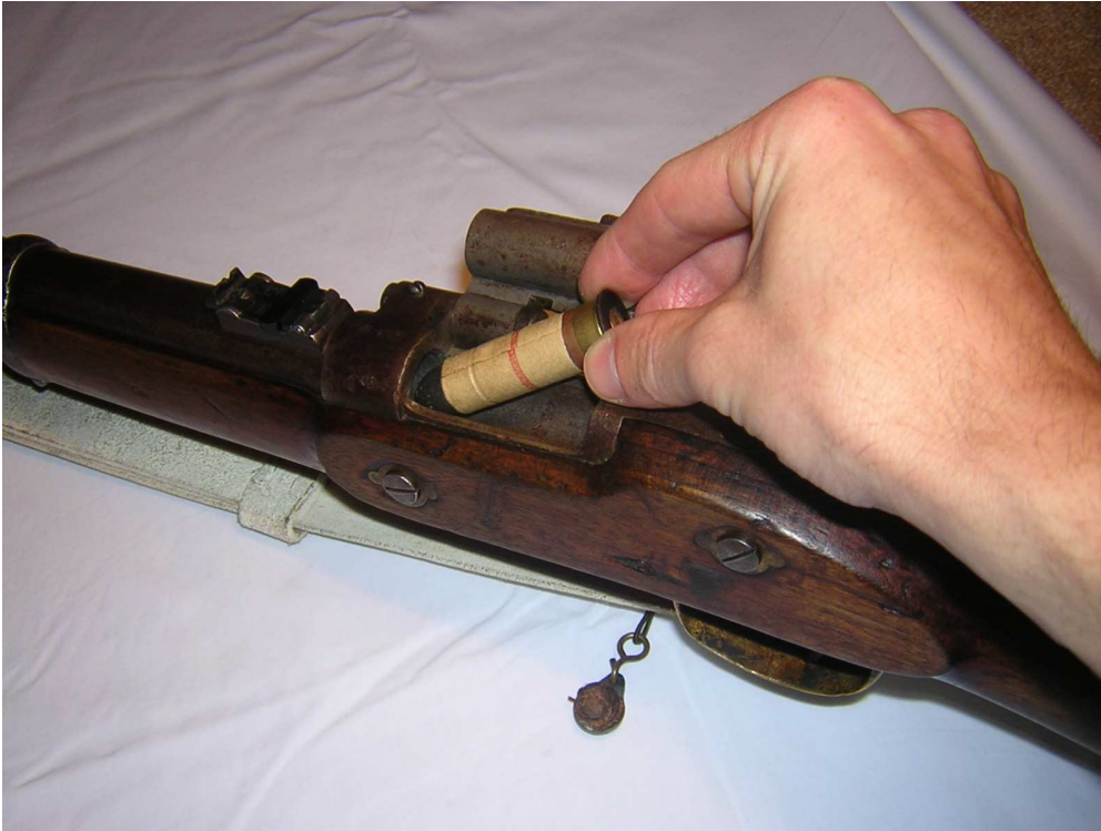
Figure 12. The loading of a single-shot breechloader. This shows a cartridge being inserted into the breech of the Snider carbine pictured above (Figure 38). Once inserted, the hinged breech-block, which can be seen to the right of the breech in the open position, is snapped shut. Author's collection.
