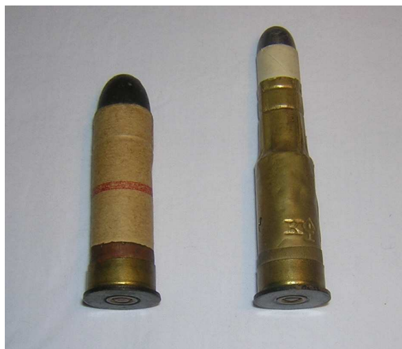
Figure 11. Cartridges for single-shot breechloading rifles. At left is a Snider cartridge, at right a Martini-Henry cartridge. The ‘primer’ which replaced the percussion cap can be seen in the centre of the bases of the cartridges. Author’s collection.
