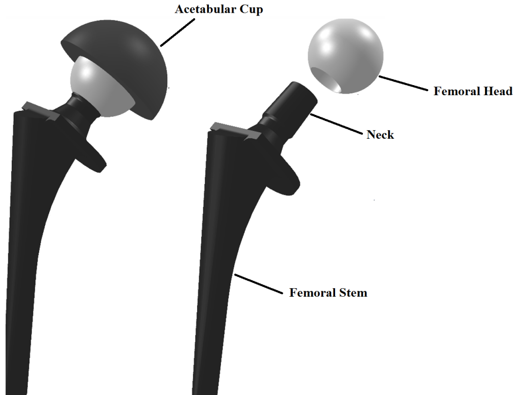
Figure 1.4- Modular design of hip joint implant
