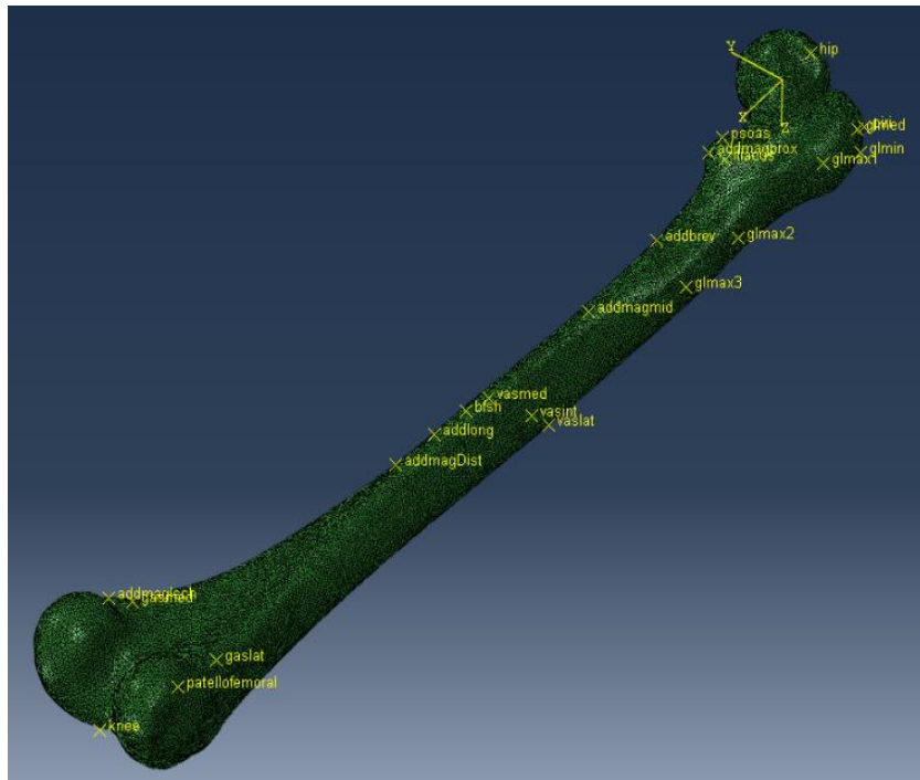
Figure 9 - Detailed FEM full femur view
