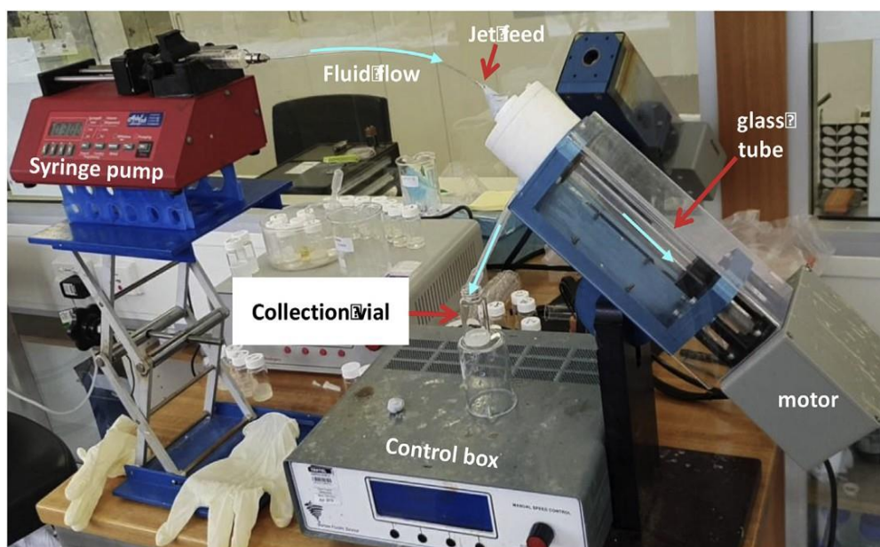
Figure 3.1: Photograph of the vortex fluidic device (VFD) highlighting its salient features. The reagents are delivered via syringe pump into the bottom of the glass tube, gets processed at optimized conditions and collected in the vial.
