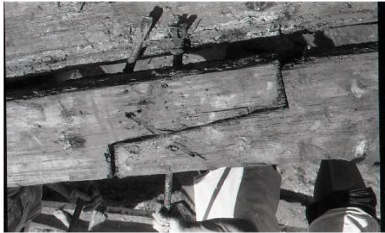
Figure 5-17 Stopped scarf joint of the bulkhead plank fastened by an iron clamp Courtesy of Museum of Overseas Communication History
