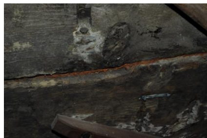
Figure 6-22 Vegetable fibre identified in the seam of the bulkhead planks. Photo by author
