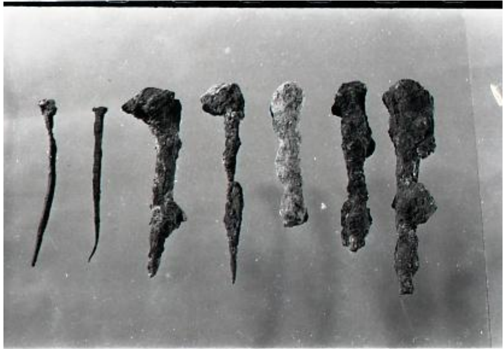
Figure 8-5 Photograph of the degraded iron nails from the Quanzhou ship. Courtesy of Museum of Overseas Communication History
