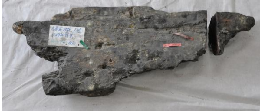
Figure 8-14 Specimen cut from the hull plank SW-82-182. Photo by author
