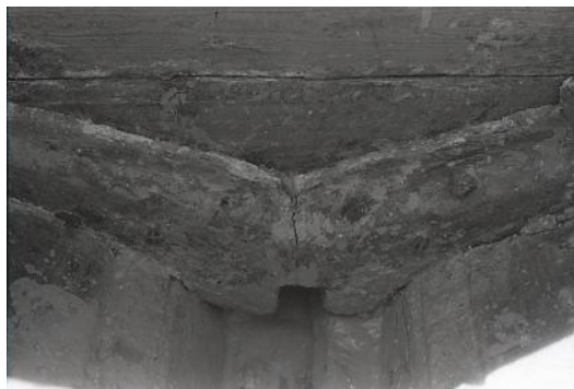
Figure 5-28 Large half-frames attached into the bulkheads. Courtesy of Museum of Overseas Communication History
