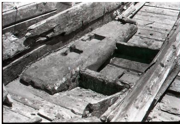
Figure 5-30 Old photograph of the main mast step after excavated. Courtesy of Museum of Overseas Communication History
