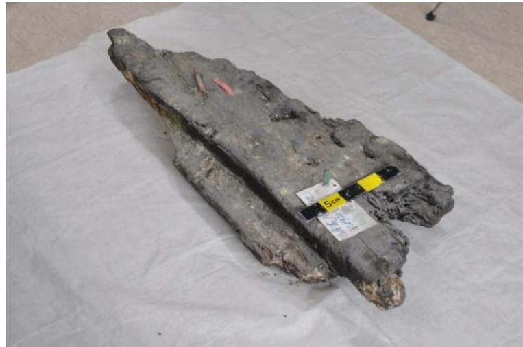
Figure 8-7 Piece of the hull plank SW-82-182 from the Shinan shipwreck, showing its rabbeted seam. Photo by author
