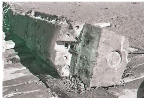
Figure 5-8 Scarf of the keel showing circular holes to place coins and a mirror. Courtesy of Museum of Overseas Communication History
