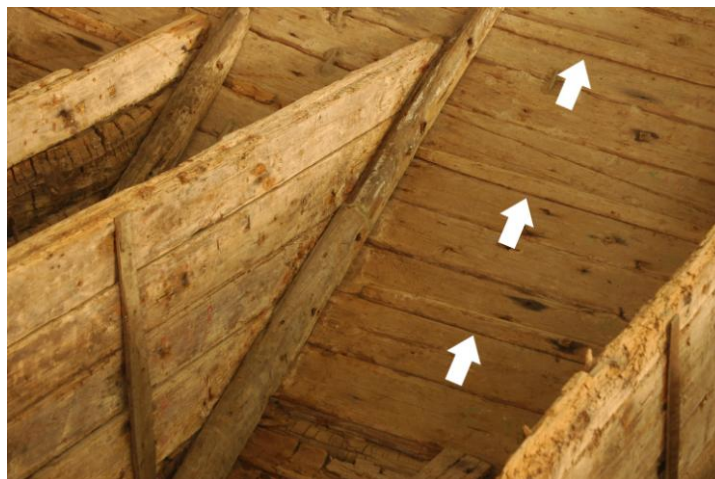
Figure 5-21 Fairing laths sitting on the inside at each clinker step. Photo by author
