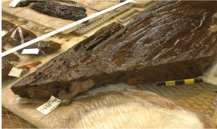
Figure 7-9 Nail holes and degraded nail on the end of the No. 1440 plank. Photo by author
