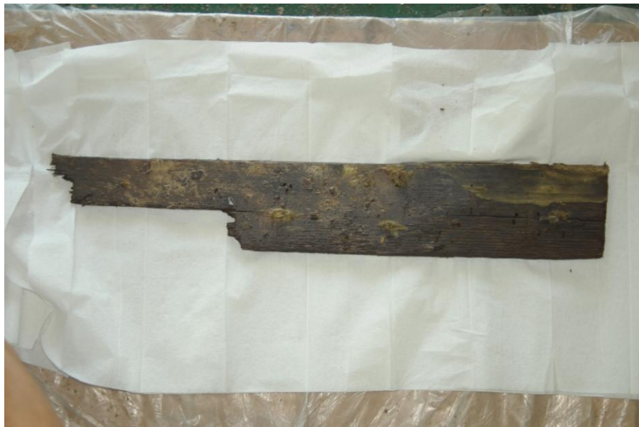
Figure 6-16 Sheathing plank that has been covering the hull. Photo by author
