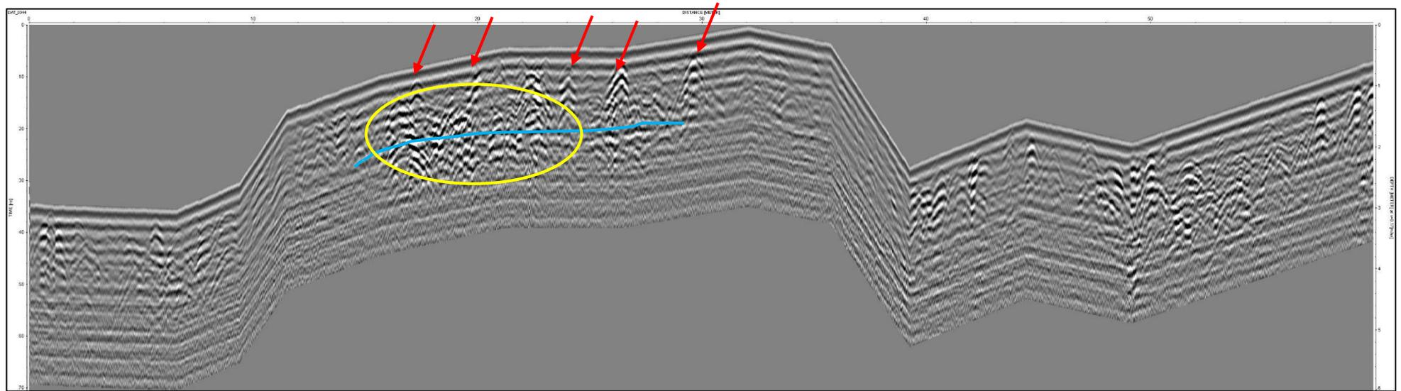
Figure 5.120: GPR Transect 02 Toul Slaeng, note vertical exaggeration. Area of high-amplitude responses (yellow) centre of the mound in combination of hyperbolas (red) and a subsurface surface (blue). Subsurface hyperbolas also present on the periphery.
