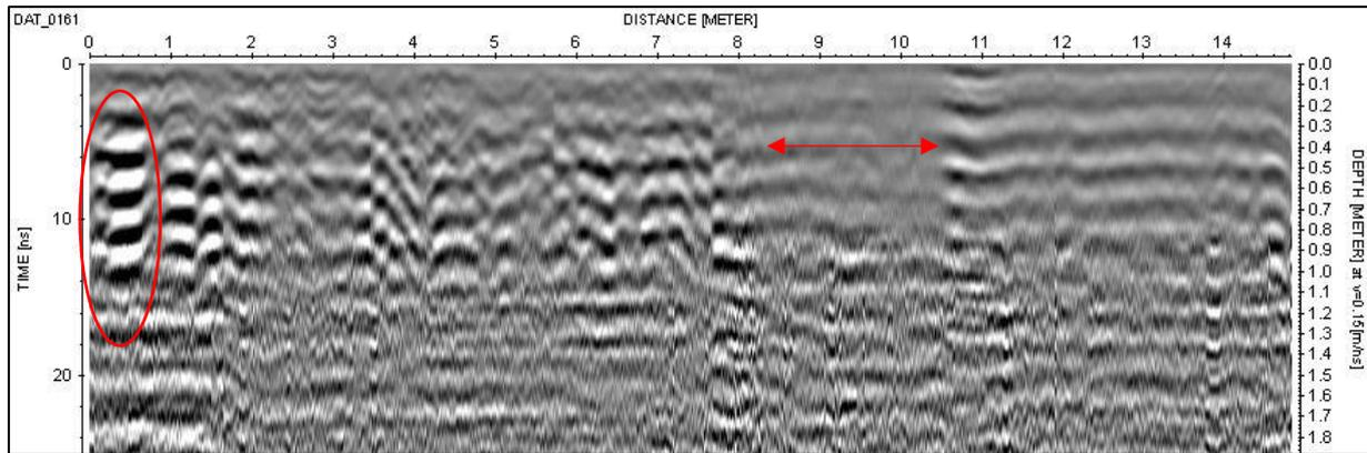
Figure 5.7: GPR line 161 at 0m of Grid 103 at Toul Basan. This line was taken adjacent to the excavation square. The reflection of the square resulting in a line break reflection highlighted by red arrow. Also present is possible buried material causing high-amplitude radar responses (circled).
