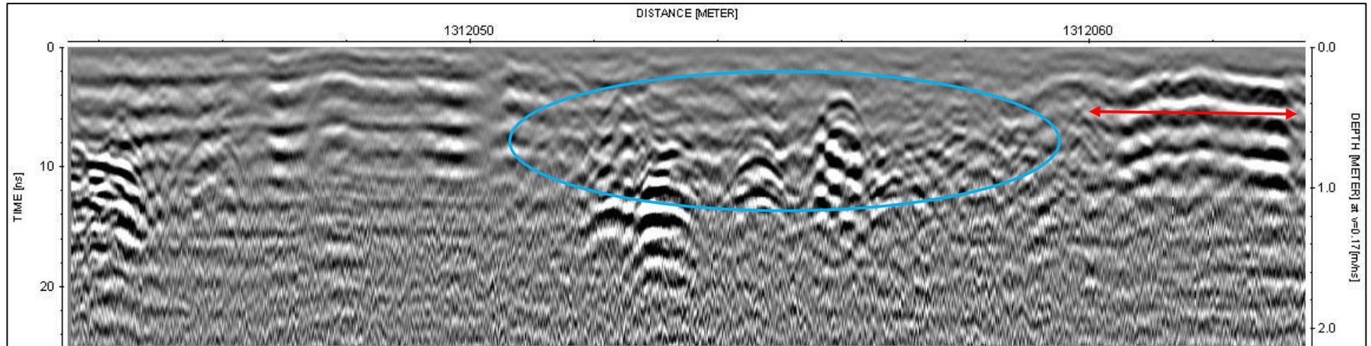
Figure 5.53: Brick factory north GPR line 231 at 9.5m of Grid 05. Note disturbed area with limited high-amplitude radar response in blue and homogenous areas highlighted in red.
