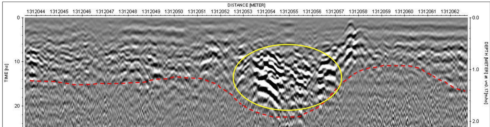
Figure 5.54: Brick factory north GPR line 254 at 20m of Grid 05 red dashed line highlighting the change in topography with ditch which is filled with high-amplitude radar responsive material highlighted in yellow.
