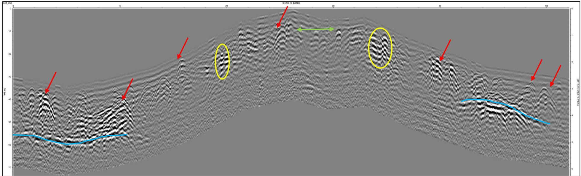
Figure 5.121: GPR Transect 03 Toul Slaeng. Note vertical exaggeration. Subsurface surface off the mound (blue), possible in situ high-amplitude feature (yellow), strata break (green) and hyperbolas (red).
