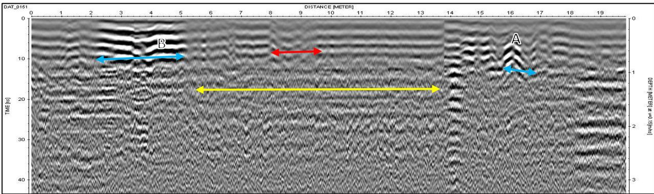
Figure 5.88: GPR line 151 at 11m of Grid 03 Wat Trolaeng Kaeng south, feature A and B are consistent across a series of profiles, and when mapped in Figure 5.89 form a unified shape across the area which corresponds with the magnetometry results. Also present but not represented in the magnetometry is a section break at the centre of the profile (red) and the area of largely homogenous activity (yellow).
