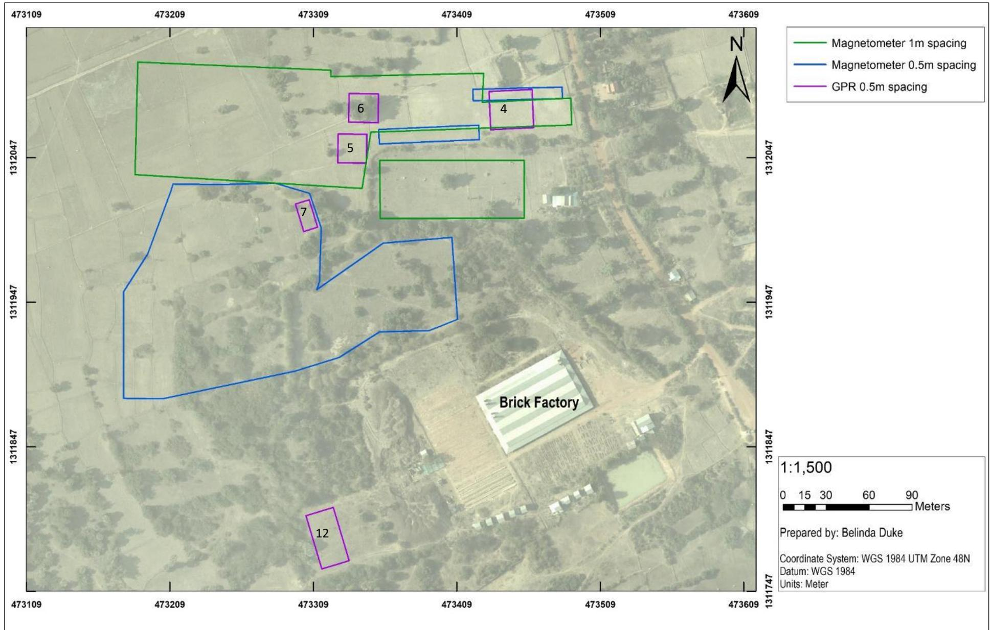
Figure 5.40: Geophysical survey conducted at Brick Factory North using a single and dual sensor magnetometer and 500mHz GPR antenna, grids numbered.
