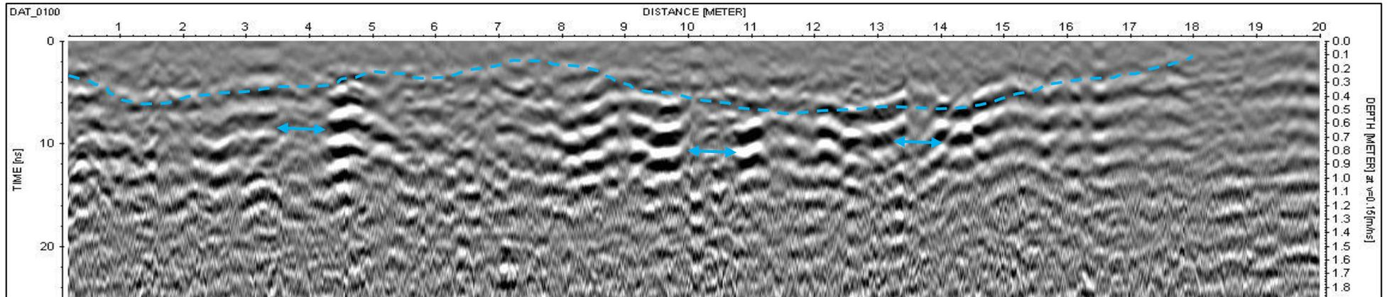
Figure 5.85: GPR line 100 at 7m of Grid 02 Wat Talaeng Kaeng south, profile of a GPR showing line breaks (blue arrows) like Grid 01. Section breaks are below the plough line (highlighted with blue dashed line).
