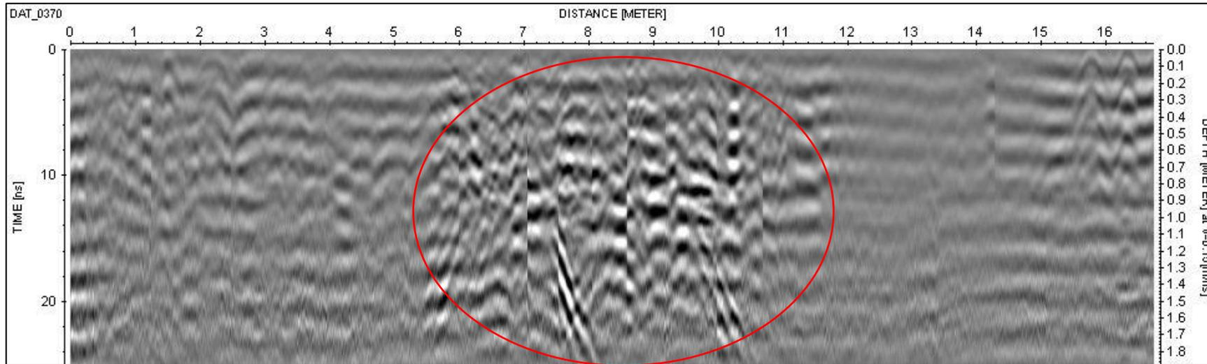
Figure 5.20: GPR line 370 a 0m of Grid 110 at Prasat Preah Theat Baray. Note disturbed area centre.
