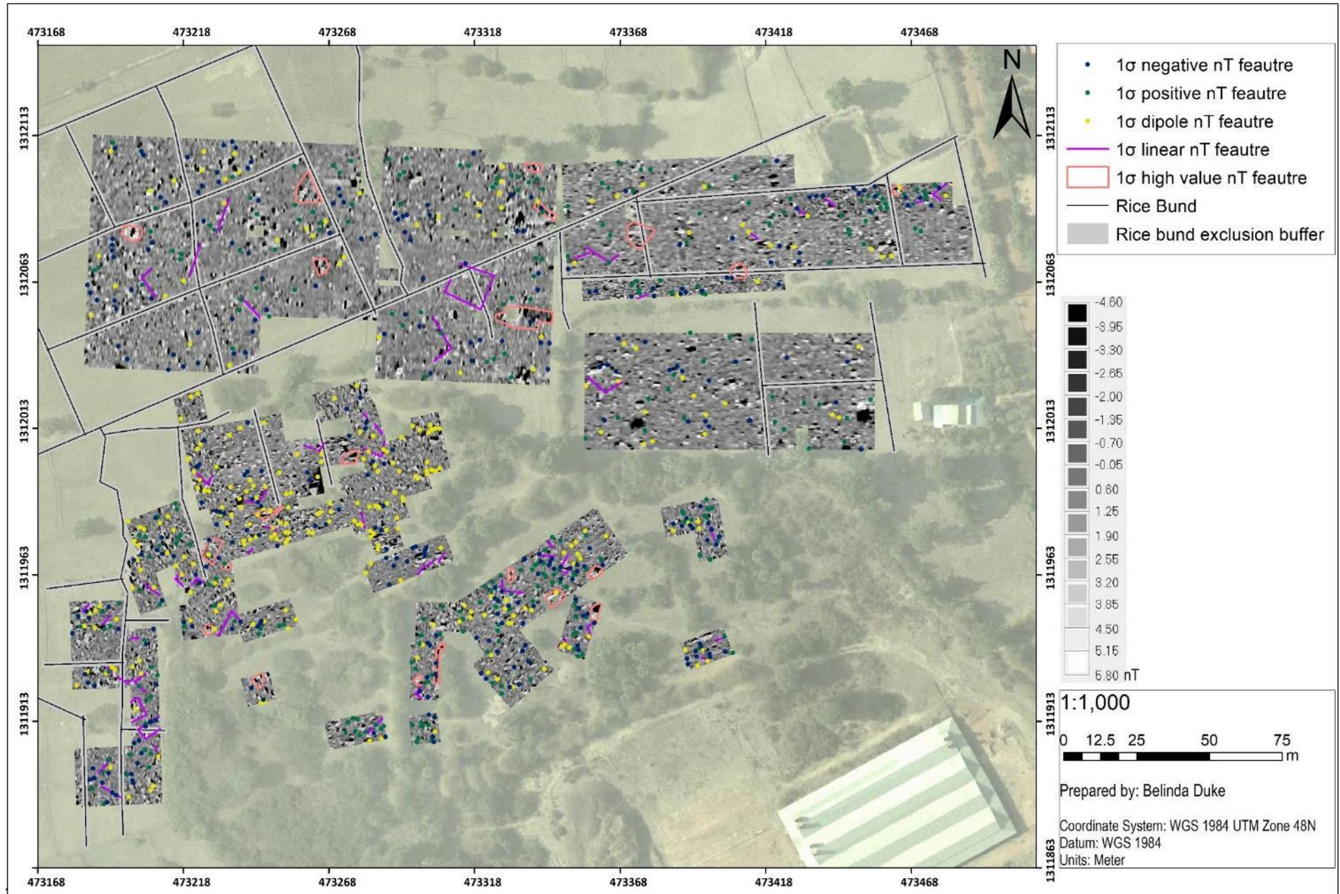
Figure 5.43: Brick factory north magnetometer survey conducted in February and December 2018. Gridding either in 20x20m or 10x10m squares magnetometer results One standard deviation (-4.6 – 5.8nT) from the mean.
