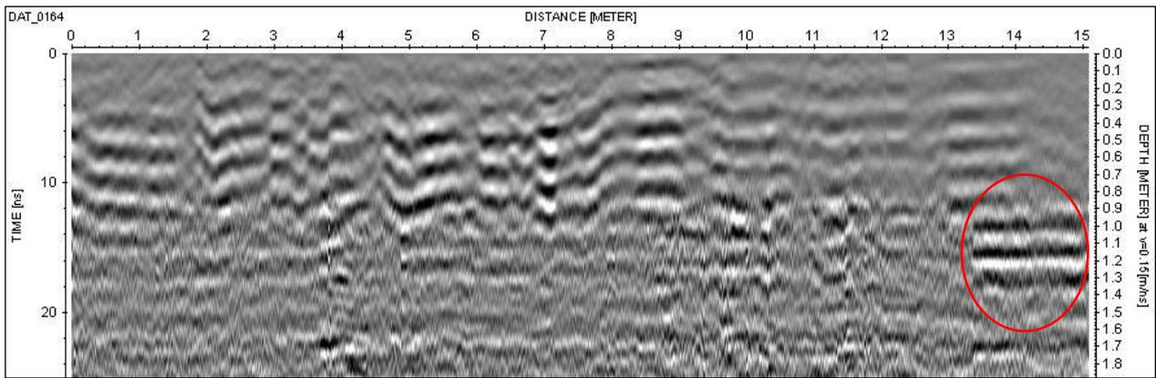
Figure 5.8: GPR line 164 at 2m of Grid 103 at Toul Basan. GPR feature one depth below surface, highlighted in red are present. However, these are likely the result of instrument reflection error.
