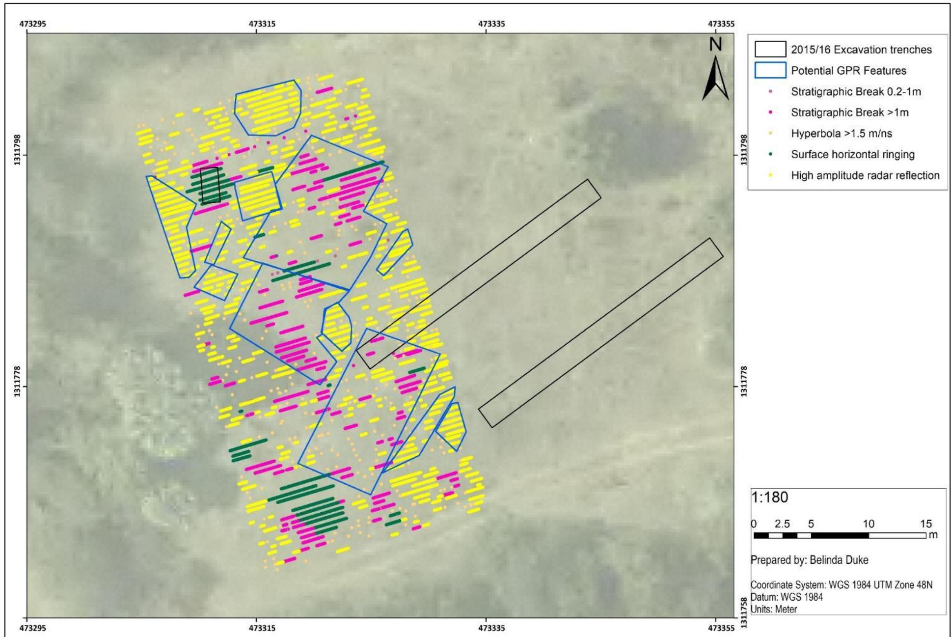
Figure 5.71: GPR Grid 12 sub-surface features. Note high volume of high-amplitude radar reflections present here.
