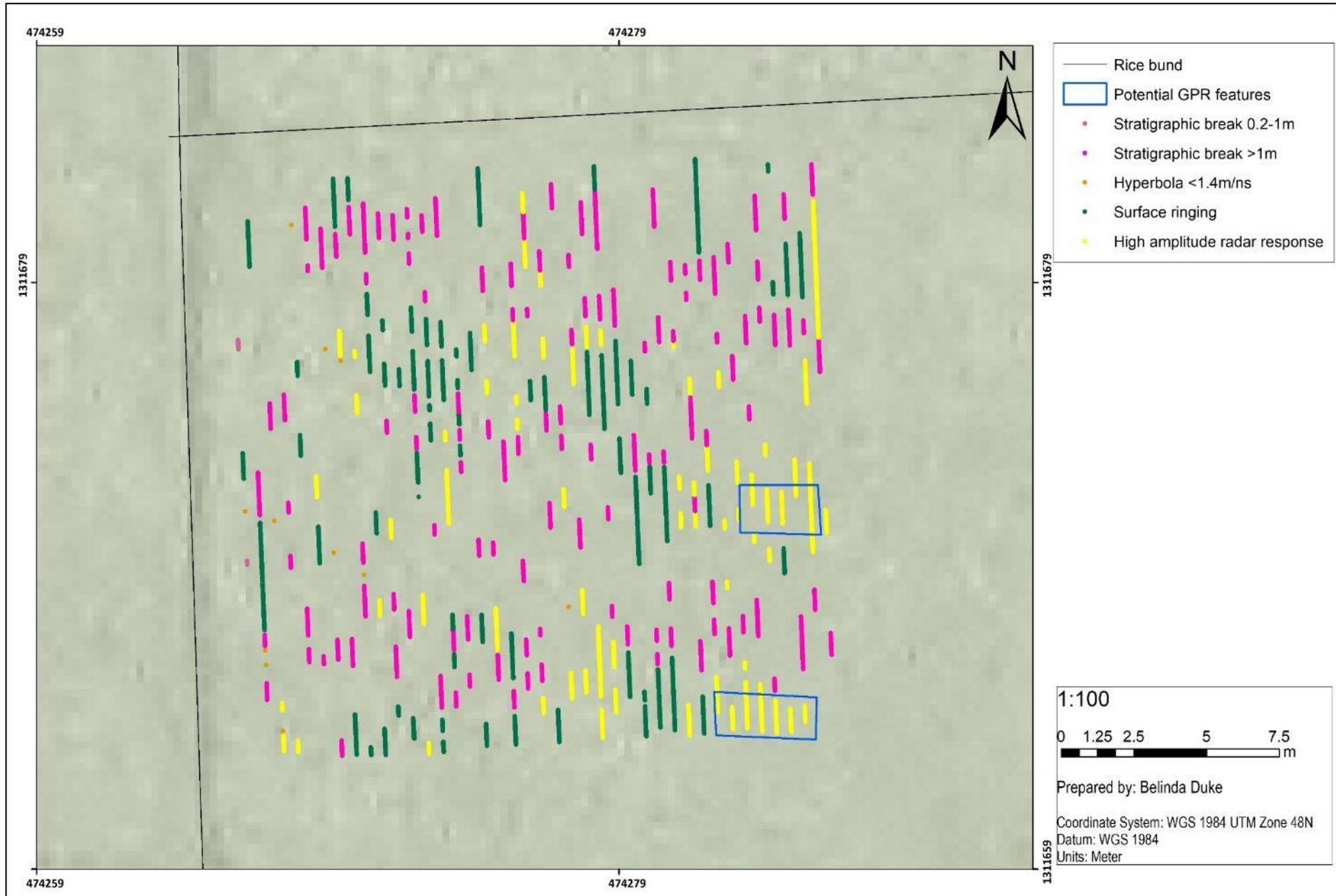
Figure 5.86: GPR Grid 02 Wat Trolaeng Kaeng south. Area contains a high volume of section breaks, like Grid 01. Likely due to ongoing farming activities.
