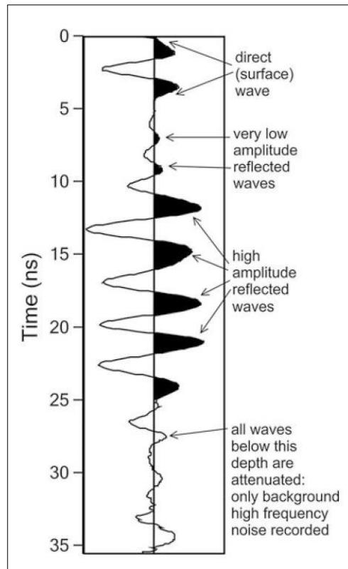
Figure 3.8: A single GPR trace with changes in amplitude and attenuation over the recorded time-window (from Conyers 2018:21).
