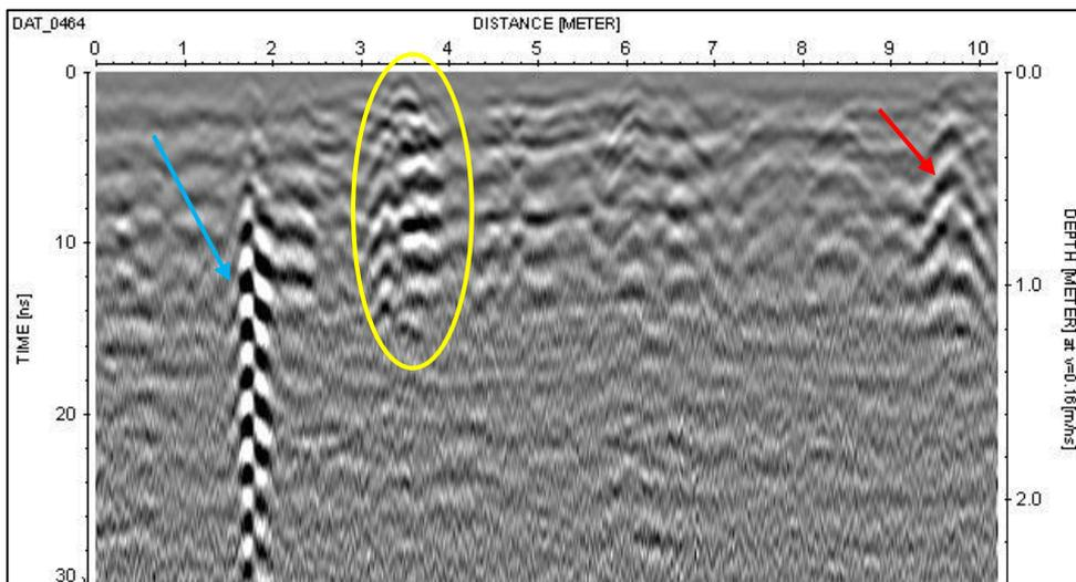
Figure 5.100: GPR line 464 at 4.4m of Grid 10 Wat Tralaeng Kaeng south. High-amplitude vertical ringing (blue), high-amplitude radar response (yellow) high-amplitude hyperbola (red).
