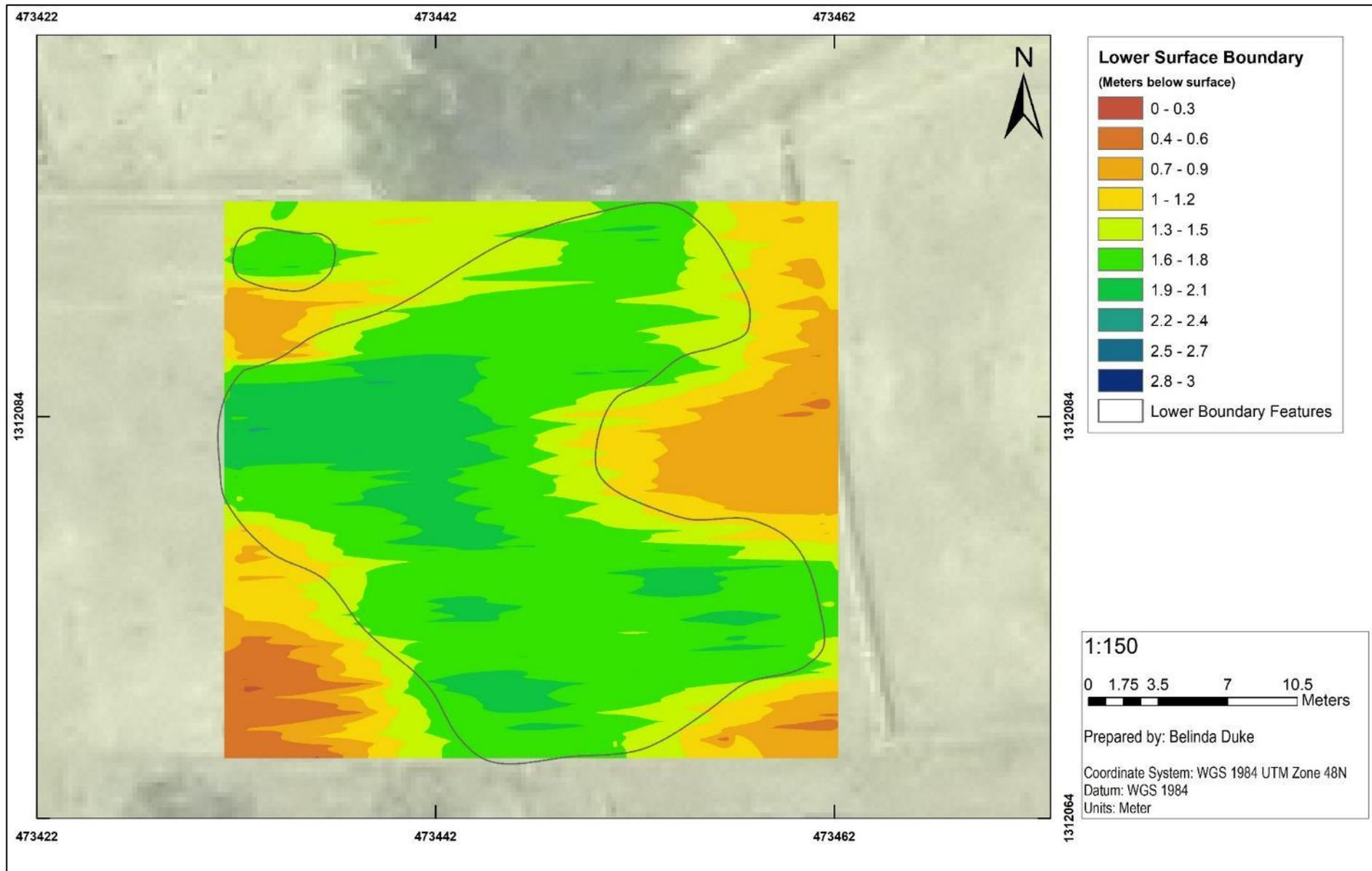
Figure 5.49: Brick factory north GPR Grid 04 subsurface topography mapped from depth of lower surface boundary which is the surface transition from middle area of intensified discrete high-amplitude features to lower level undisturbed strata. Two large pits and two medium sized pits identified. Possibly a large single feature, however surface disturbance which caused compacted strata from heavy vehicles may be impacting this.
