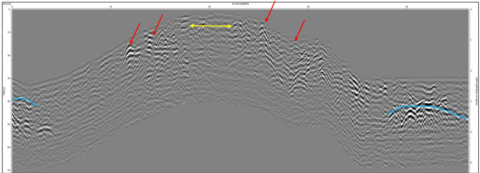
Figure 5.119: GPR Transect 01 Toul Slaeng. Note vertical exaggeration. Subsurface surface (Blue), centre of the mound has a higher number of hyperbolas (red) and a strata break at the centre (yellow).
