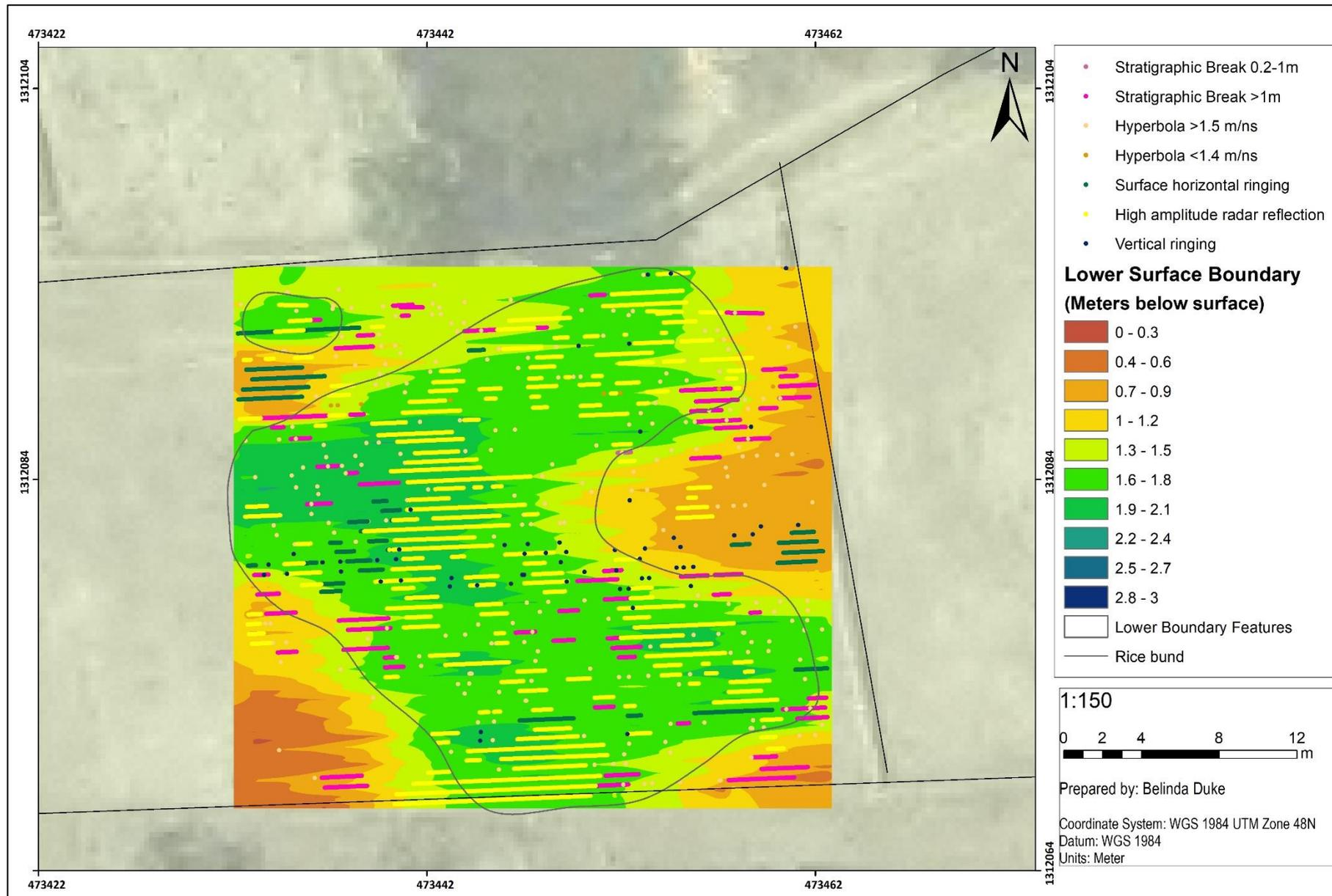
Figure 5.51: Brick factory north GPR Grid 04 with features overlaid lower surface boundary. Note the majority of the high-amplitude radar response are contained within the lower areas of the feature.
