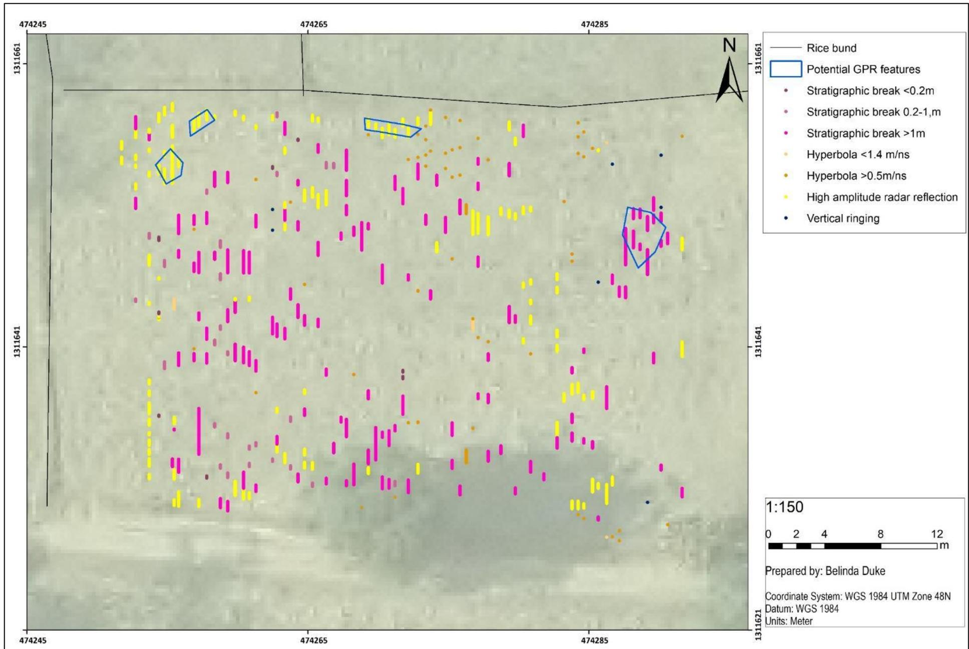
Figure 5.83: GPR Grid 01 Wat Trolaeng Kaeng South. Radar response reflects homogenous nature of the sediment with high prevalence of section breaks. Features identified are likely modern.
