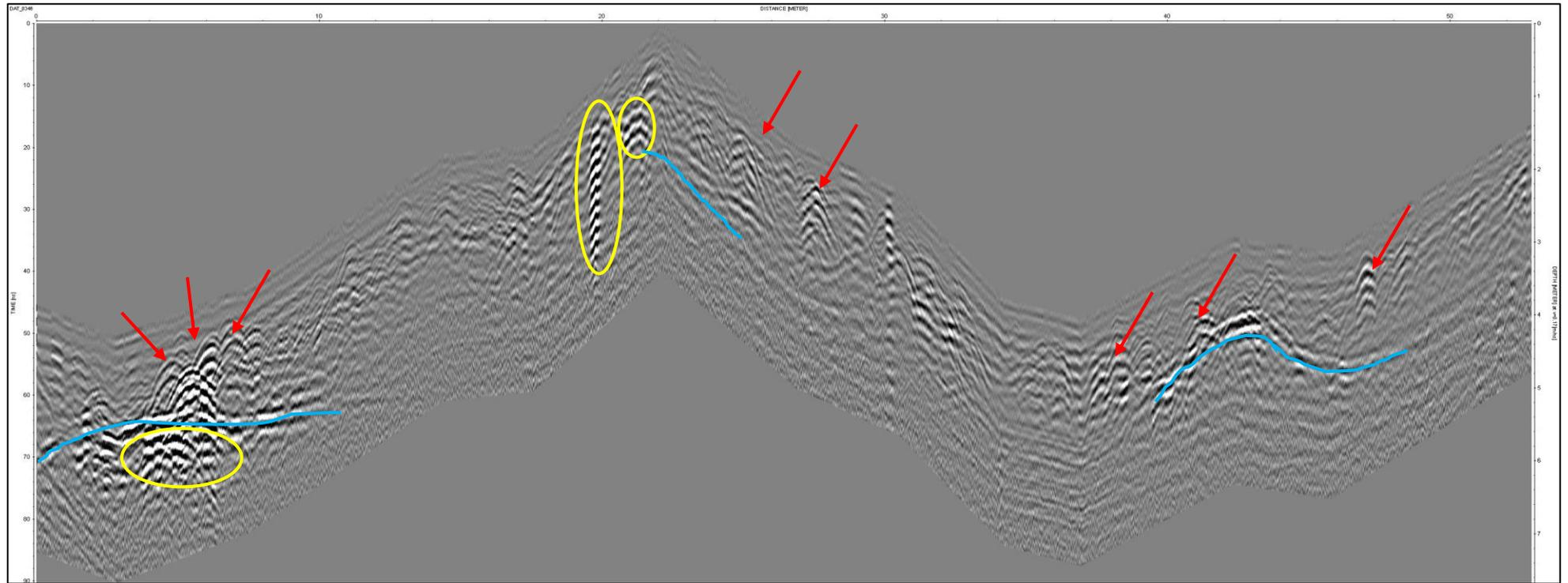
Figure 5.122: GPR Transect 04 Toul Slaeng. Note vertical exaggeration. Subsurface surface (blue), possibility in situ features (yellow), high-amplitude hyperbolas (red) and high-amplitude radar response under (yellow) buried under the surface.
