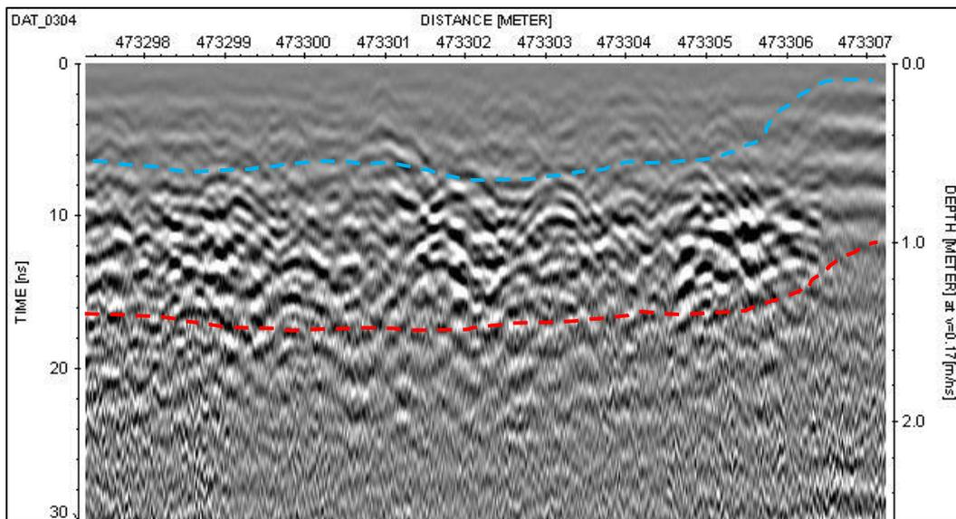
Figure 5.60: Brick factory north GPR line 304 at 1.5m of grid 07. Transition from homogenous strata with little disturbance to area of multiple high-amplitude features (blue) and transition from high-amplitude features to lower level undisturbed strata (red). This defined layer is consistent across Grid 07.
