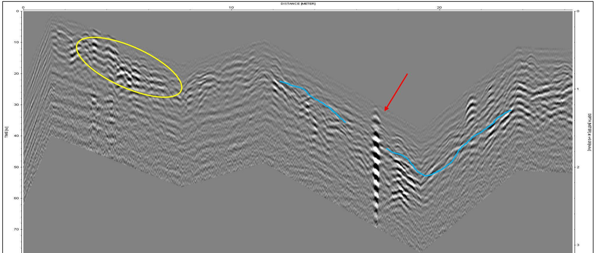
Figure 5.115: GPR Transect 03 Toul Tatob. Note exaggerated vertical axis. In situ feature (yellow), high-amplitude vertical ringing (red) and sub surface layer (blue).
