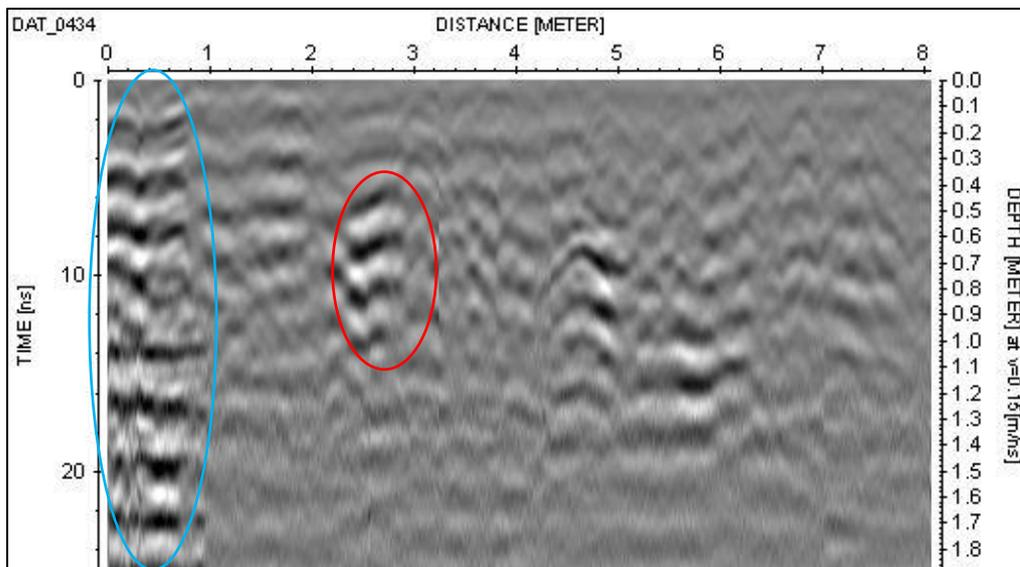
Figure 5.27: GPR line 434 at 11m of Grid 112 at Prasat Preah Theat Baray. Note high-amplitude radar reflections in red and surface ringing to the left in blue.
