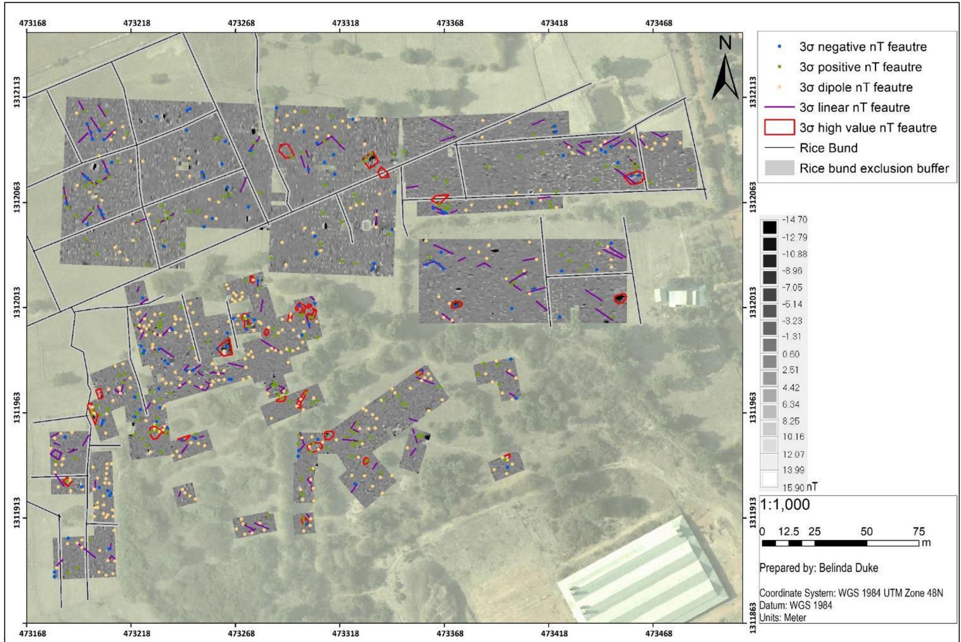
Figure 5.41: Brick factory north magnetometer survey conducted in February and December 2018. Gridding either in 20x20m or 10x10m squares magnetometer results presented with the nT range three standard deviations (-14.7-15.9 nT) from the mean.
