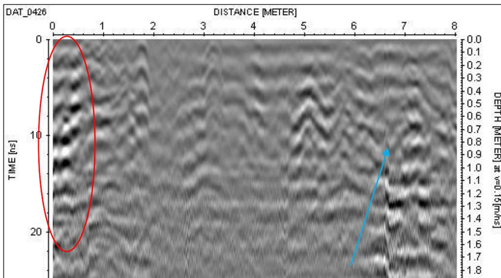
Figure 5.26: GPR line 426 at 11m of Grid 112 at Prasat Preah Theat Baray. Area of high-amplitude reflection on the left (red) with area of what appears to be disturbed sediment to the right (blue).
