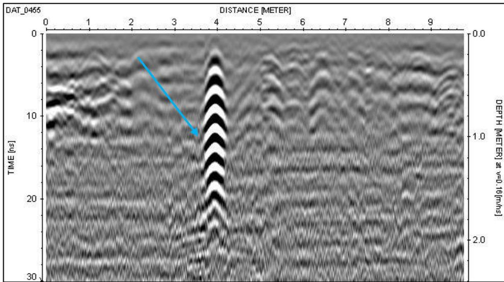
Figure 5.99: GPR line 455 at 0m of Grid 10 Wat Tralaeng Kaeng south. High-amplitude vertical ringing (blue), similar to other survey grids for this area.
