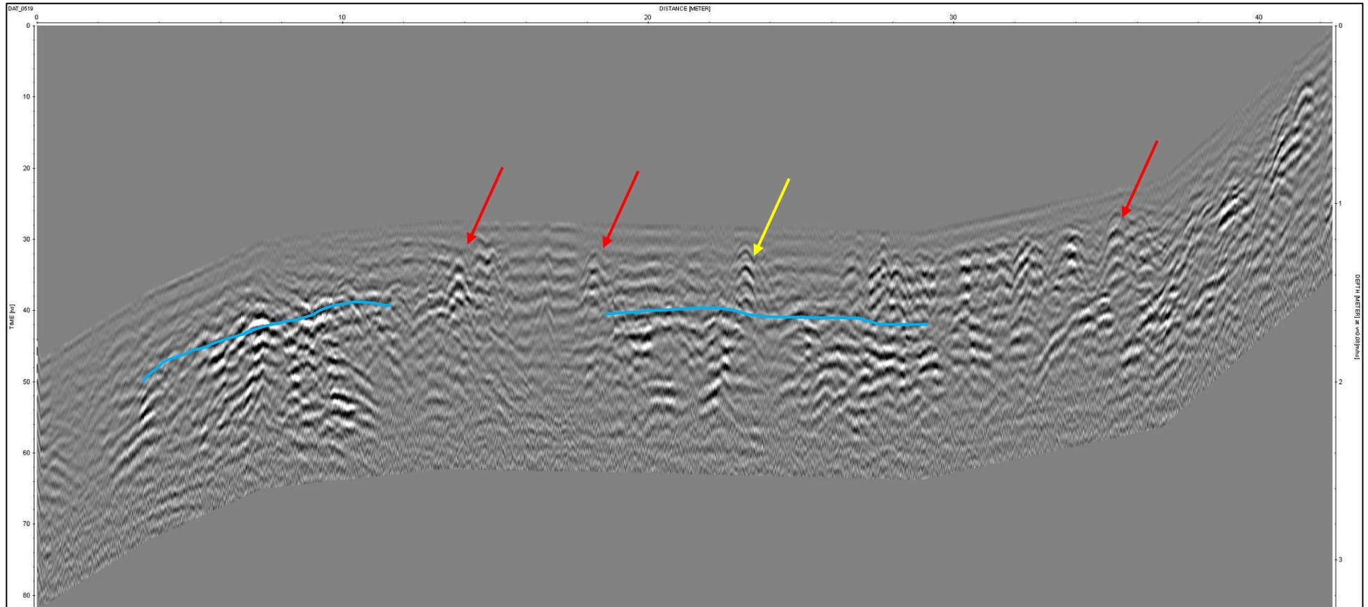
Figure 5.114: GPR Transect 02 Toul Tatob. Note vertical exaggeration. Buried surface (blue), hyperbola (red). The hyperbola indicated by the yellow arrow is likely the brick found in section in Figure 5.117.
