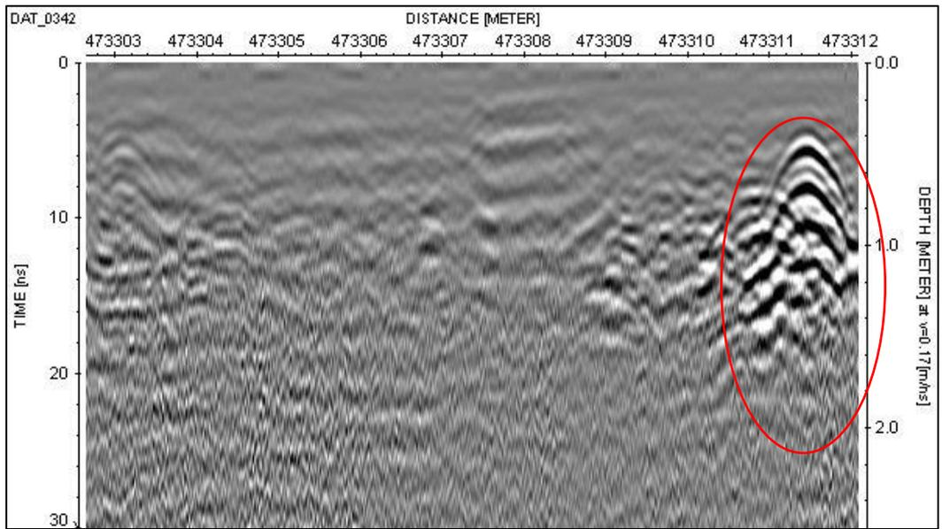
Figure 5.62: Brick factory north GPR line 342 at 20m of Grid 07. Last line in the profile with high-amplitude features and surface horizontal ringing.
