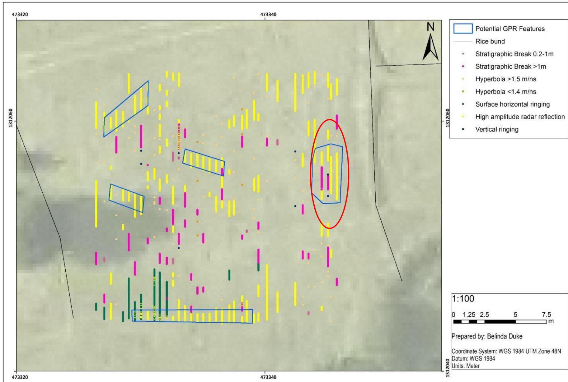
Figure 5.55: Brick factory north GPR Grid 05 sub-surface GPR features. Area highlighted in red corresponds with pit features highlighted in Figure 5.54.
