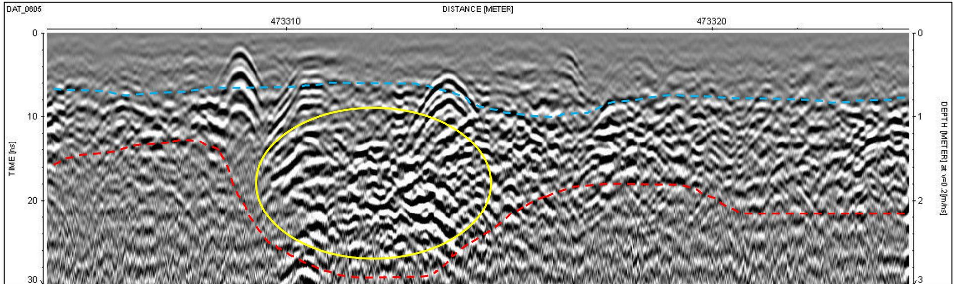
Figure 5.68: South of the brick factory GPR line 605 at 39m of Grid 12. The last line in the survey grid, highlighted in blue the upper sediment horizon and lower in red. Note in yellow a pit filled with high-amplitude radar responses. Pit may be comparable to that found during excavation in Figure 5.65.
