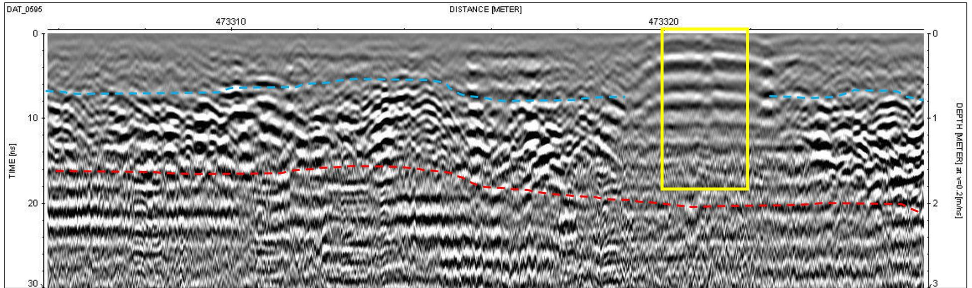
Figure 5.67: South of the brick factory GPR line 595 at 34m of Grid 12. Highlighted excavation trench 1501 in yellow represented as a stratum break, upper surface horizon in blue and lower surface horizon in yellow. Archaeological deposit here 1.5-2m deep. Comparable to excavation section drawing in Figure 5.66 view south.
