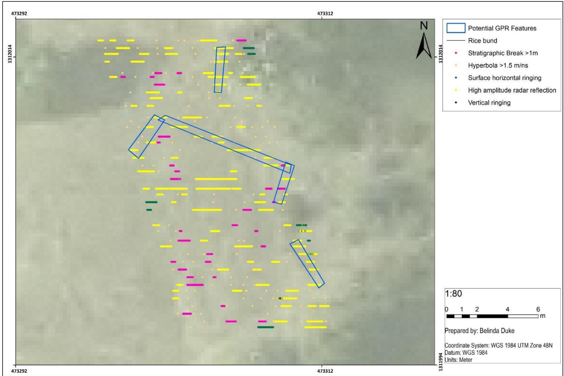
Figure 5.63: Brick factory north GPR Grid 07 with proposed subsurface features.
