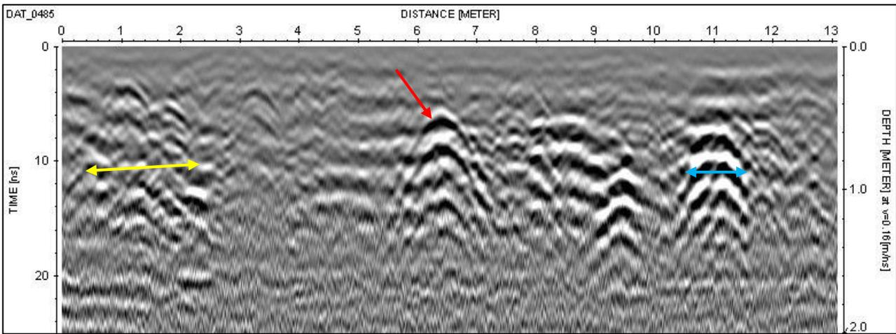
Figure 5.103: GPR line 485 at 4.5m of Grid 11 Wat Tralaeng Kaeng South. In-situ high-amplitude response (blue). Also present high-amplitude hyperbola (red) and area of disturbance (yellow), also seen in profile of Figure 5.104, occurring over almost all profiles which corresponds with a large features mapped in Figure 5.105.
