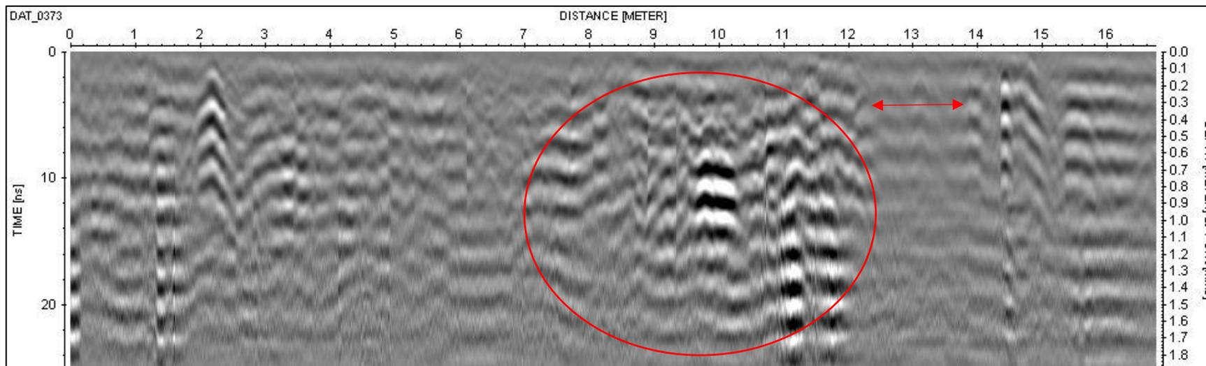
Figure 5.21: GPR line 373 at 1.5m of Grid 110 at Prasat Preah Theat Baray with area of archaeological features centre and section break right which is consistently found across all profiles.
