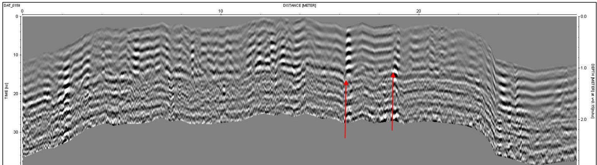
Figure 5.12: Toul Basan transect four running north to east at Toul Basan. Note areas of vertical ringing caused by an object in the near subsurface.
