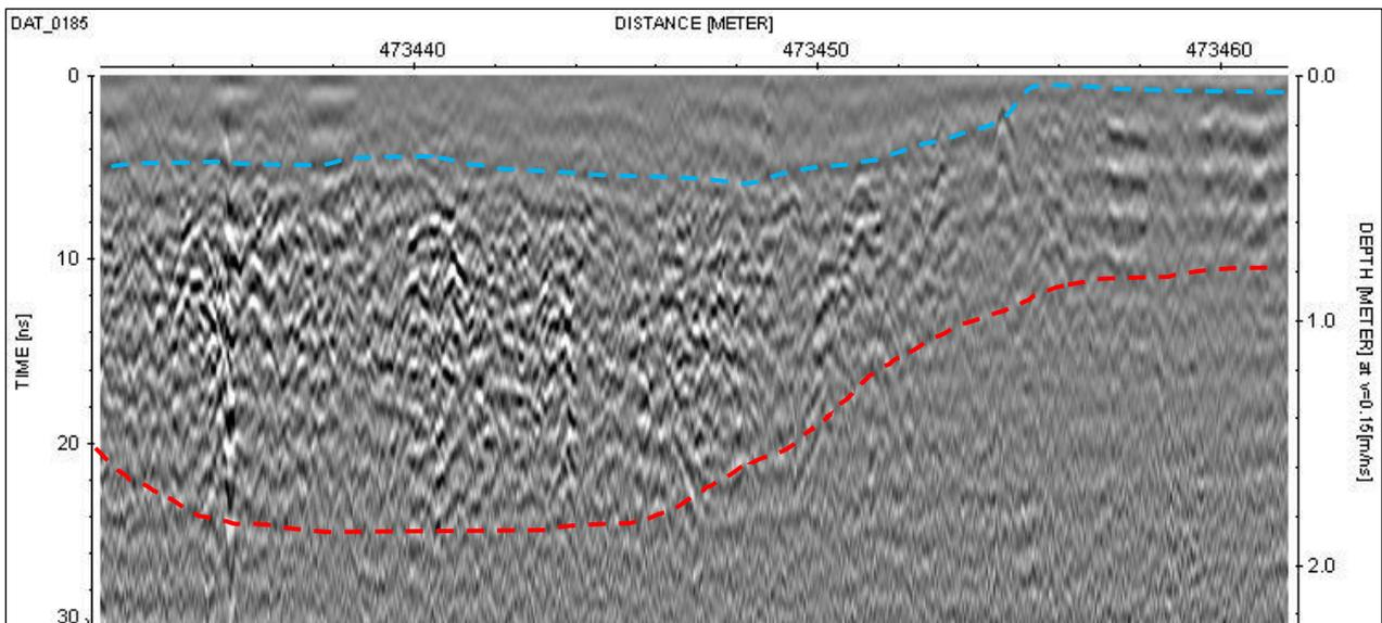
Figure 5.47: GPR Line 26 at 12.5m of Grid04 at brick factory north showing a layer of high-amplitude radar reflections with an upper boundary, in blue, transitioning to homogenous sediment and a lower boundary, in red, transitioning to undisturbed strata at the lower boundary.
