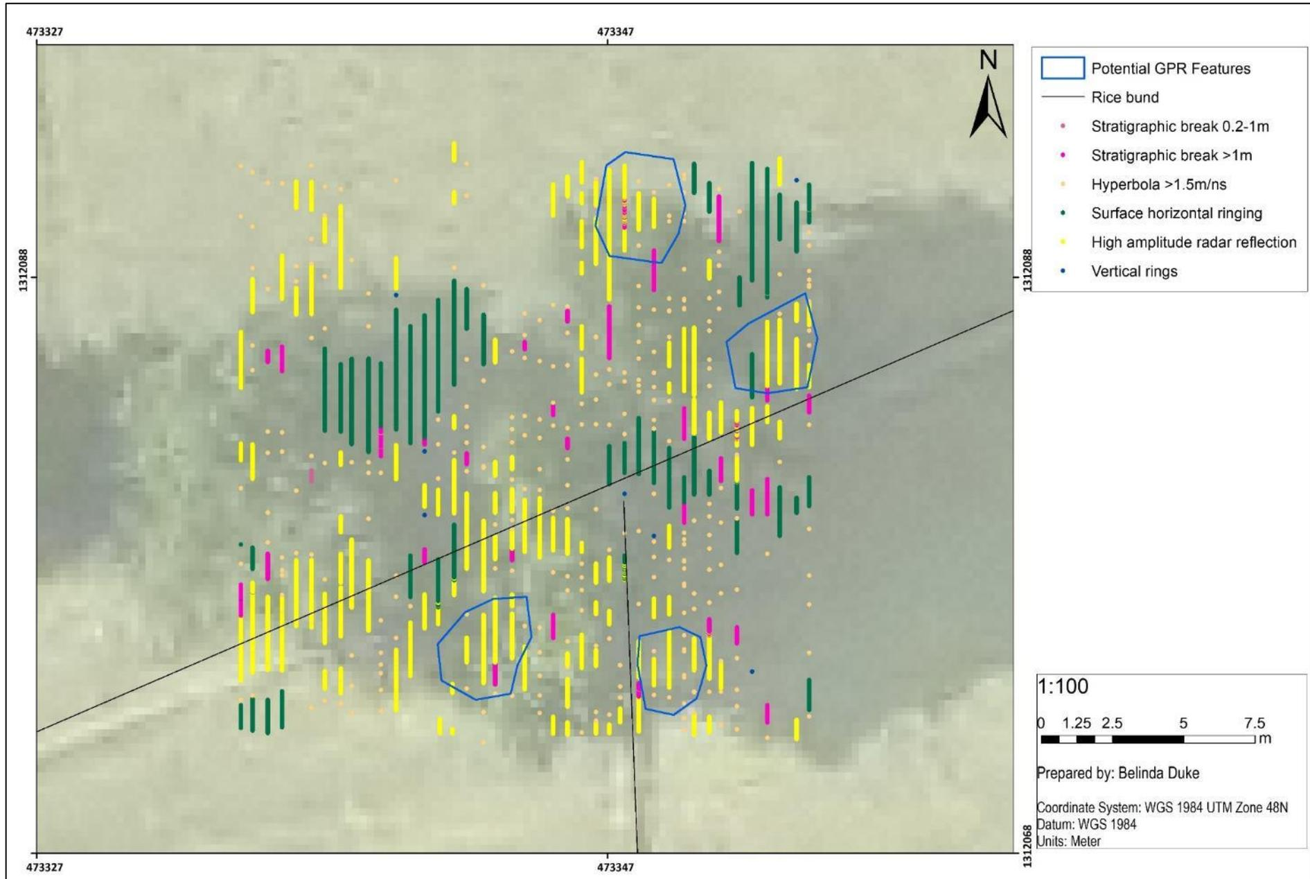
Figure 5.57: Brick factory north GPR Grid 06 with sub-surface GPR features.
