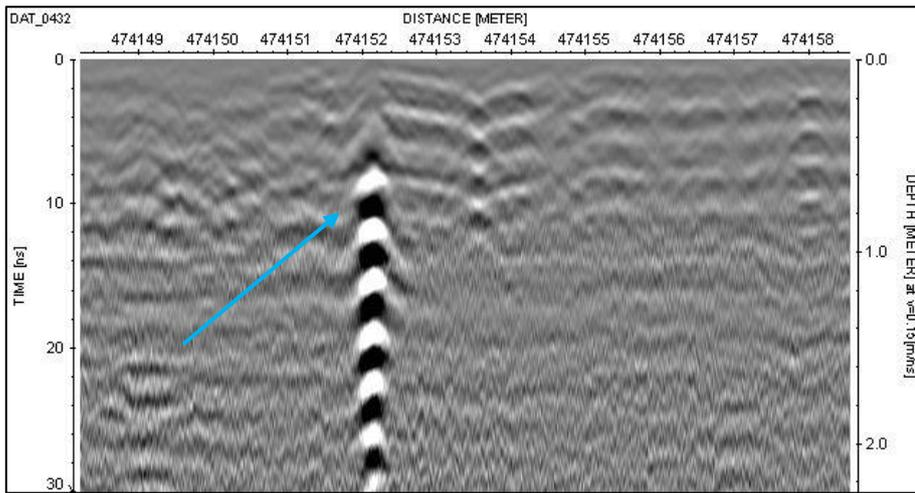
Figure 5.95: GPR line 432 at 10m of Grid 09 Wat Tralaeng Kaeng south. High-amplitude vertical ringing (blue)
