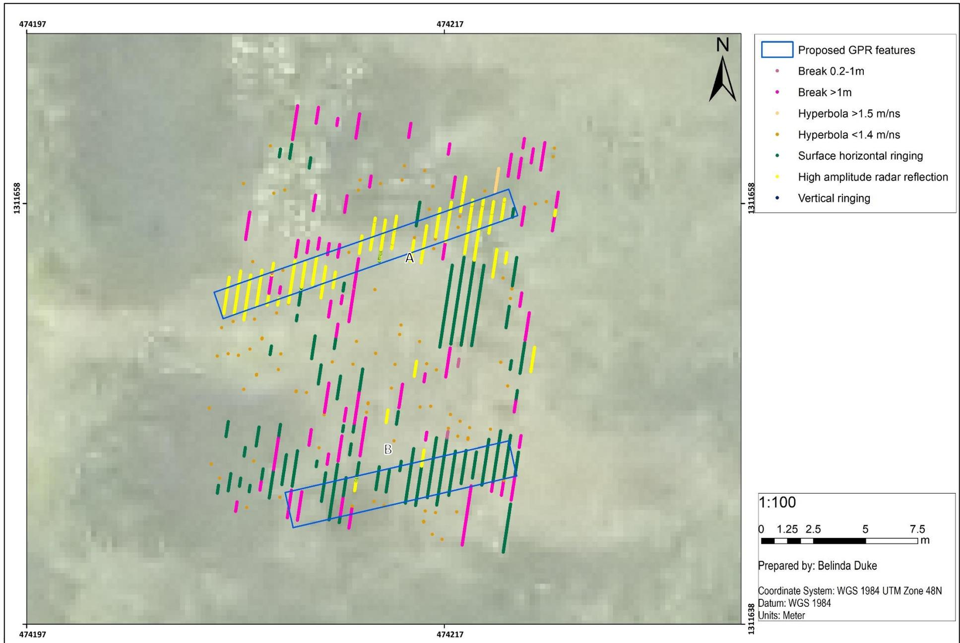
Figure 5.89: GPR Grid 03 Wat Tralaeng Kaeng south, features A and B corresponding with features in Figure 5.88. These distinct features were also found in the magnetometer results.
