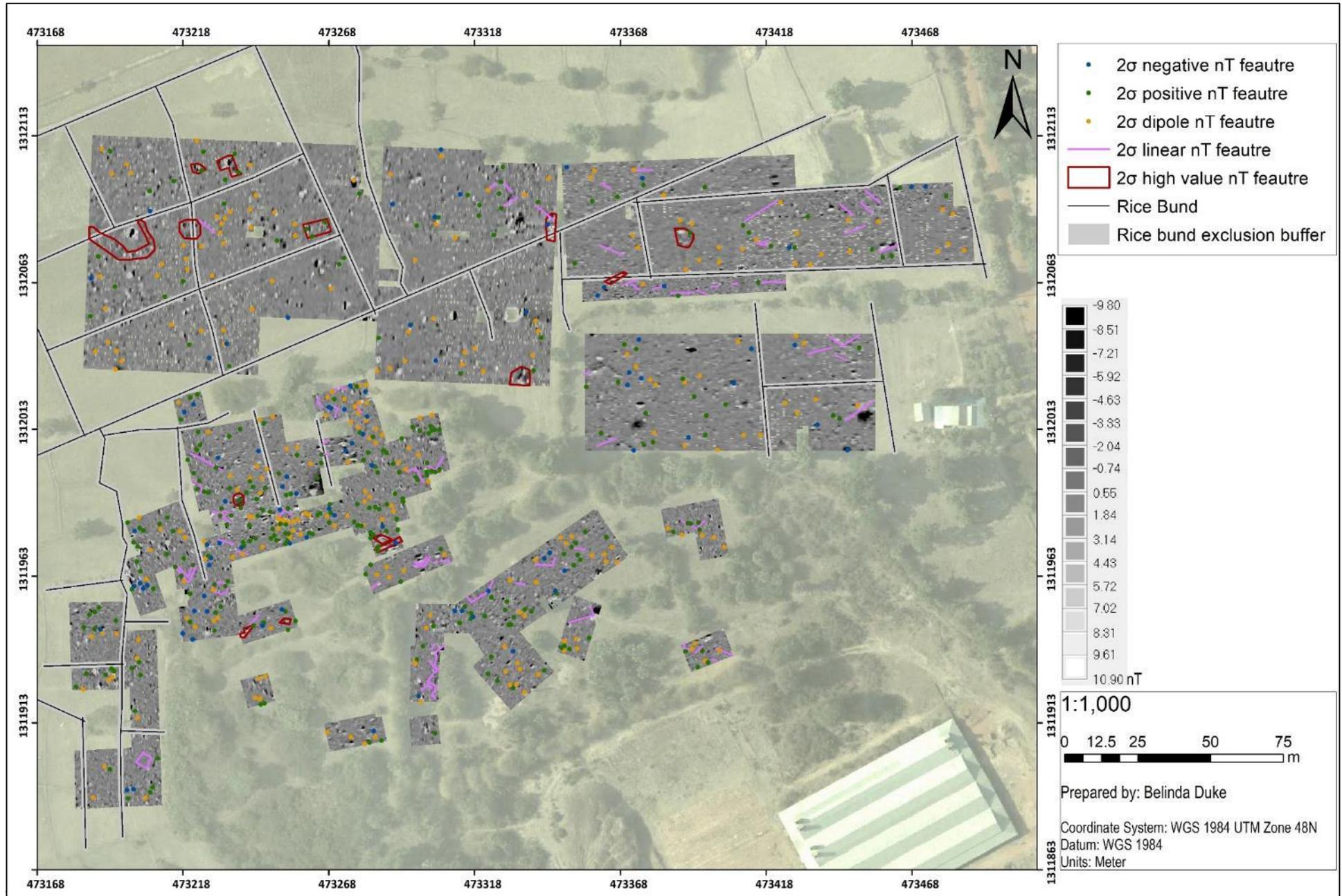
Figure 5.42: Brick factory north magnetometer survey conducted in February and December 2018. Gridding either in 20x20m or 10x10m squares magnetometer results two standard deviation (-9.8- 10.9 nT) from the mean.
