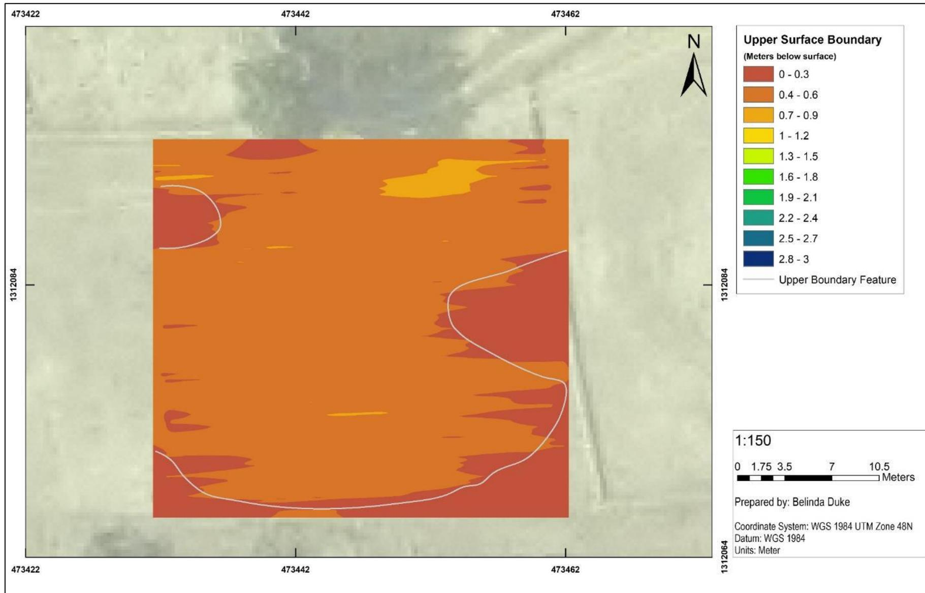
Figure 5.48: Brick factory north GPR Grid 04 subsurface topography mapped from depth of upper surface boundary which is the surface transition from upper homogenous strata with little disturbance to middle area of intensified discrete high-amplitude features. Areas not in depression were compacted strata which the radar pulsed did not penetrate. Compaction may be due to surface disturbance caused by heavy vehicles and soil disturbance.
