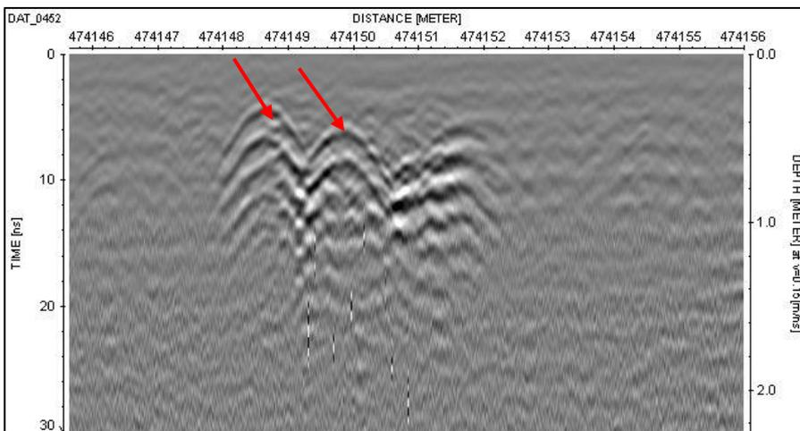
Figure 5.96: GPR line 452 at 19.4m of Grid 09 Wat Tralaeng Kaeng South. High-amplitude hyperbola (red).
