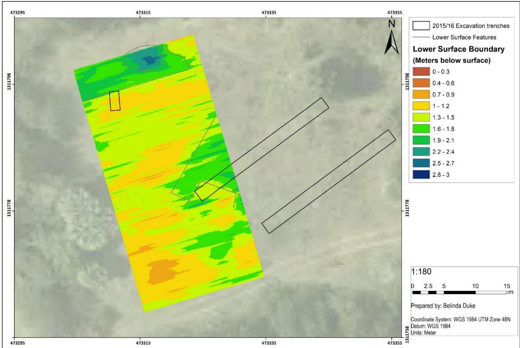
Figure 5.70: GPR Grid 12 south of the brick factory sub-surface topographic reconstruction of the lower surface boundary.
