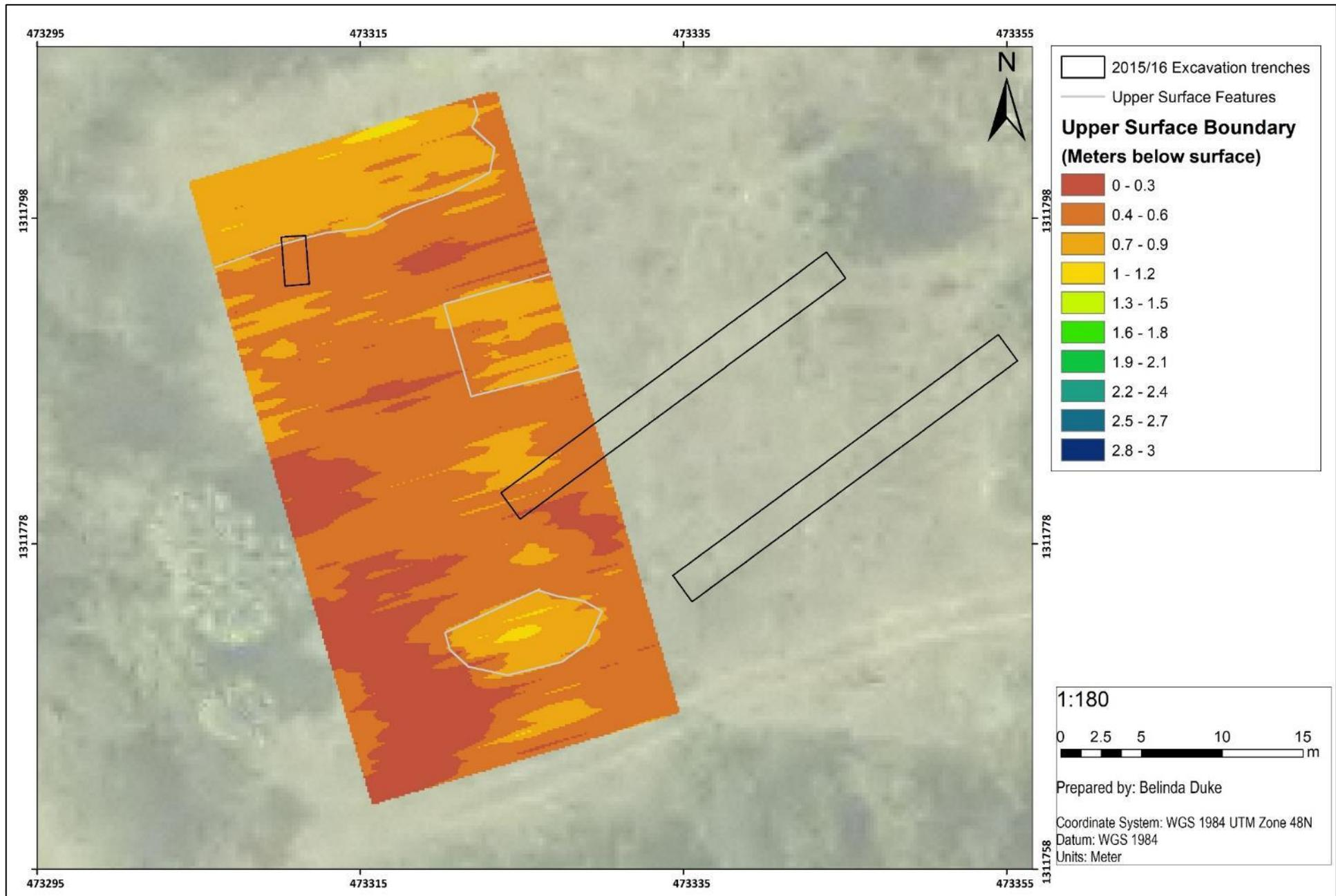
Figure 5.69: GPR Grid 12 south of the brick factory sub-surface topographic reconstruction of the upper surface boundary identified within the profiles.
