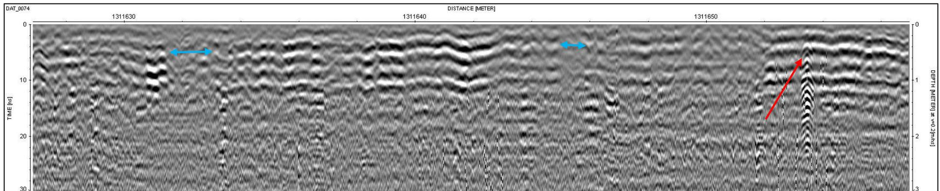
Figure 5.82: GPR line 74 at 34.5m of Grid 01, Wat Tralaeng Kaeng South. Section breaks found across area and are likely the result of farming activity (in blue). Vertical ringing highlighted in red likely the result of metal in the subsurface.
