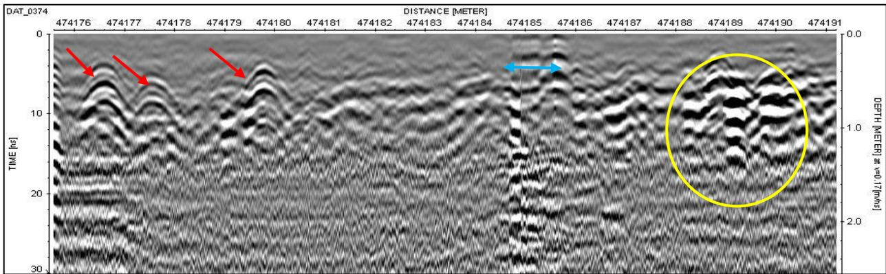
Figure 5.91: GPR line 374 at 13.5m of Grid 08 Wat Trolaeng Kaeng south. Area contains a high volume of hyperbola (red) and surface ringing (blue). High-amplitude radar reflections (yellow) also present.
