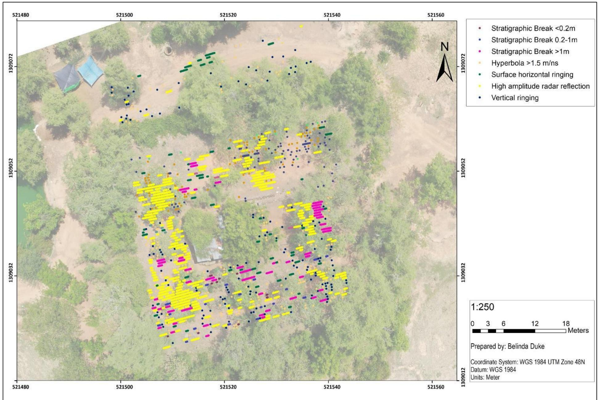
Figure 5.31: Prasat Preah Theat Baray ground-penetrating radar subsurface features.
