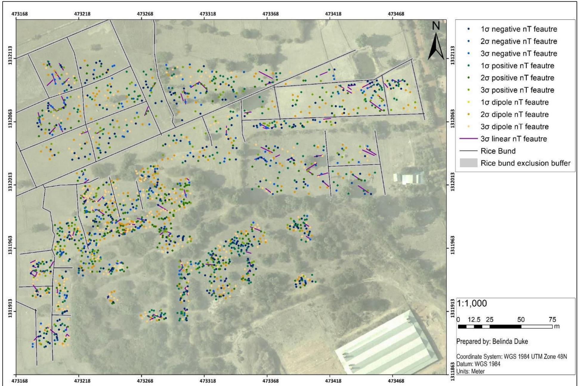
Figure 5.44: Brick factory north distribution of all identified magnetometer features at three, two and one standard deviation combines all the identified features from the three data mapping ranges. Boundary between two areas when examining the volume of points. The top half had a one-meter line spacing while the bottom has a half meter line spacing.
