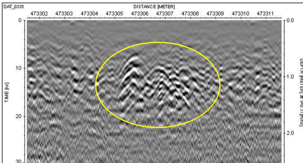
Figure 5.61: Brick factory north GPR line 335 at 17.5m of Grid 07, high-amplitude hyperbola (highlighted in yellow) likely the result of archaeological material. Deep enough in the profile to be unrelated to surface contamination.
