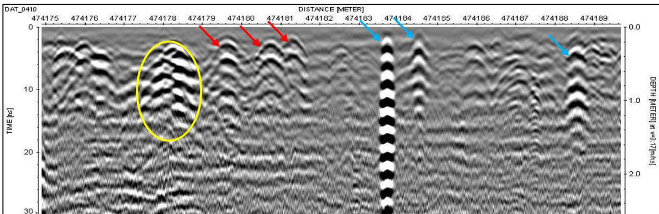
Figure 5.92: GPR line 410 at 30m of Grid 08 Wat Trolaeng Kaeng south. Continuation of the hyperbola (red) but also in this profile is high-amplitude vertical ringing (blue) and thing but in yellow.
