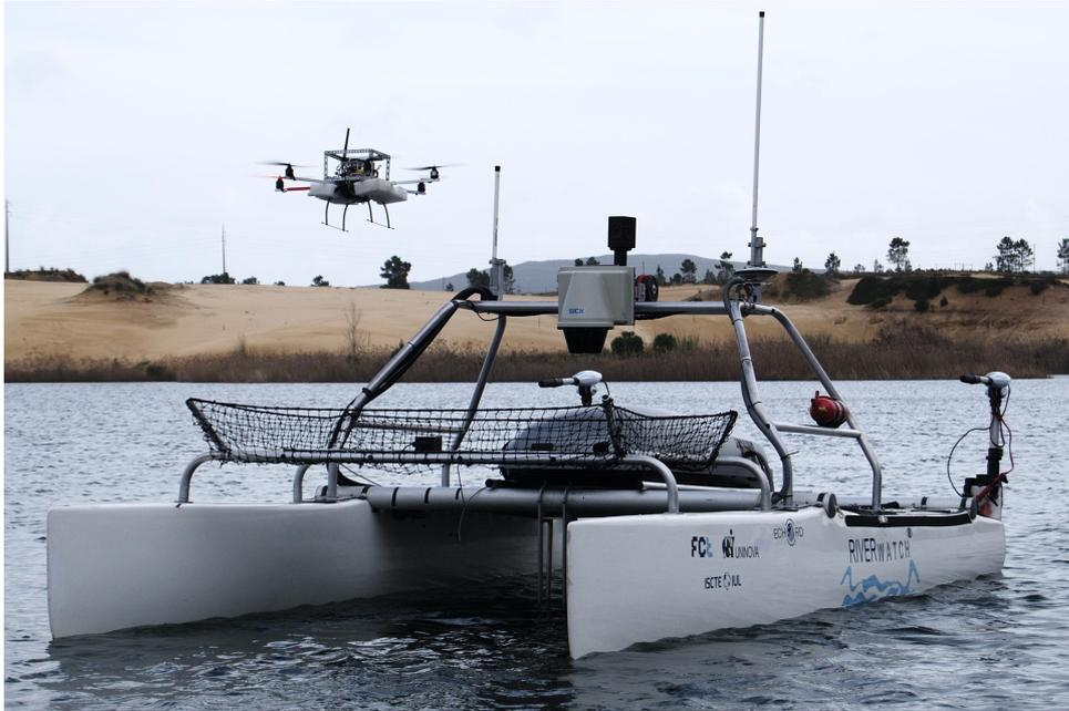
Figure 1.4: Riverwatch Autonomous Surface Vessel with hovering Unmanned Aerial Vehicle [Pinto et al., 2014a]. Image ©2014 IEEE .
