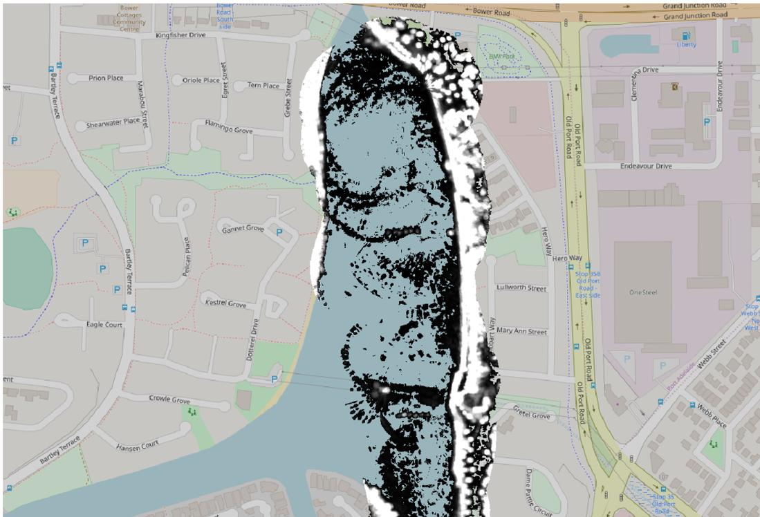
Figure 5.8: RAdio Direction And Ranging (RADAR) map of West Lakes. White areas are accumulated strong RADAR returns. Backing image ©OpenStreetMap contributors.
