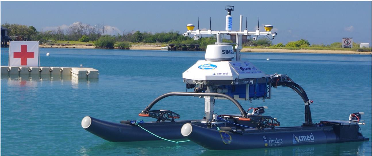
Figure 1.5: TopCat Autonomous Surface Vessel at Maritime RobotX 2016. Cropped from original image by Andrew Webb.
