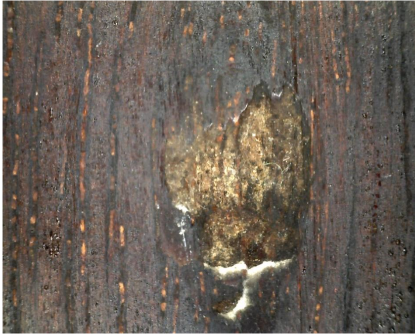
Figure 33. Woomera QE261.1: Possible impact mark or wood defect filled with resin.
