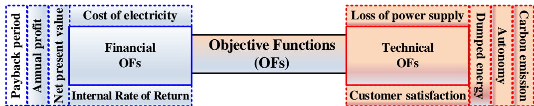
Figure 2-4. Applicable objective functions for optimal sizing of PV-battery system in grid-connected residential sectors.
