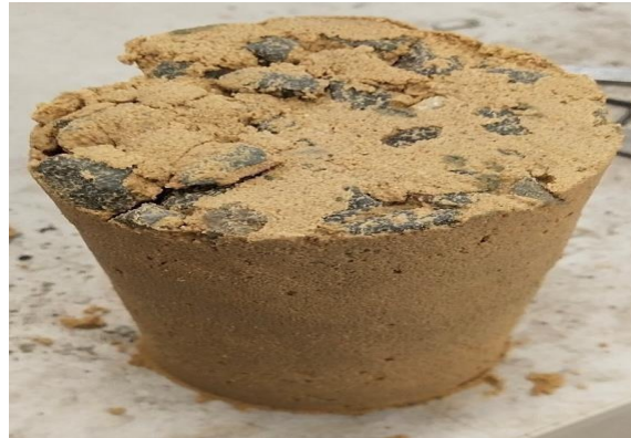
Figure 22 Recycle settled concrete column
