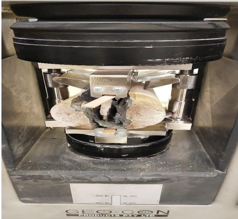
Figure 39. Splitting tensile test
