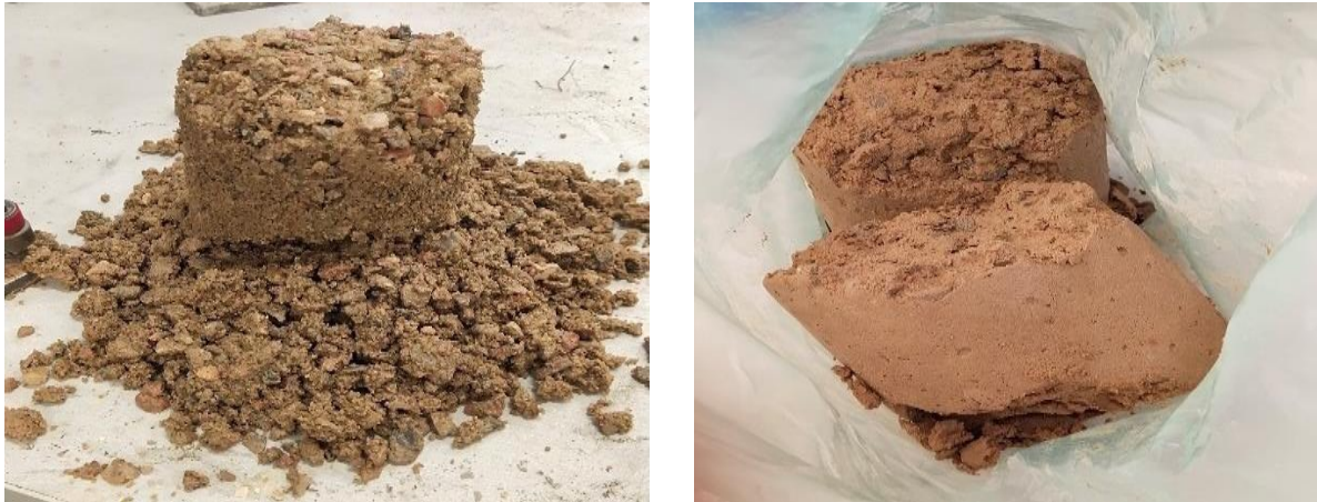
Figure 19. GGBS, Fly Ash and RCA failed concrete
