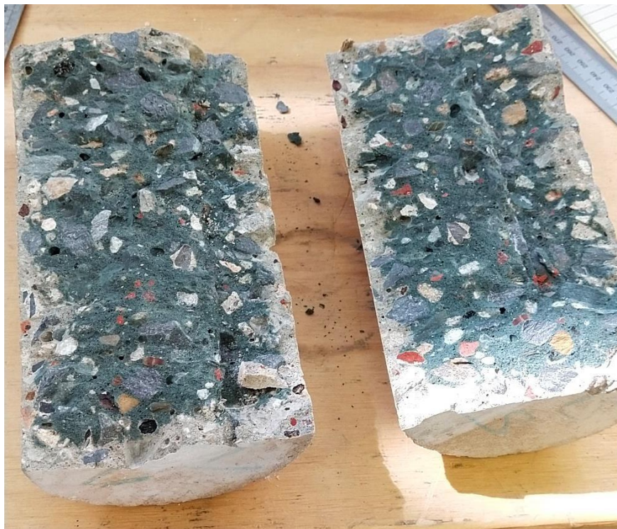
Figure 51 Appendix 6 Broken water material concrete sample
