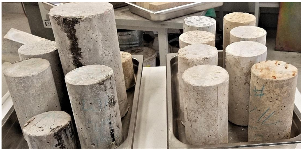
Figure 1. ASR Affected concrete column
