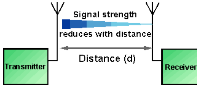
Figure 8. present the relationship between the signal strength and the distance (Poole, I 2016a).
