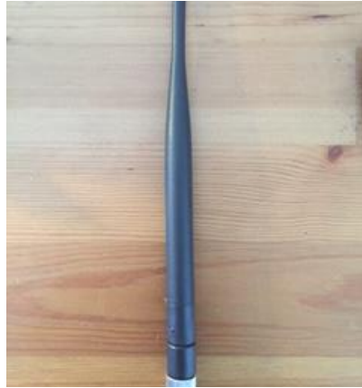
Figure 19. Half Wave Dipole Antenna 900MHz
