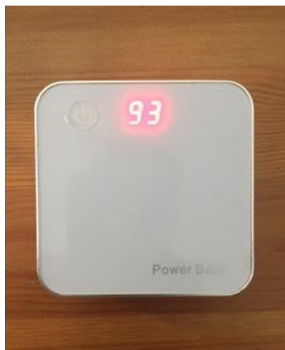
Figure 20. Power bank (battery) output voltage 5V and capacity is 8400mA
