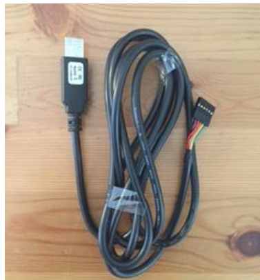
Figure 18. The serial port FTDI cable which is used to link the radio modem and computer or with battery
