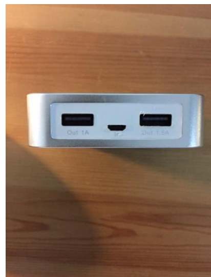
Figure 20. Power bank (battery) output voltage 5V and capacity is 8400mA
