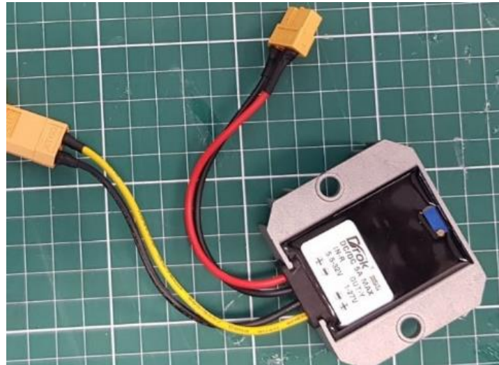
Figure 37: XT60 power port was soldered and covered with heat shrink tubes
