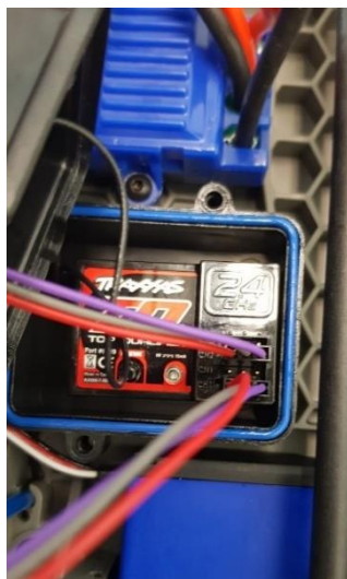
Figure 27: Motor cables are removed and replaced with the D7 and D8 Arduino pins
