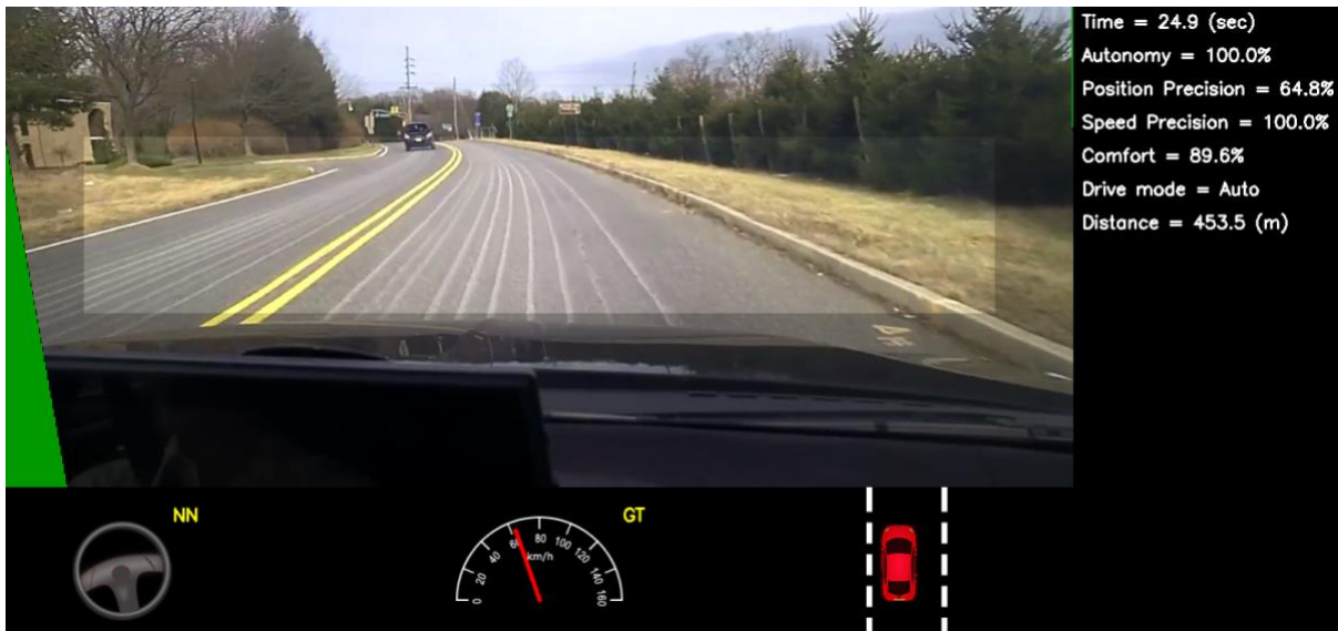
Figure 9: Screen shot of the simulator in interactive mode. The green area on the left is unknown because of the viewpoint transformation. The highlighted, wide rectangle below the horizon is the area which is sent to the CNN.
