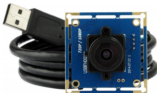
Figure 29: ELP USB 1080 p HD camera with 2.1 mm lens
