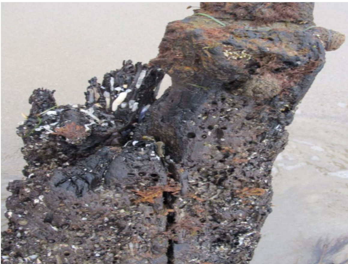
Figure 5.2 Teredo navalis attack on frame timber (photograph by J. Mitchell).
