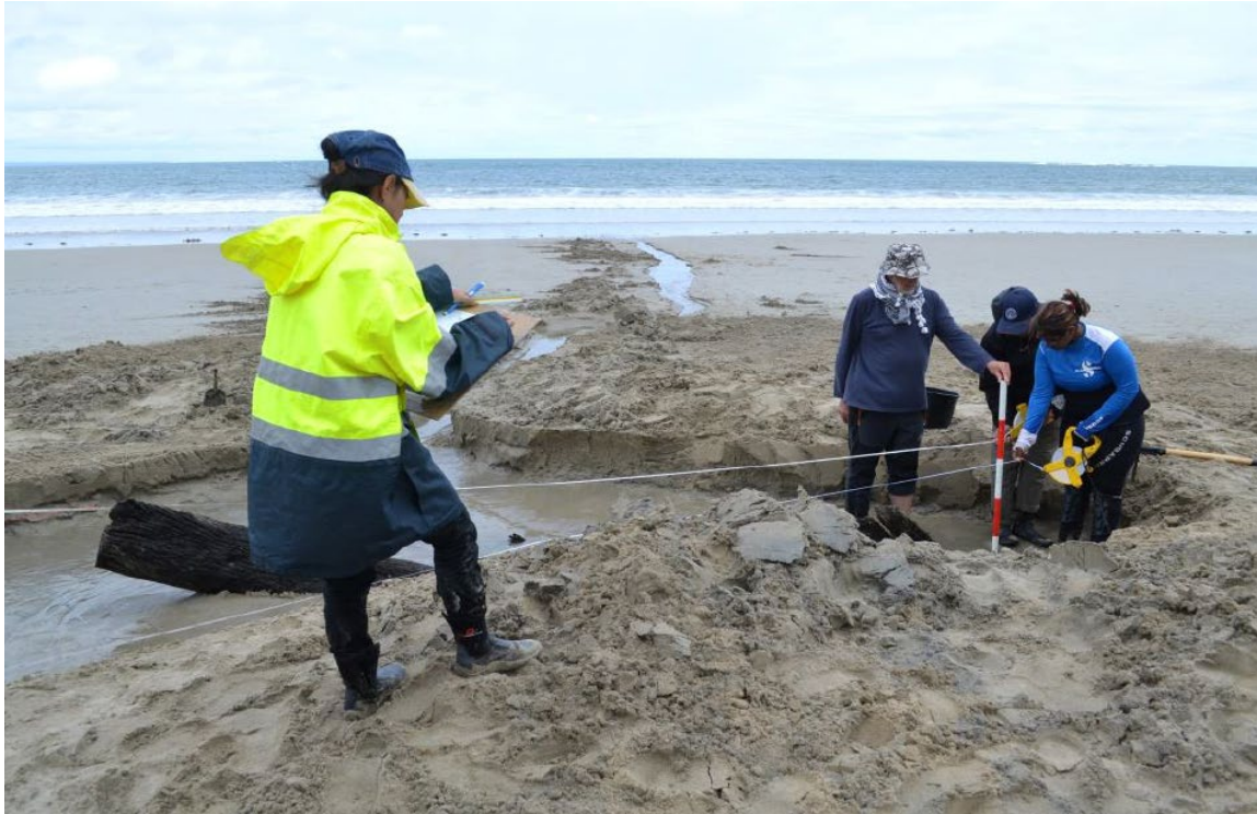
Figure 3.5 Participants measuring Site A using trilateration with C. King illustrating the site (photograph by S. Landicho).
