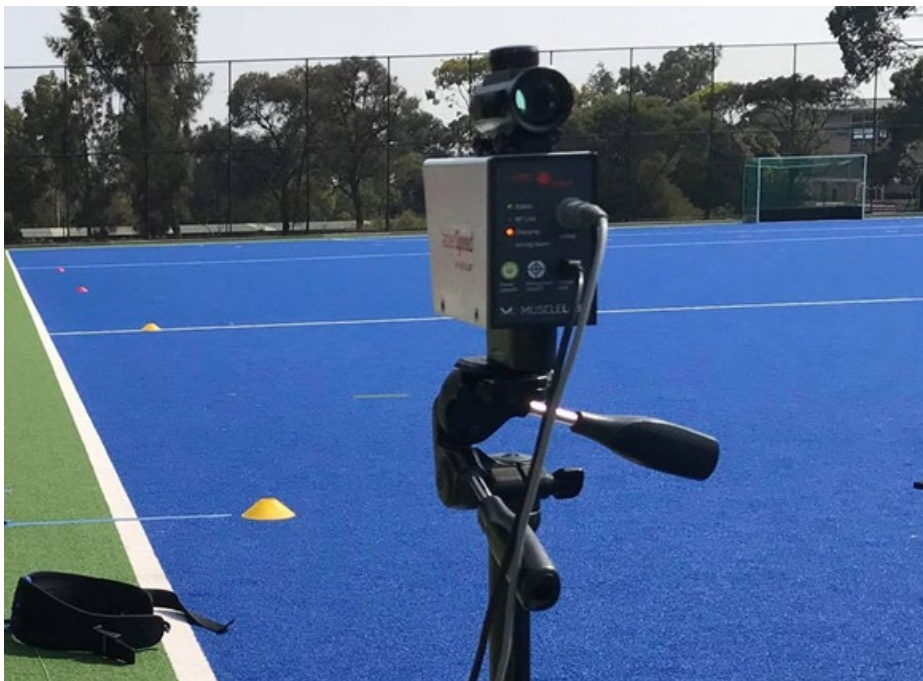
Figure 5.2. MuscleLab™ is a system which uses an optical laser to measure sprint distance over time and automatically calculates sprint mechanical properties.
