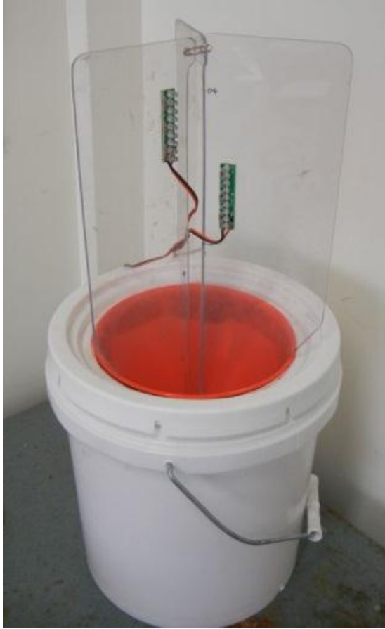
Figure 1: Constructed Light trap showing banks of LEDs and general setup of upright clear vanes positioned over a funnel.
