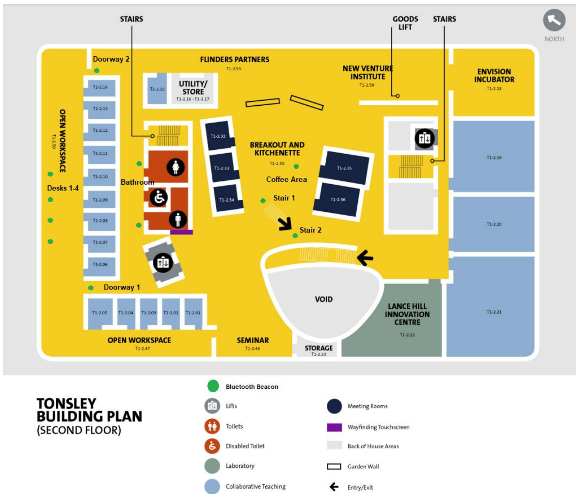
Figure 17: Office building layout with Bluetooth beacons (Flinders University, Tonsley Campus Map with Bluetooth beacon markings, 2019)
