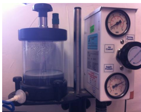
Figure 4 – 4: The low-compliance pneumohydraulic perfusion pump. The reservoir on the left of the image is attached to catheter and manifold for perfusion manometry.
