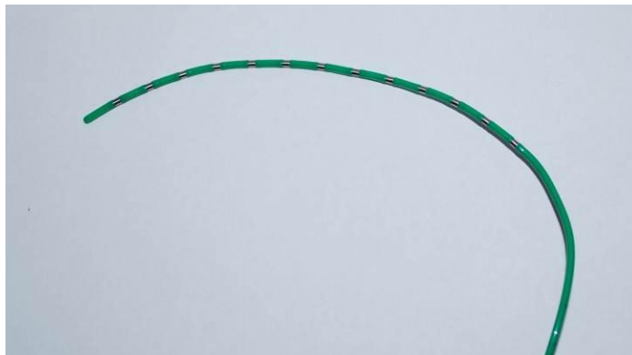
Figure 4-7: Photograph of impedance catheter containing 13 impedance electrodes.
