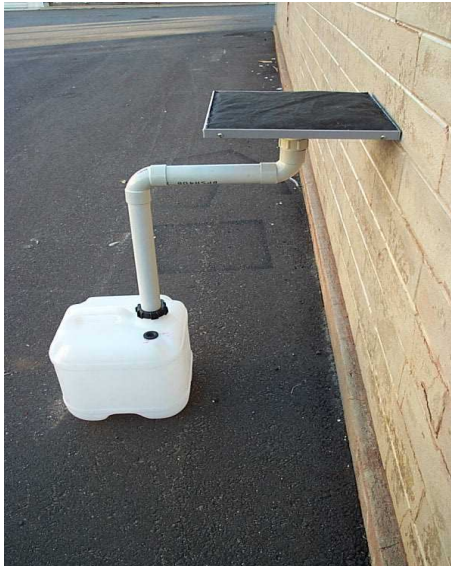
Fig 2.2. Capillary wick lysimeter Figure 2.3 Lysimeter collection plate installation
