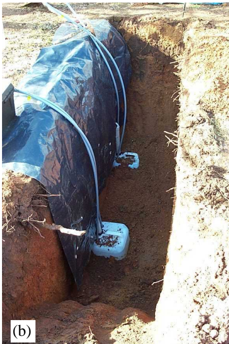
Figure 2.4 Installation of capillary wick lysimeters
