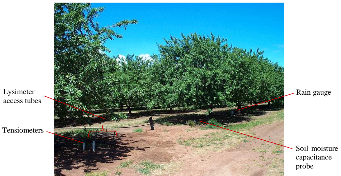
Figure 2.12 Monitoring station 2 at the SR study site. The area of coverage of the micro sprinklers necessitated spreading monitoring equipment between canopies of two trees.
