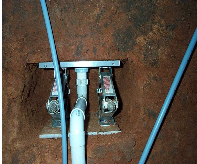
Fig 2.2. Capillary wick lysimeter Figure 2.3 Lysimeter collection plate installation
