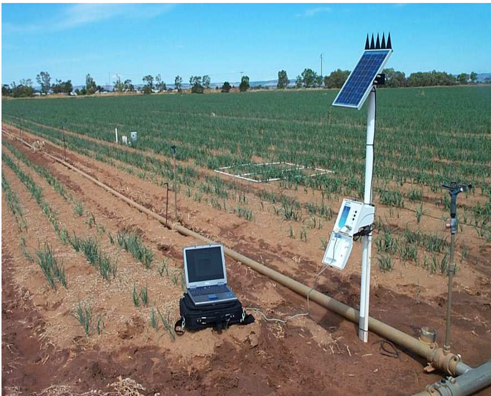
Figure 2.5 Soil moisture probes at study site TR.
