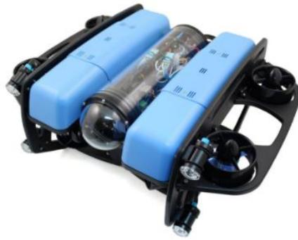
Figure 3.1 The BlueROV2 Heavy Configuration Retrofit Kit (BlueRobotics 2018a)
