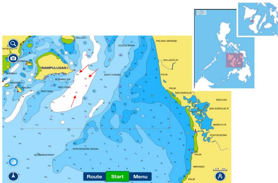
Figure 37 In Navionics 2010 Asia&Africa of the same region as Pontevedra 3551-II, bathymetric values at the same location as the NAMRIA's topographic map in figure 21 are listed as 23.5, 29, and 29 m.
