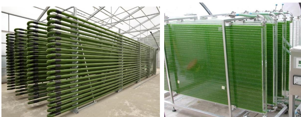
Figure 1.3. Different types of photobioreactors (a) A tubular photobioreactor designated PBR 4000 G IGV Biotech, and (b) plastic plate photobioreactor PBR 500 P IGV Biotech (Alaswad et al., 2015).
