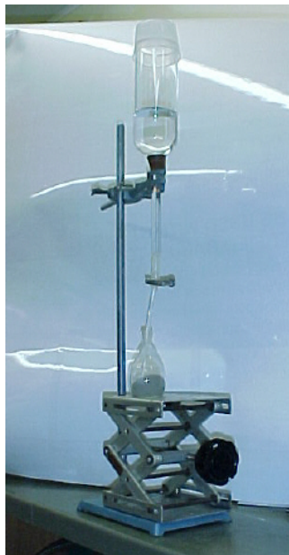
Fig. Appendix 3.2.1 Setup of apparatus for removal of air from soil by capillary action
