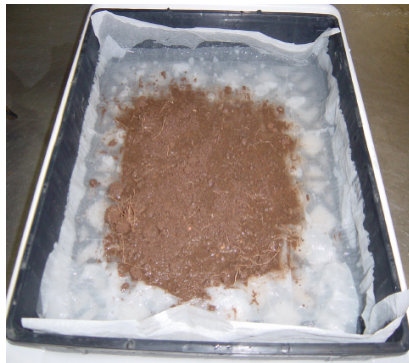
Fig. Append. 10.1 setup of tray with water level immediately below 200g soil.
