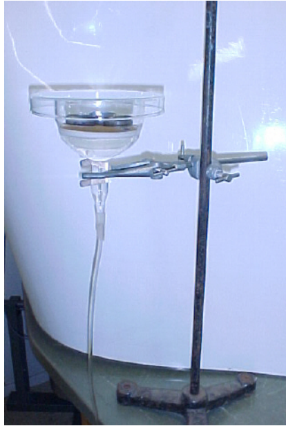
Fig. Appendix 3.1.1 Apparatus for testing field capacity
