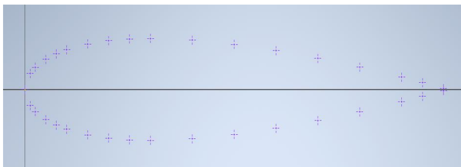
Figure 34 NACA 0018 coordinates plotted in Inventor software.
