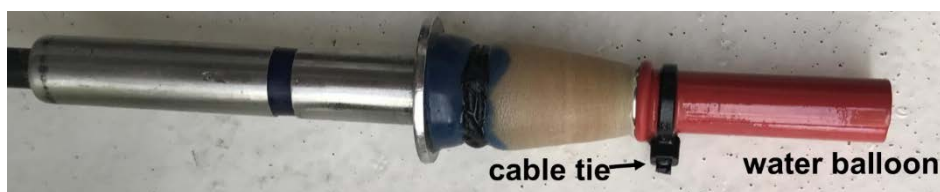
Figure 3.2 - Photograph of the biopsy probe with the surface adaptation including the water balloon (red) covering the biopsy probe tip and secured with a cable tie (98 x 2.5 mm).
