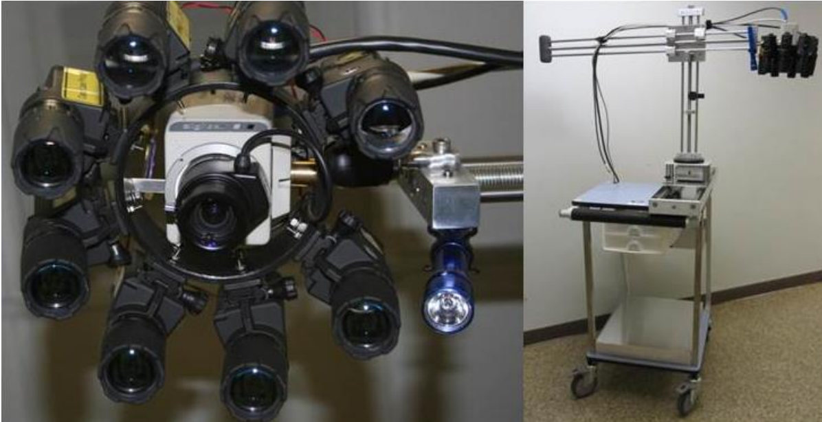
Figure 2-9: Image head with eight laser torches and the imaging system set-up.
