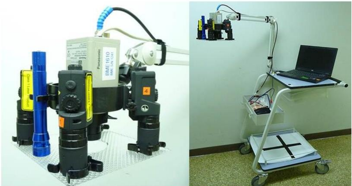
Figure 2-7: Close-up of camera imaging head and the whole imaging system set-up
