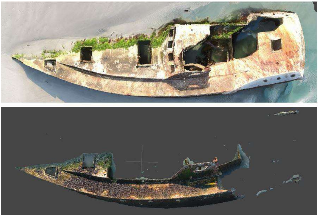
Figure 4.9. 3D photogrammetry comparison of missing main cabin roof and overgrowth of algae (Agisoft Metashape, 2022-07-30)
