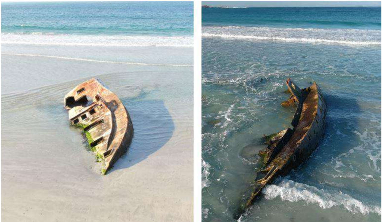
Figure 4.8. Pisces Star 2021 (left) and 2022 (right) deterioration process (2022-06-22)
