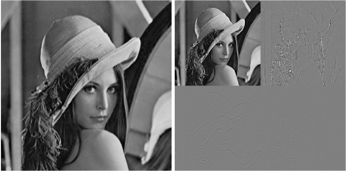
Figure 8.4: Left - Original uncompressed image; Right - One octave wavelet transformed image
