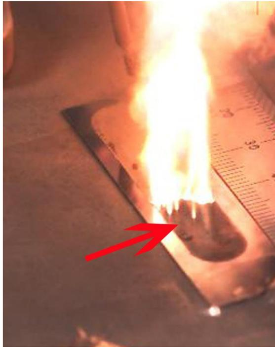
**Figure 3-6: 49.9  $\mu\text{m}$  thick pSi sample, depicting flame break-through ahead of main reaction front.**
