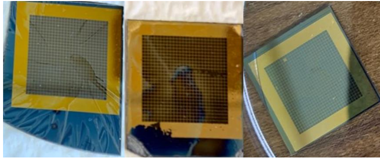
Figure 6-98: CuSCN thin coatings on device substrates demonstrating the macro-scale morphology differences.
