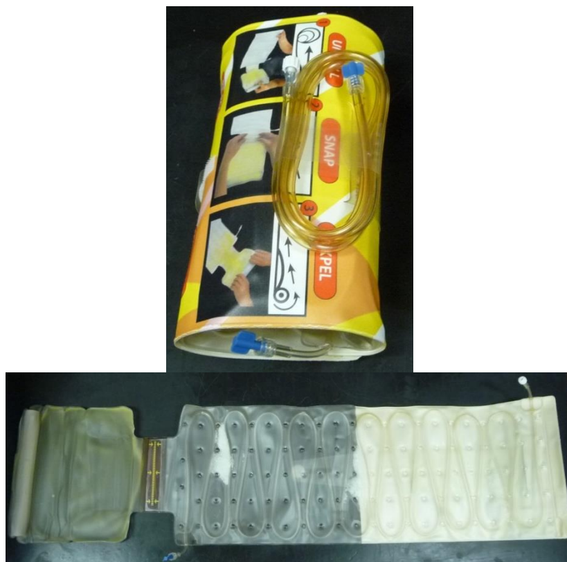
Figure 5.8. An example the clinical trial blood warmer prototype showing it rolled during storage and unrolled for clinical use.
