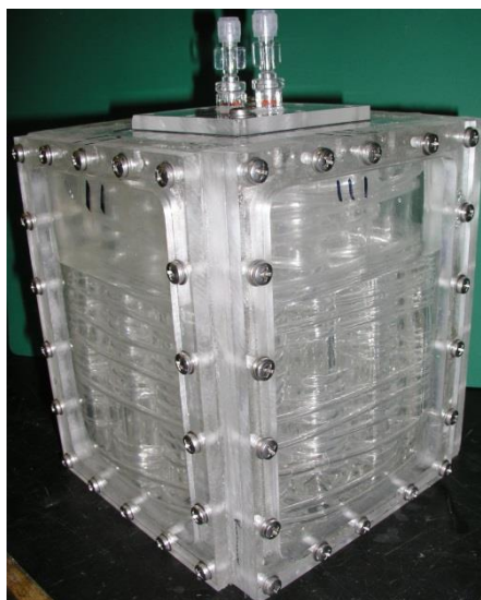
Figure 5.5.1. Initial prototype blood warmer incorporating a rigid design
