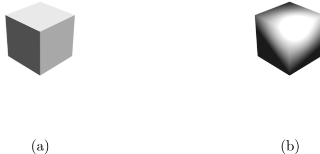
Figure 2.4: A Phong shaded cube: (a) normal vectors perpendicular to the faces (b) normals coincident with the cube centre
