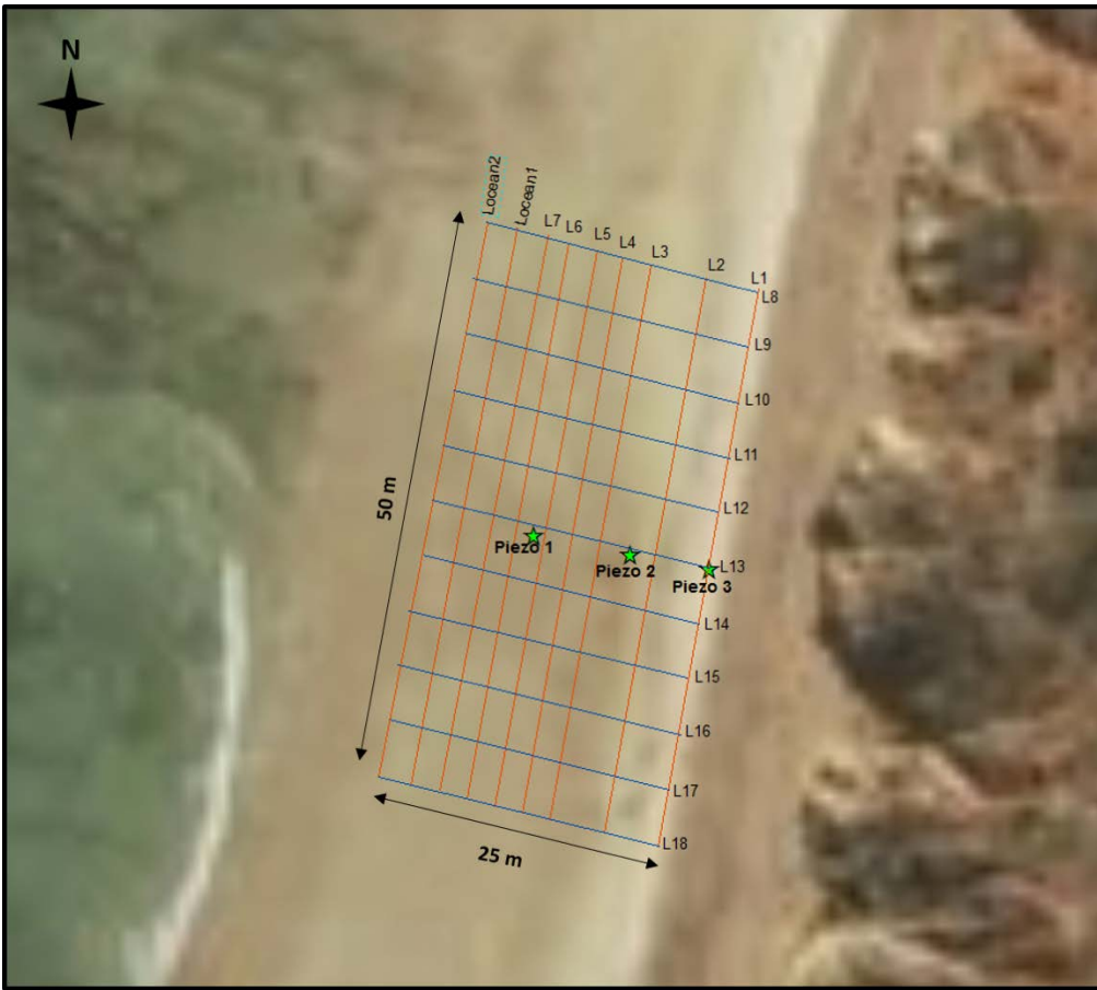
Figure 10 Schematic representation of the geophysical survey transect array at Sellicks Beach. The image shows the 11 x 50 m N-S transect lines (orange lines), the 9 x 25 m E-W transect lines (blue lines) and the three piezometers (green stars).
