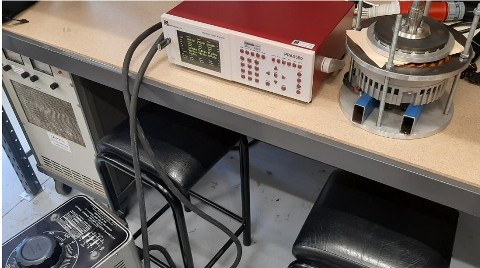
Fig. 8.18. The experimental setup, consisting of autotransformer, power analyser, and the AFIM, for carrying out the locked rotor test at 50Hz.
