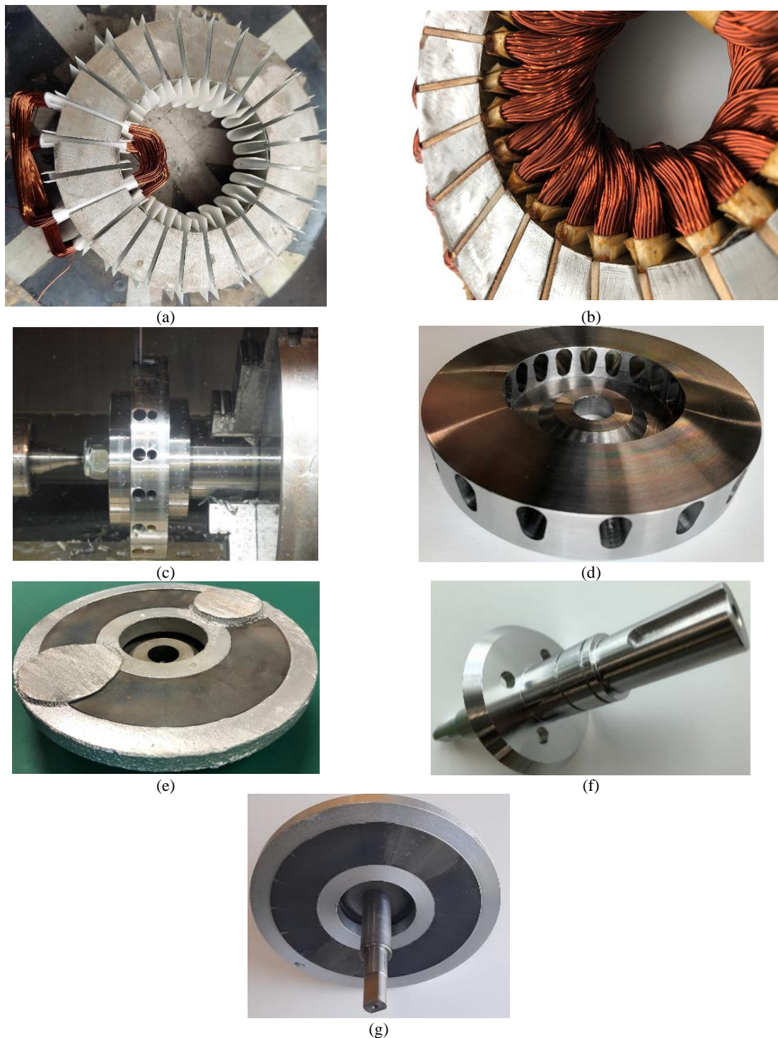
Fig. 8.7. The fabricated parts of the designed AFIM. (a) stator with the insulator layers prepared for winding. (b) wound stator. (c) the initial step for the rotor slots milling. (d) rotor iron. (e) the die-casted cage on rotor (the aluminium circles on the rotor are the inlet and outlets of the casting process). (f) shaft. (g) the assembled shaft on rotor.
