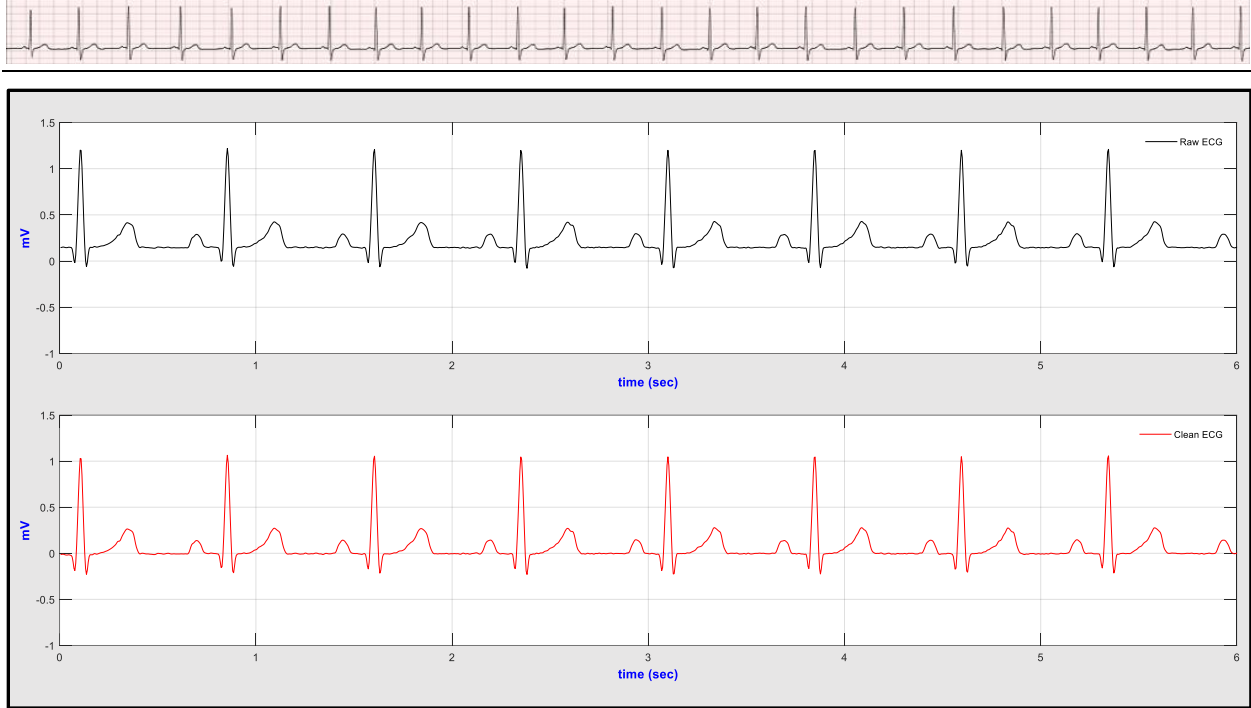
Figure 5.8: ECG from 1mV input signal; black – raw ECG; red – after the baseline wander was removed by a 2 nd order zero-phase shift MATLAB based Butterworth high pass filter.
