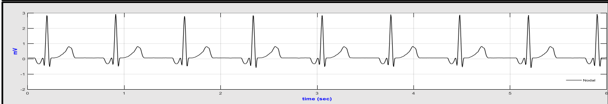
c) Nodal in lead II ECG; top - captured by the reference Resting ECG, 25mm/s, 10mm/mv, R_{peak} = \sim 2.8mV ; bottom - captured by the proposed ECG hardware
