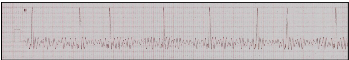
a) Atrial flutter in lead-II ECG; top - captured by the reference Resting ECG, 25mm/s, 10mm/mv, R_{peak} = \sim 2.8mV ; bottom - captured by the proposed ECG hardware
