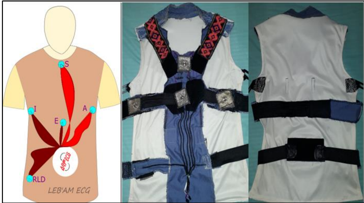
Figure 4.16: The first ECG vest (left – proposed model; middle – anterior view and right – posterior view)
