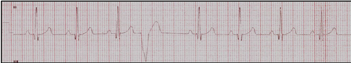
a) Premature atrial contraction in lead-II ECG; top - captured by the reference Resting ECG, 25mm/s, 10mm/mv, R_{peak} = \sim 2.8\text{mV} ; bottom - captured by the proposed ECG hardware
