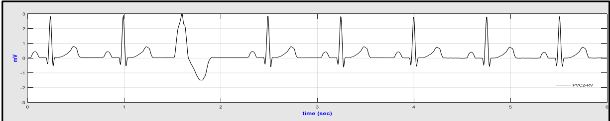
c) Premature ventricular contraction (PVC2-RV) in lead-II ECG; top - captured by the reference Resting ECG, 25mm/s, 10mm/mv, R_{peak} = \sim 2.8\text{mV} ; bottom - captured by the proposed ECG hardware
