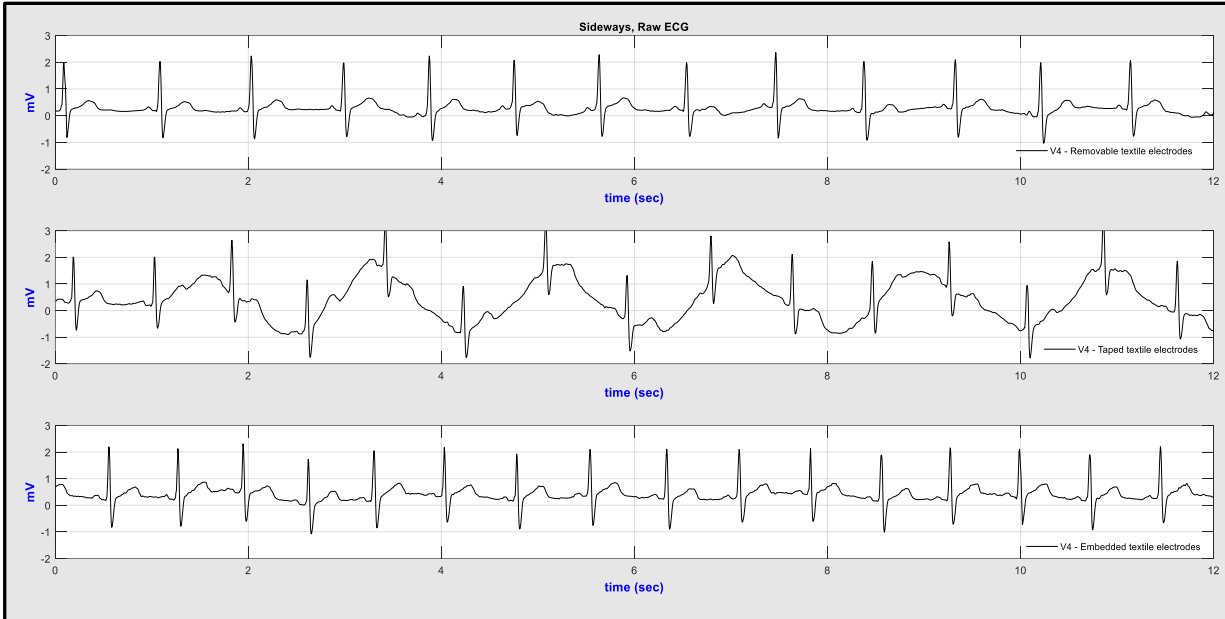
a) Sideways ECG (top – removable; middle – taped and bottom – embedded electrodes)
