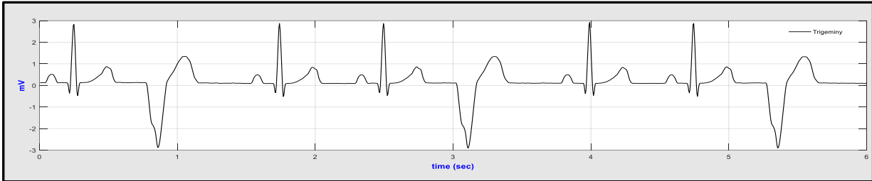
b) Trigeminy in lead-II ECG; top - captured by the reference Resting ECG, 25mm/s, 10mm/mv, R_{peak} = \sim 2.8mV ; bottom - captured by the proposed ECG hardware
