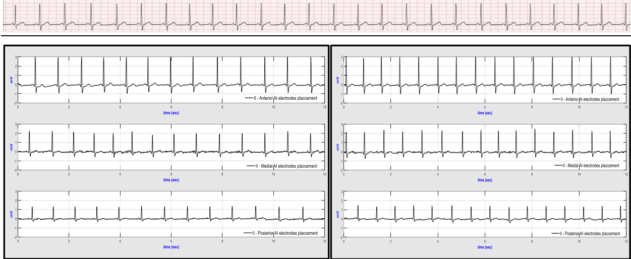
Figure 6.8: Comparison of lead-II ECGs acquired during sideways movement (left) and climbing stairs (right) based on different AI electrodes placements (top – anterior, middle – medial and bottom – posterior electrode placement)
