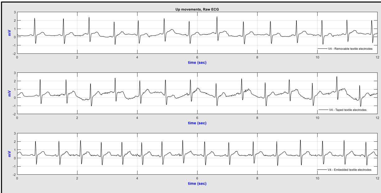
b) Up movements ECG (top – removable; middle – taped and bottom – embedded electrodes)
