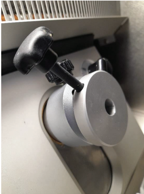
FIGURE 20: ANGLED PLATFORM FOR OBLIQUE CUTTING.
