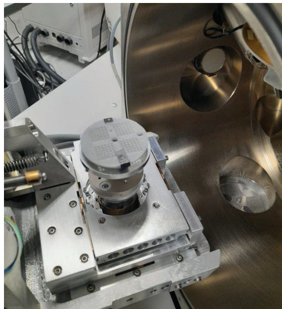
FIGURE 9: SAMPLE HOLDER PLACED INSIDE CHAMBER BEFORE IMAGING.
