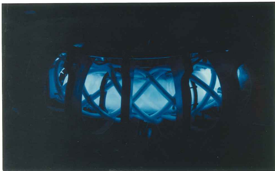
Frontispiece Photograph of a typical \langle \tilde{j} \times \tilde{b} \rangle RF current drive discharge recorded in the dark. The discharge was produced in Argon gas using the Rythmac-2 conventional toroidal device equipped with the helical mesh antenna.
