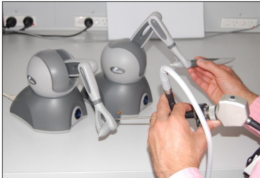
Figure 48: An endoscope connected to a 3DOF haptic device at its tip delivers reactive torques to the user's hand
